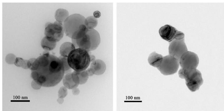
**Figure S6.** The TEM picture of FeNP (left) and CuNP (right).
