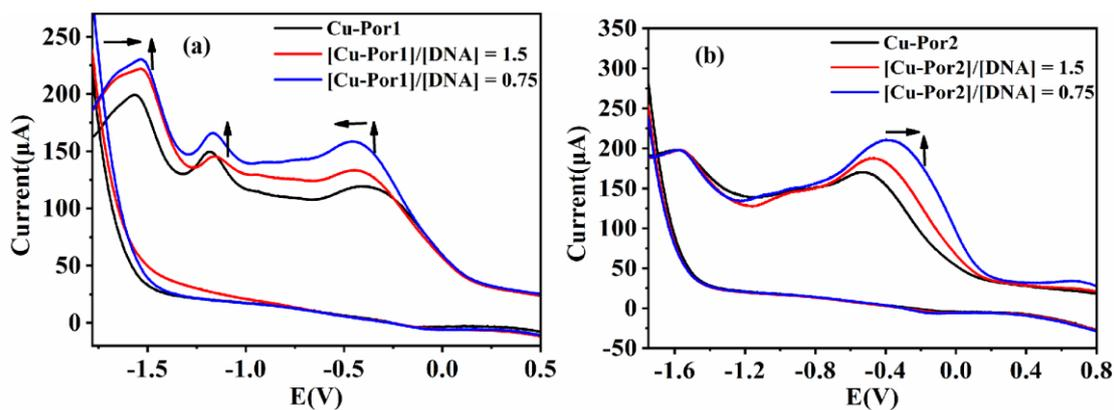
**Fig. S6** Cyclic voltammogram of (a) Cu-Por1 ( $2 \times 10^{-4}$  M), (b) Cu-Por2 ( $2 \times 10^{-4}$  M) in the absence and presence of ct-DNA in 50 mM NaCl, 5 mM Tris, pH 7.2. [complex] / [DNA] = 0, 1.5, 0.75, scan rate, 100 mVs<sup>-1</sup>.
