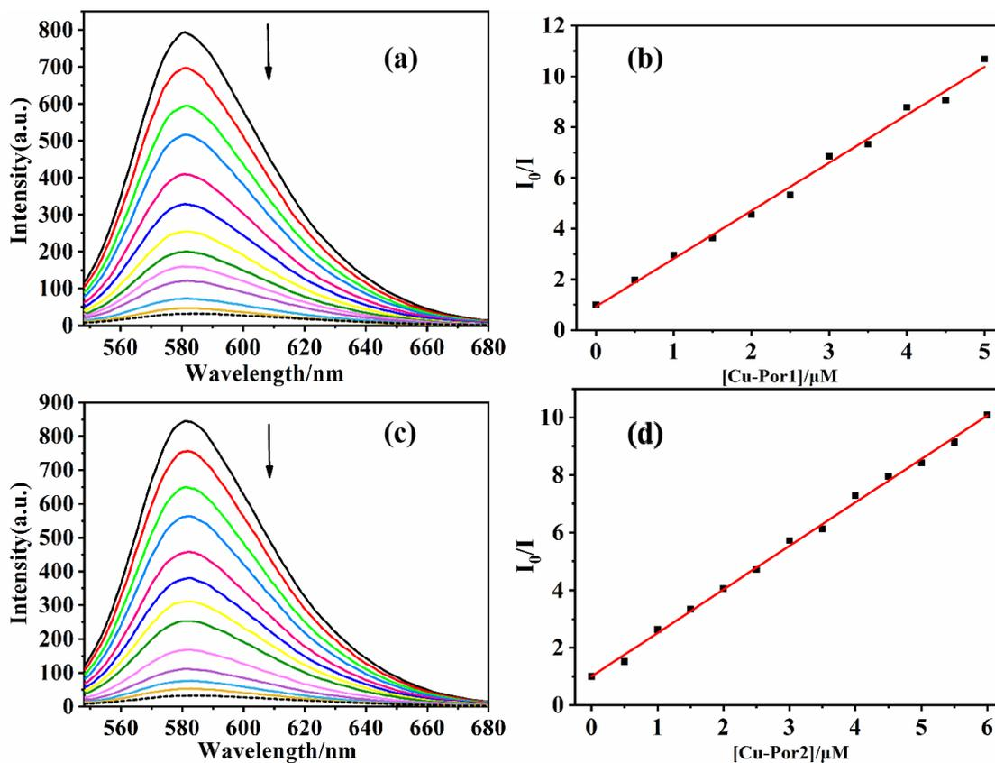
**Fig. S5** Emission spectra of EtBr (black dotted line), EtBr bound to the ct-DNA (black solid line), and in the presence (other colored lines) of Cu-Por1 (a), Cu-Por2 (c) with increasing amounts 0-20 μM. [EtBr] = 5 μM, [DNA] = 1 mM. Arrow indicates changes in the emission intensity upon addition of the Porphyrins concentration; Stern-Volmer plots of the EtBr-DNA fluorescence titration for complexes Cu-Por1 (b) and Cu-Por2 (d).
