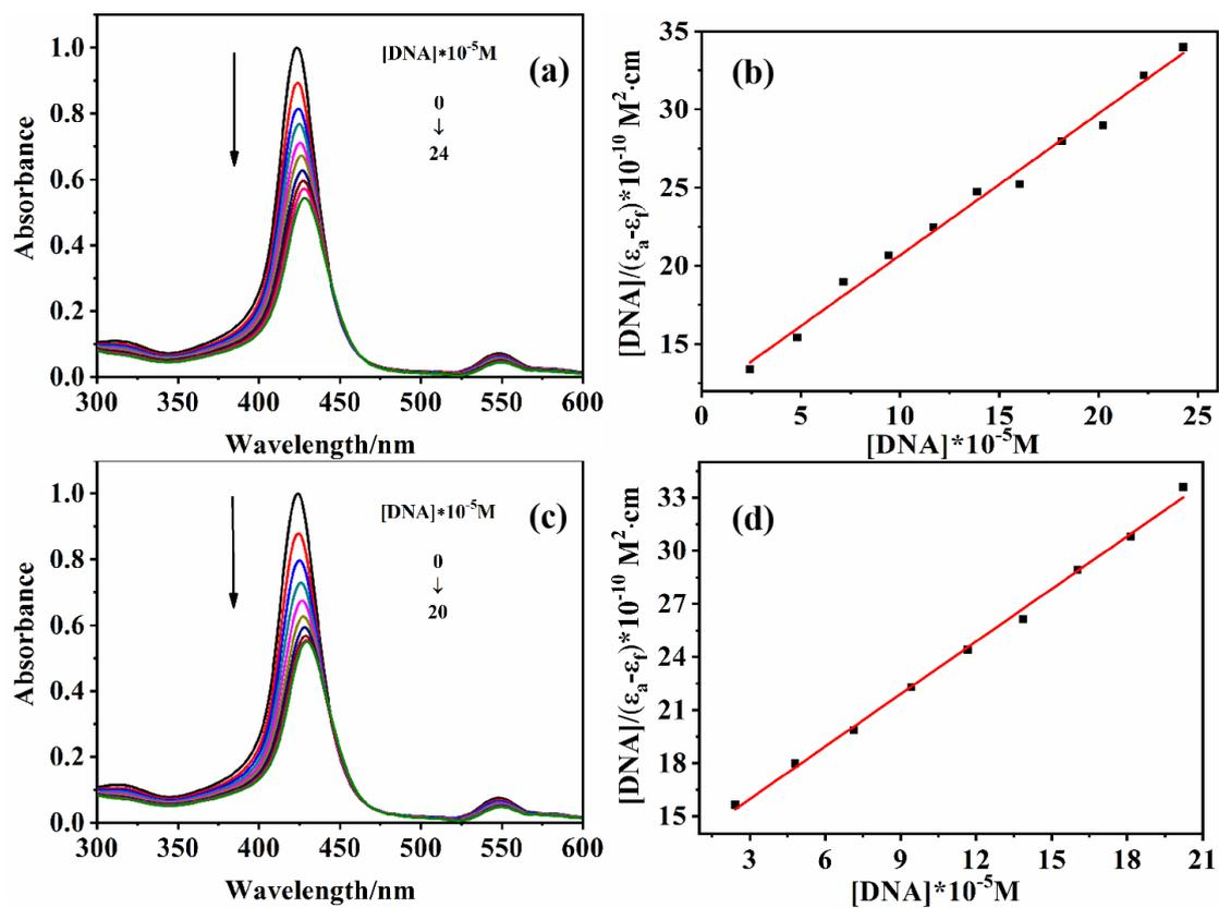
**Fig. S4** Normalized absorption spectra of Cu-Por1 (a), Cu-Por2 (c) in buffer at 25°C in the presence of increasing amounts of ct- DNA. [Cu-Porx] = 10  $\mu\text{M}$ . Black arrow indicate the change in absorbance upon increasing the DNA concentration; Plot of [DNA] vs  $[DNA]/(\epsilon_a - \epsilon_f)$  of Cu-Por1 (b), Cu-Por2 (d).
