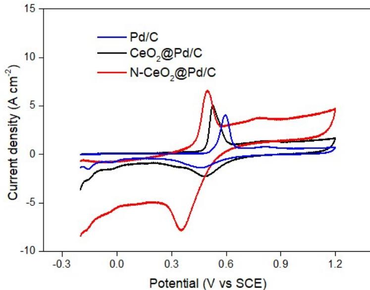
**Fig. S11** CO stripping measurements recorded in N<sub>2</sub>-saturated solution of 0.1 M H<sub>2</sub>SO<sub>4</sub> electrolyte at scan rate of 50 mV s<sup>-1</sup> and 25 °C for Pd/C, CeO<sub>2</sub>@Pd/C and N-CeO<sub>2</sub>@Pd/C catalysts.
