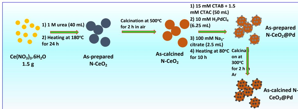
**Fig. S1** Hydrothermal synthesis of N-CeO<sub>2</sub>@Pd catalyst.
