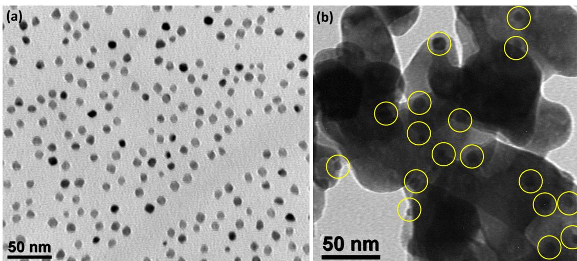
Fig. S7 HRTEM image of (a) the synthesized Pd and (b) Pd/C (~20 wt.% Pd) nanocatalyst.
