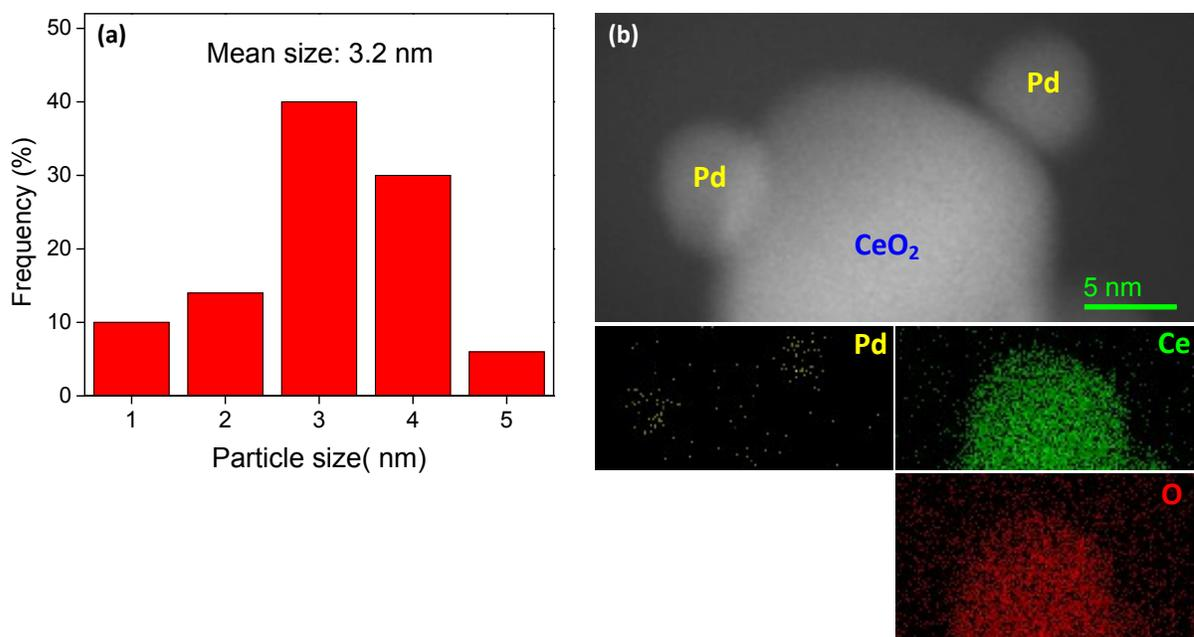
**Fig. S4** (a) Particle size distribution of Pd loaded on N-CeO<sub>2</sub> and (b) HRTEM mapping elements of N-CeO<sub>2</sub>@Pd nanocatalyst.
