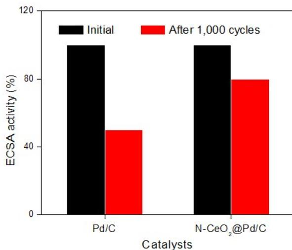
**Fig. S12** ECSA stability tests for Pd/C and N-CeO<sub>2</sub>@Pd/C catalysts in the N<sub>2</sub>-saturated solution of 0.1 M H<sub>2</sub>SO<sub>4</sub> at a sweep rate of 50 mV s<sup>-1</sup> at room temperature.
