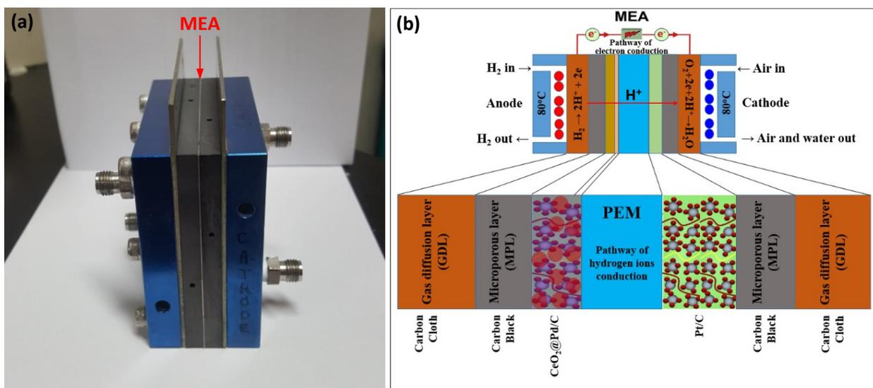
**Fig. S3** (a) Prepared device for single cell test and (b) device simulation for layer-by-layer.
