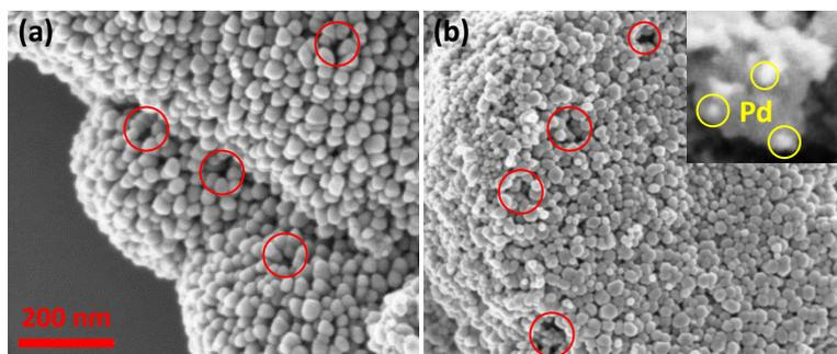
Fig. S5 FEM analysis of (a) N-CeO<sub>2</sub> and (b) N-CeO<sub>2</sub>@Pd nanocatalyst.
