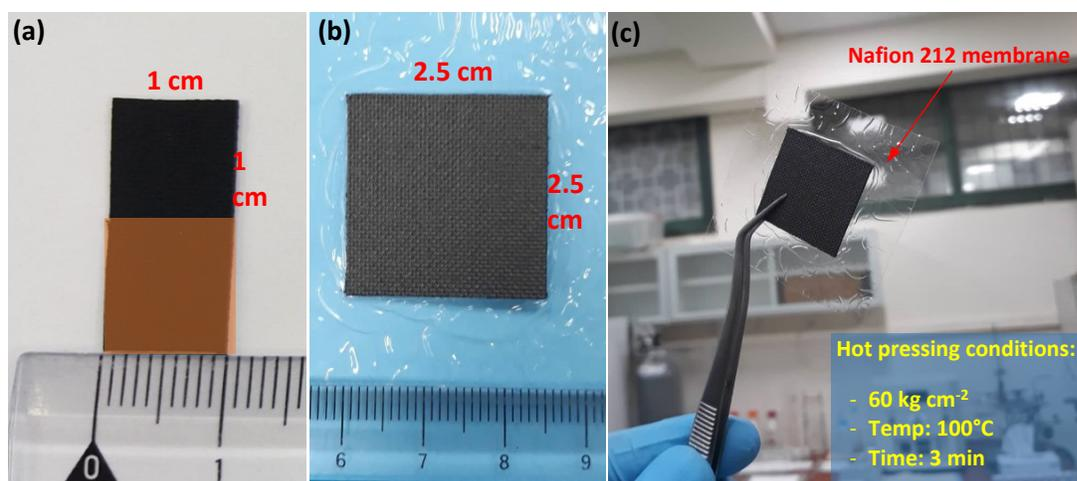
**Fig. S2** Working area of electrodes for (a) CV and (b) single cell tests. (c) Prepared MEA consisting N-CeO<sub>2</sub>@Pd/C as anode and Pt/C as cathode.
