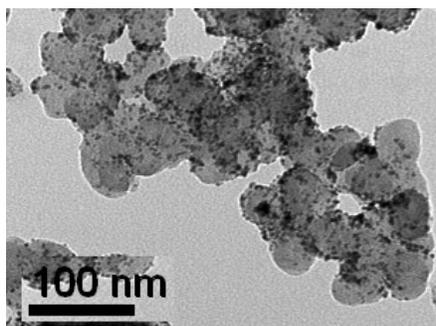
Fig. S8 HRTEM image of Pt/C (~20 wt.% Pt) nanocatalyst.
