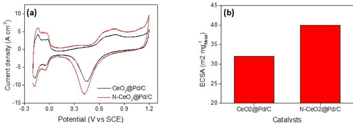
**Fig. S10** (a) CV curves of hydrogen oxidation reaction and (b) ECSA results in the N<sub>2</sub>-saturated solution of 0.1 M H<sub>2</sub>SO<sub>4</sub> for CeO<sub>2</sub>@Pd/C and N-CeO<sub>2</sub>@Pd/C electrodes.
