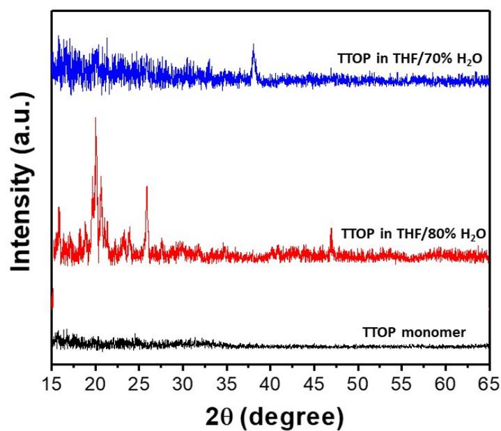
**Figure S2.** XRD patterns of the monomeric TTOP molecules (black line) and TTOP aggregates in the THF/H<sub>2</sub>O mixtures with the water fraction of 70% (blue line) and 80% (red line).
