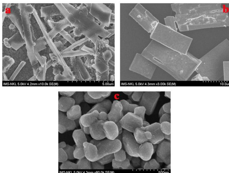
**Figure S1.** SEM images of TTOP aggregates after catalysis; aggregates prepared from H<sub>2</sub>O/HF mixture with water fraction of 70% (a), 80% (b), and 90% (c).
