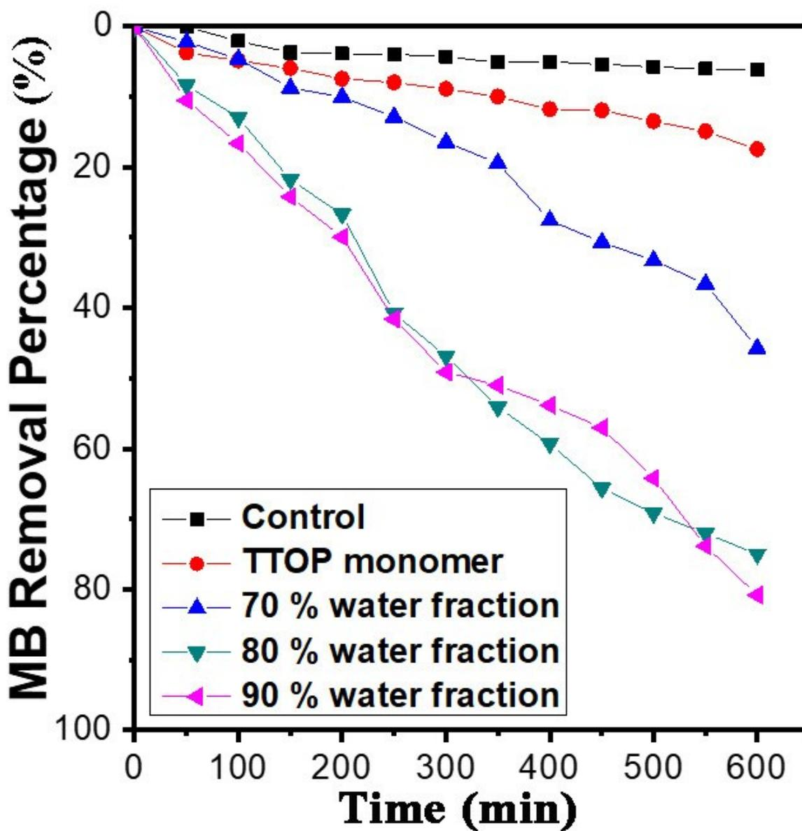
Figure S3. Photocatalytic behaviour of TTOP porphyrin aggregates toward Methylene blue dye
