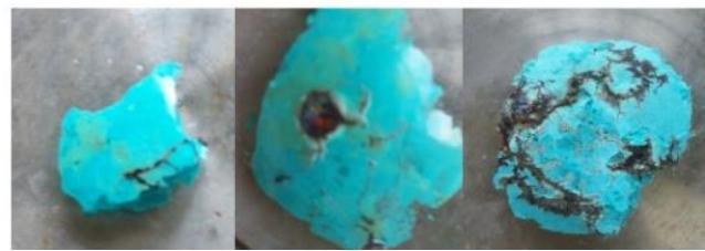
**Figure S1** Non-ignited the precursor of  $\phi = 1.5$  with physically adsorbed water of 1.4%.
