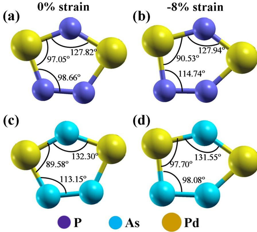
**Figure S2:** The electronic structure of pentagonal PdP<sub>2</sub> and PdAs<sub>2</sub> at 0% and 8% compressive strain.
