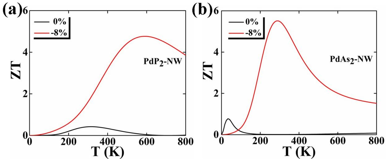
**Figure S9:** Calculated figure of merit (ZT) of both strained and unstrained ( $\epsilon = 0\%$  and  $-8\%$ ) for (a) PdP<sub>2</sub>-NW and (b) PdAs<sub>2</sub>-NW as a function of temperature is shown for larger lead. Both lead and scattering region are of the same material. The left and right lead consists of three primitive unit cells. The scattering region is consisting of three primitive cells.
