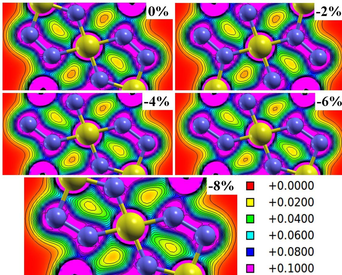
**Figure S11:** The charge contour plot of PdP<sub>2</sub>-NW with applied strain.
