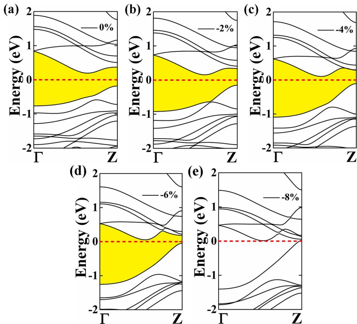
**Figure S4:** The electronic band structure of penta PdP<sub>2</sub>-NW with applied strain. The Fermi level is set at 0K.
