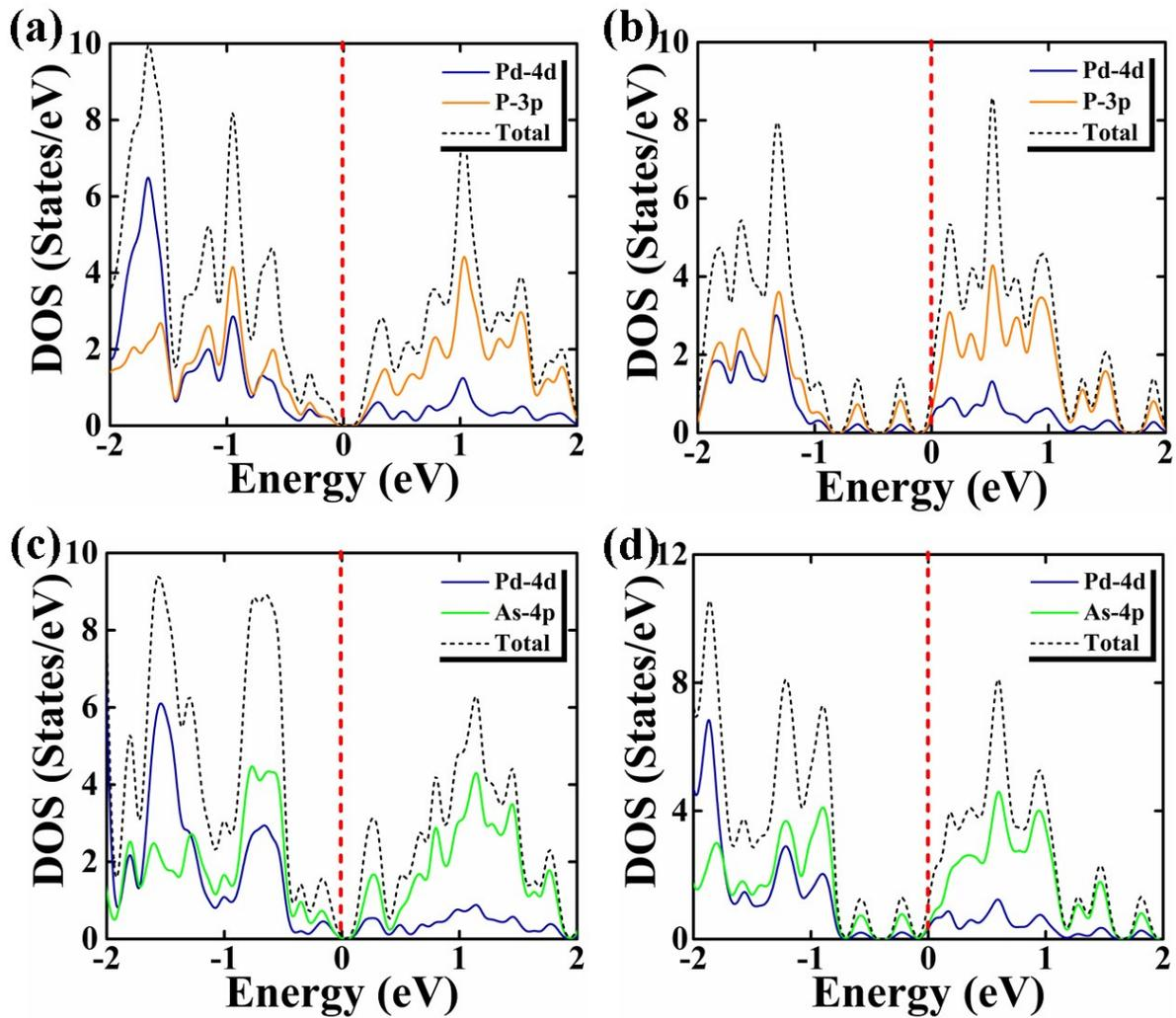
**Figure S3:** The calculated total density of states (TDOS) and partial density of states (PDOS) graph of unstrained ( $\epsilon=0\%$ ) (a) PdP<sub>2</sub>-NW and (c) PdAs<sub>2</sub>-NW is shown. Correspondingly, strained ( $\epsilon=-8\%$ ) PDOS of (b) PdP<sub>2</sub> and (d) PdAs<sub>2</sub> is also shown.
