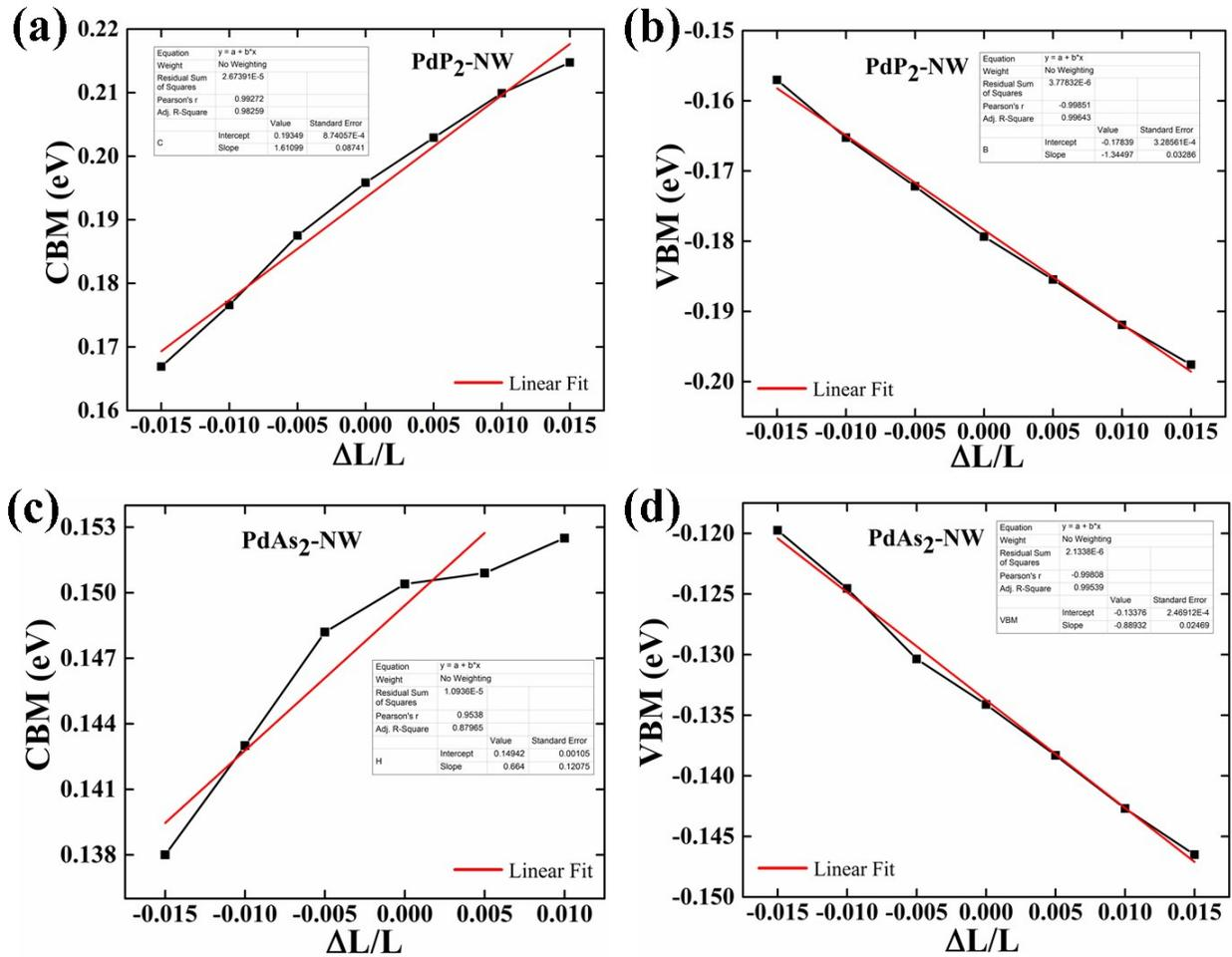
**Figure S7:** The graph for deformation potential of (a) electrons and (b) holes of PdP<sub>2</sub>-NW and (c) electrons and (d) holes of PdAs<sub>2</sub>-NW
