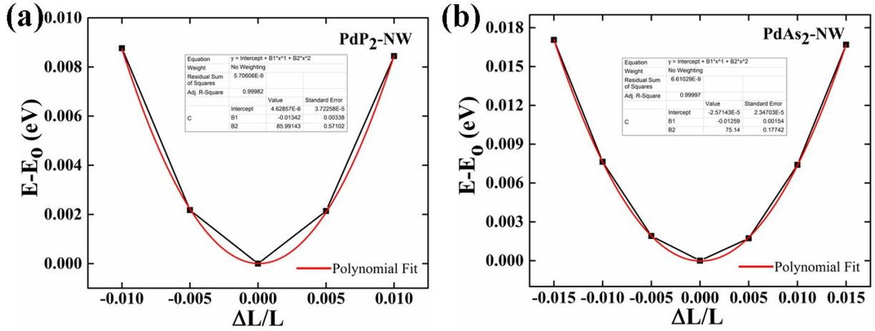
**Figure S6:** The graph for stiffness constant of (a) PdP<sub>2</sub>-NW and (b) PdAs<sub>2</sub>-NW
