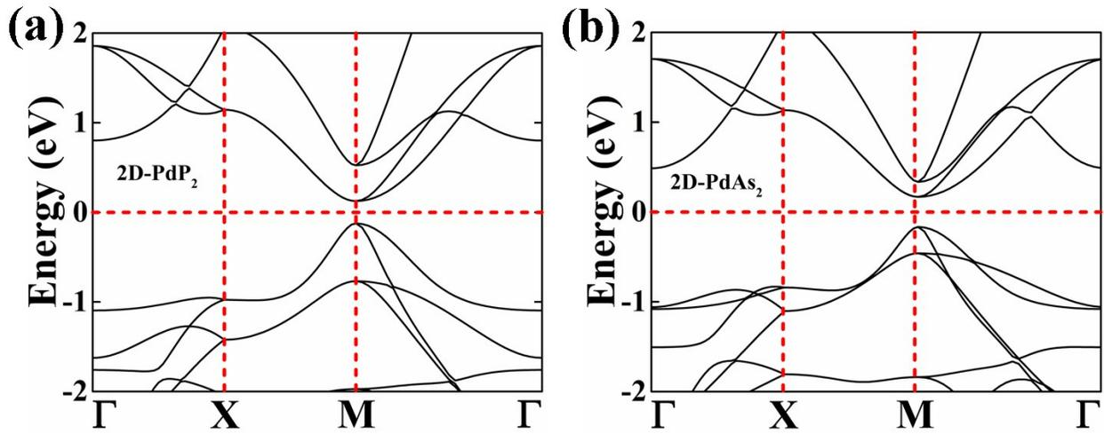
**Figure S1:** The electronic band structure of penta PdP<sub>2</sub> and PdAs<sub>2</sub> monolayer. The Fermi level is set at 0K.
