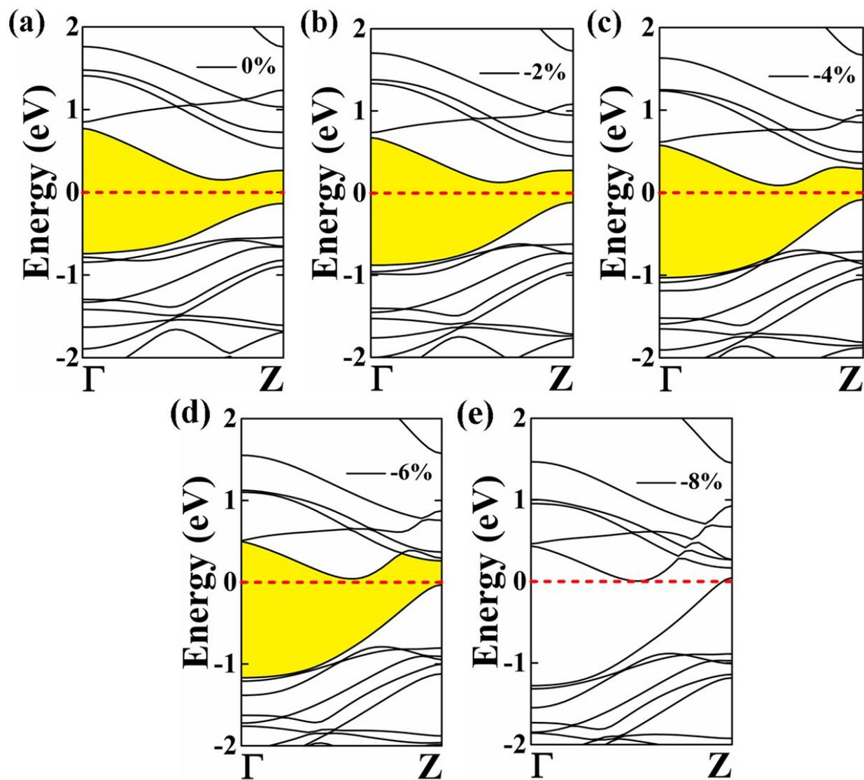
**Figure S5:** The electronic band structure of penta PdAs<sub>2</sub>-NW with applied strain. The Fermi level is set at 0K.
