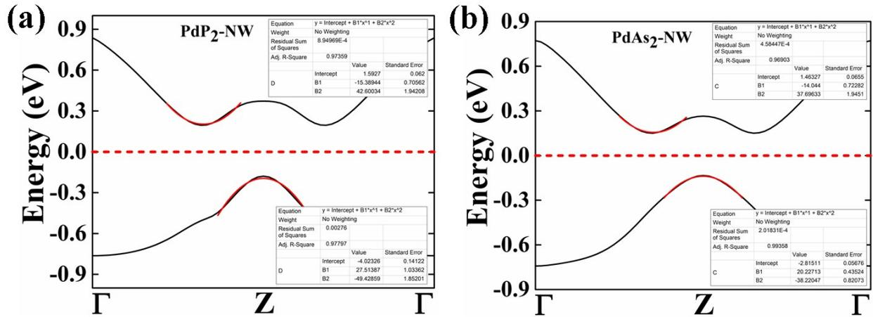
**Figure S8:** The graph for effective mass calculation of (a) PdP<sub>2</sub>-NW and (b) PdAs<sub>2</sub>-NW
