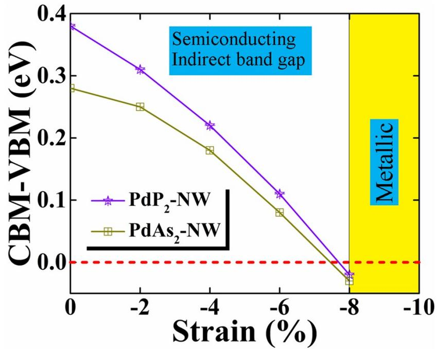
**Figure S10:** The variation of band gap with applied compressive strain for penta PdP<sub>2</sub> and PdAs<sub>2</sub>-NW.
