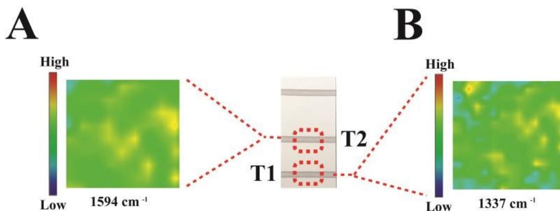
**Fig. S1** (A) SERS mapping of 4-MBA measured at  $1594 \text{ cm}^{-1}$  of T2 line on the SERS-ICA strip. (B) SERS mapping of DTNB measured at  $1337 \text{ cm}^{-1}$  of T1 line on the SERS-ICA strip.
