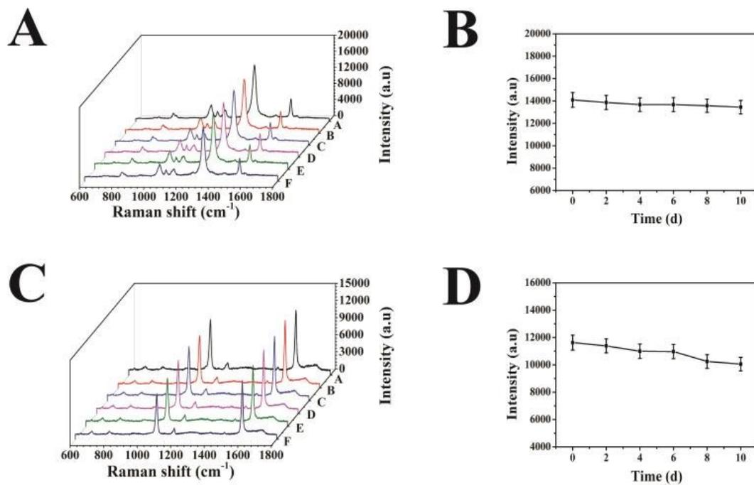
**Fig. S2** Stability of the SERS-ICA strip. (A) SERS spectra on T1 line of SERS-ICA strips. (B) Corresponding scattergram of the peak intensity at 1337 cm<sup>-1</sup>. (C) SERS spectra on T2 line of SERS-ICA strips. (D) Corresponding scattergram of the peak intensity at 1594 cm<sup>-1</sup>.
