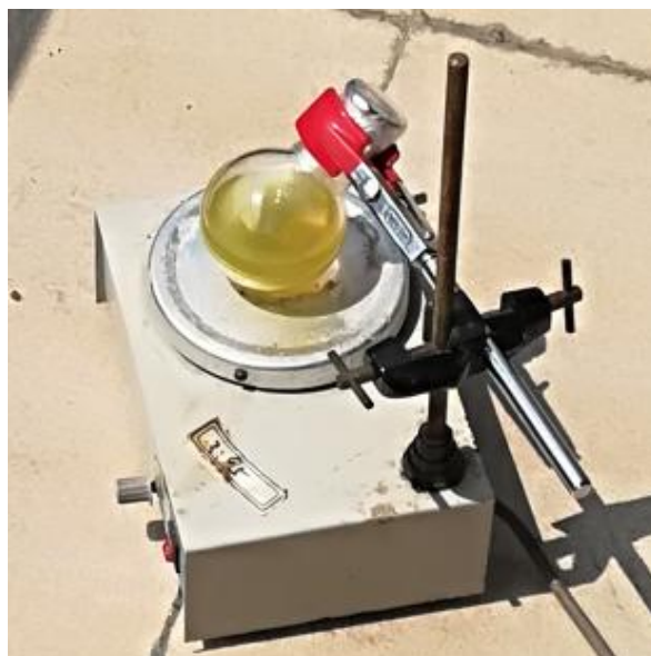
Fig.S1 Outdoor equipment of sunlight-driven water splitting by \text{NiO}_x/\text{Cu}_2\text{O}/\text{CdS} composite.
