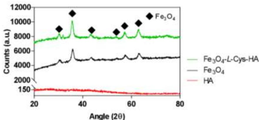
**Figure S3:** DRX diffractograms of bare Fe<sub>3</sub>O<sub>4</sub> nanoparticles, HA and Fe<sub>3</sub>O<sub>4</sub>-*L*-Cys-HA HMNP.
