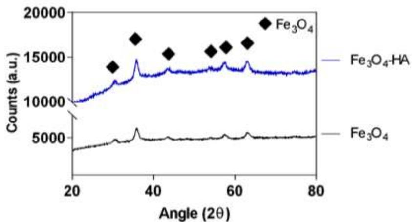
**Figure S5:** DRX diffractograms of bare Fe<sub>3</sub>O<sub>4</sub> nanoparticles, HA and Fe<sub>3</sub>O<sub>4</sub>-HA HMNP.
