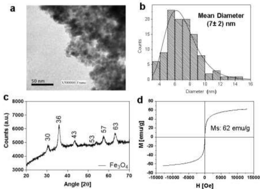
**Figure S1.** Characterization of  $\text{Fe}_3\text{O}_4$  nanoparticles obtained by co-precipitation reaction by: a) TEM image, b) particle size distribution, c) PXRD, and d) VMS analysis.
