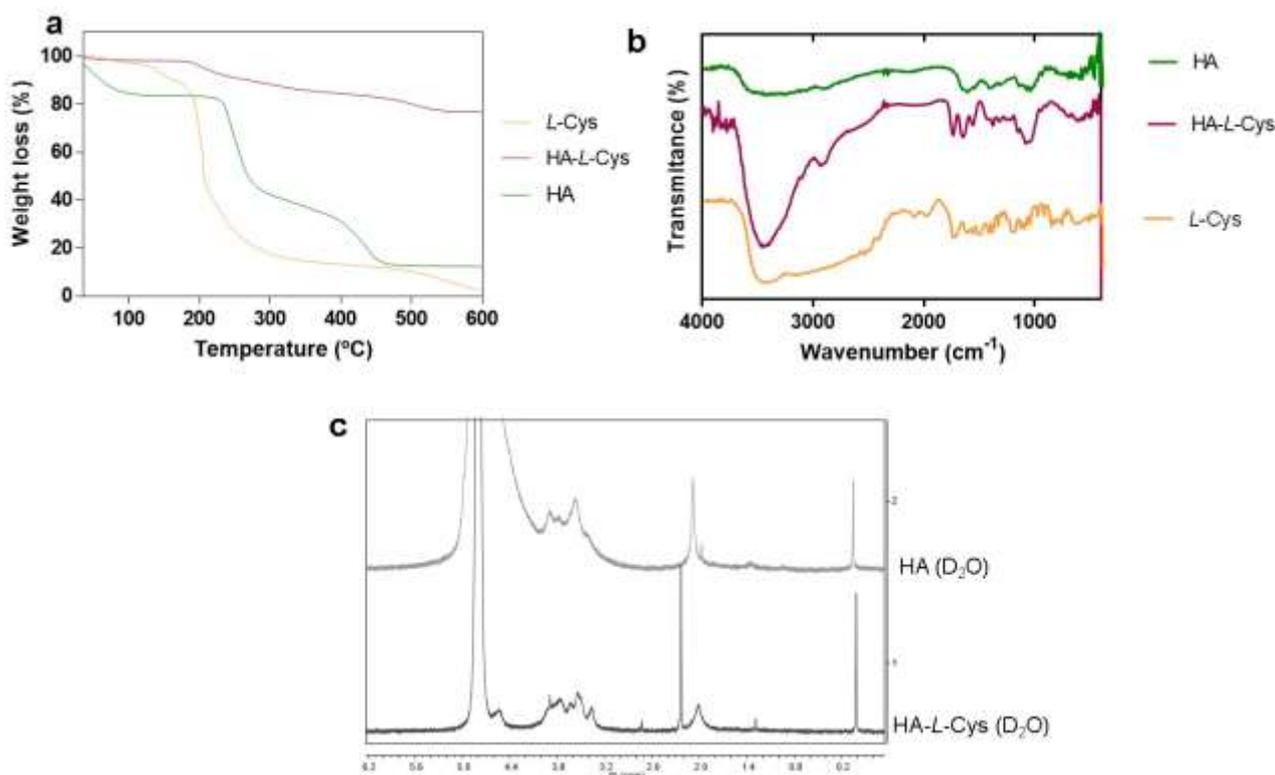
**Figure S4:** a) TGA curves and b) FT-IR spectra of the HA-*L*-Cys bioconjugate polymer and its precursors (hyaluronic acid (HA) and *L*-Cysteine (*L*-Cys)). c) <sup>1</sup>H NMR analysis of the bioconjugate and unmodified polymer HA.
