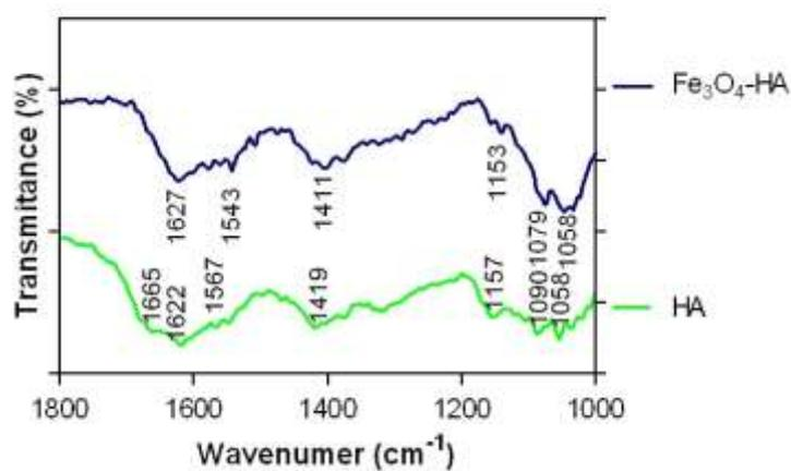
**Figure S6:** FT-IR spectra for HA and Fe<sub>3</sub>O<sub>4</sub>-HA HMNP.
