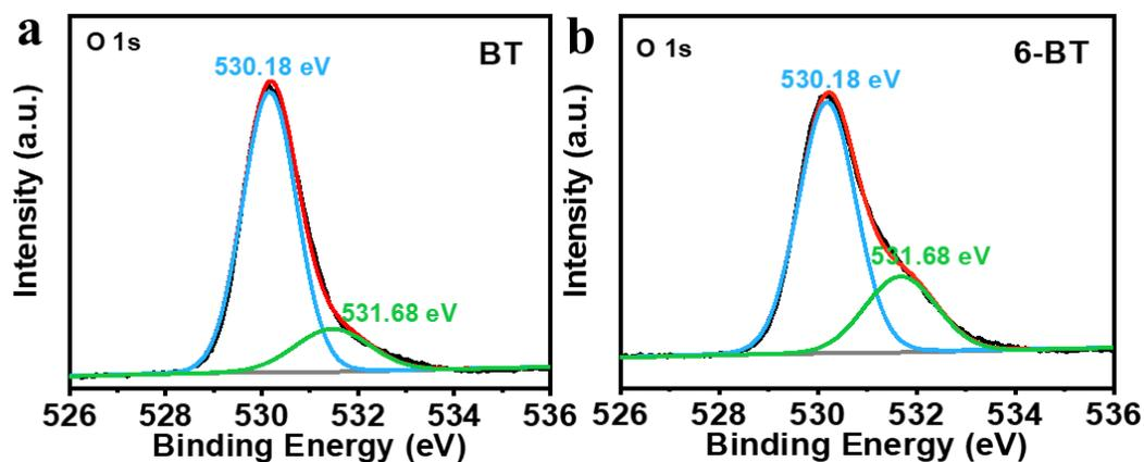
Fig. S2 XPS high-resolution spectra of (a) O 1s of BT and (b) O 1s of 6-BT.
