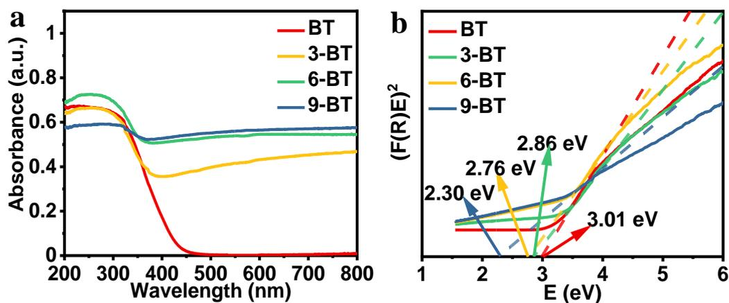
Fig. S3 (a) UV-vis diffuse reflection spectrum and (b) estimated bandgap of BT and X-BT (X=3, 6, 9).
