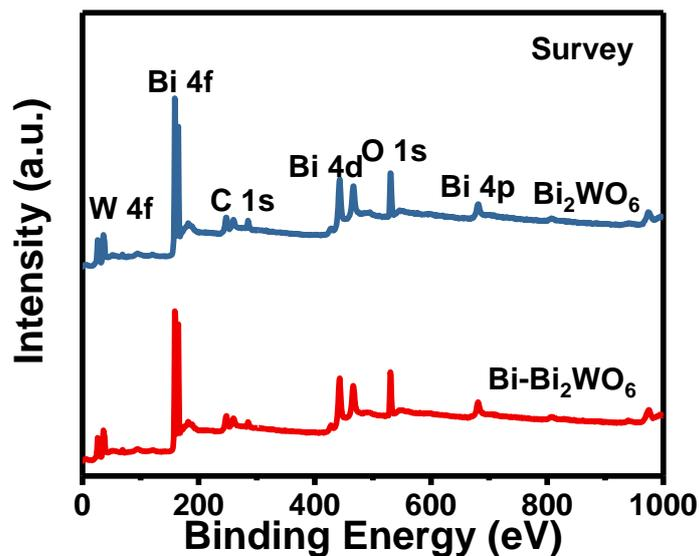
Fig. S1 XPS spectra of original  $\text{Bi}_2\text{WO}_6$  and 6-BT.
