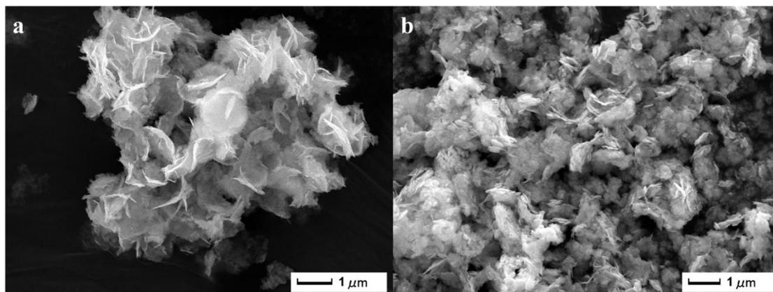
**Fig. S7** SEM images of 6-BT before (a) and after (b) the photocatalytic  $\text{CO}_2$  reduction reaction.
