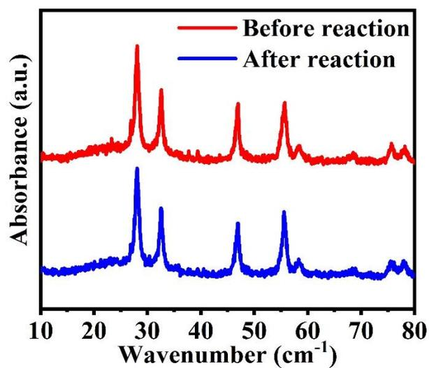
**Fig. S6** XRD patterns of 6-BT before and after the photocatalytic  $\text{CO}_2$  reduction reaction.
