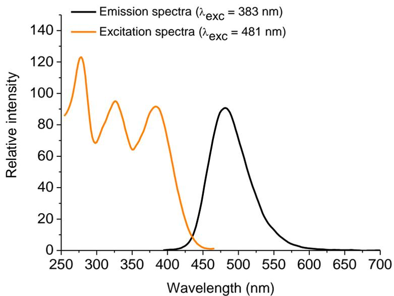
**Figure S43.** Steady-state emission and excitation spectra ( $[ ] = 10^{-6}$  M range) of derivative **6** in CH<sub>3</sub>CN solution.
