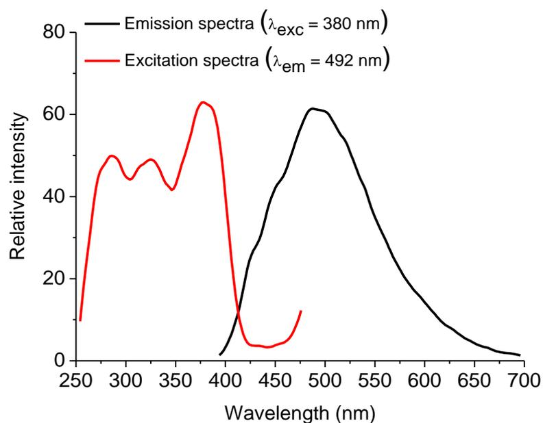
**Figure S46.** Steady-state emission and excitation spectra ( $[ ] = 10^{-6}$  M range) of derivative **4** in DMSO solution.
