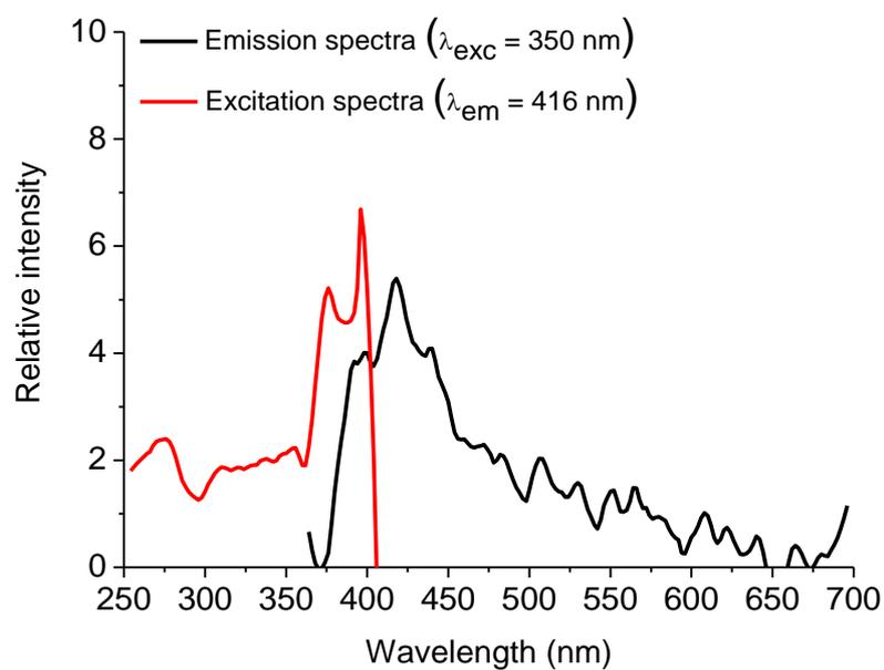
**Figure S45.** Steady-state emission and excitation spectra ( $[ ] = 10^{-6}$  M range) of derivative **3h** in DMSO solution.
