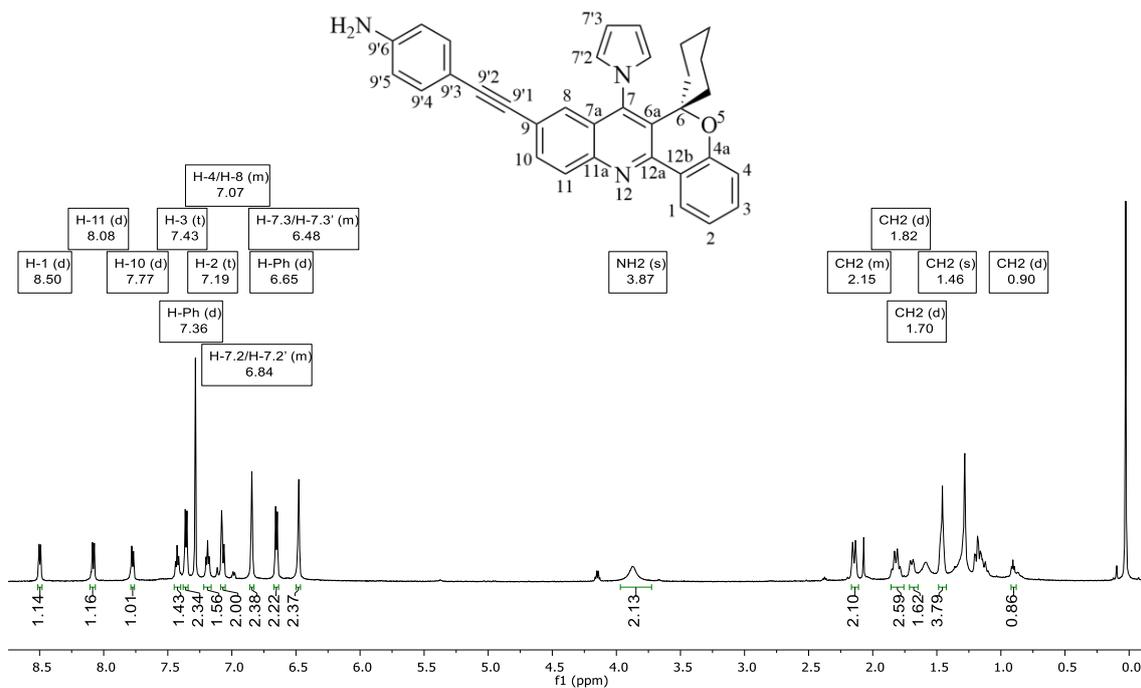
**Figure S30. <sup>1</sup>H NMR spectra at 600 MHz in CDCl<sub>3</sub> of compound 5**
