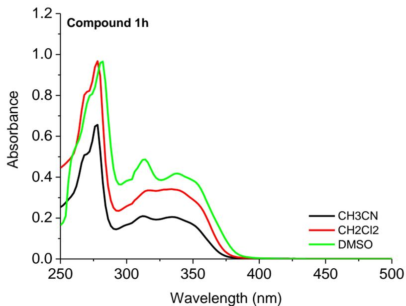
**Figure S34.** UV-Vis ( $[ ] = 10^{-5}$  M range) spectra of derivative **1h**.
