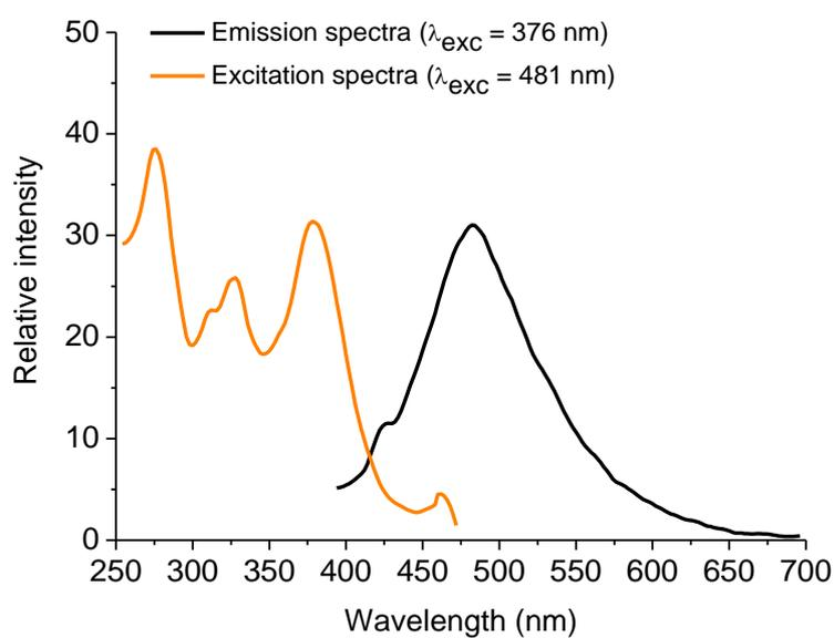
**Figure S41.** Steady-state emission and excitation spectra ( $[ ] = 10^{-6}$  M range) of derivative **4** in CH<sub>3</sub>CN solution.
