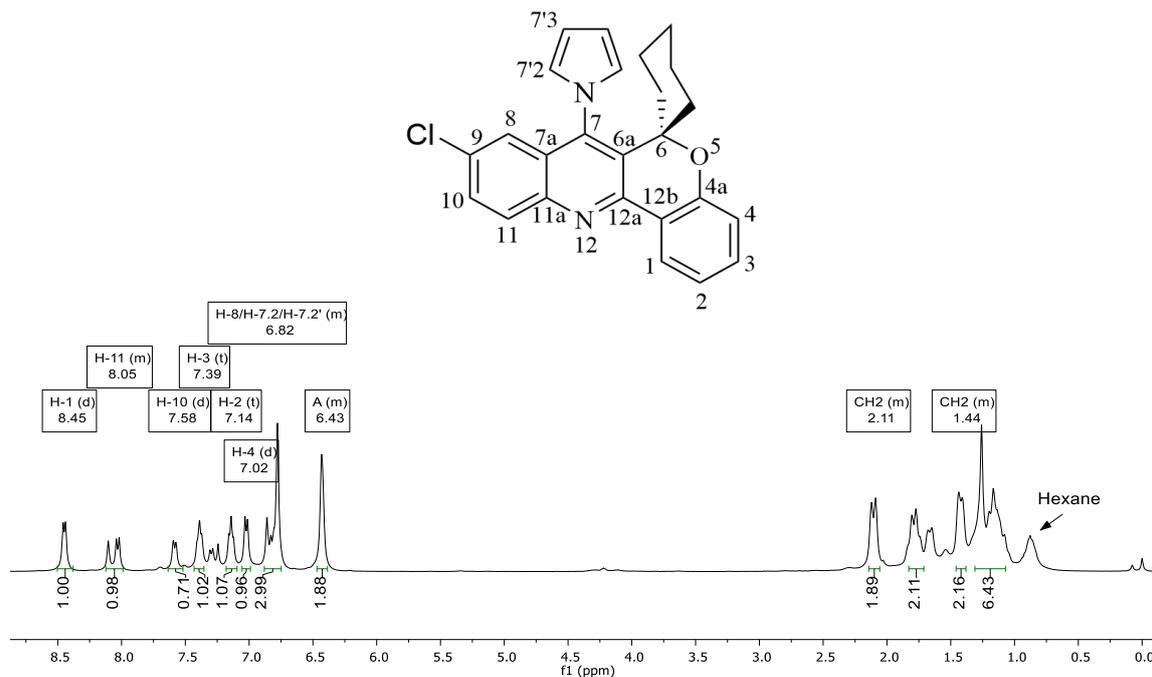
**Figure S16.**  $^1\text{H}$  NMR spectra at 400 MHz in  $\text{CDCl}_3$  of compound **3f**
