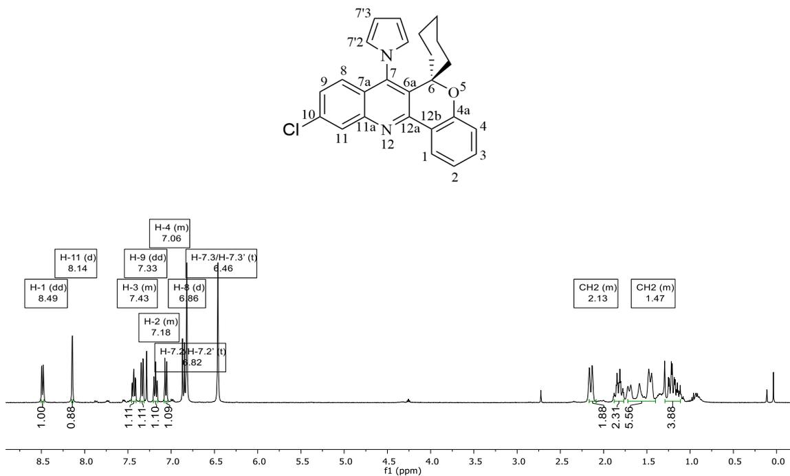
**Figure S24.**  $^1\text{H}$  NMR spectra at 400 MHz in  $\text{CDCl}_3$  of compound **3j**
