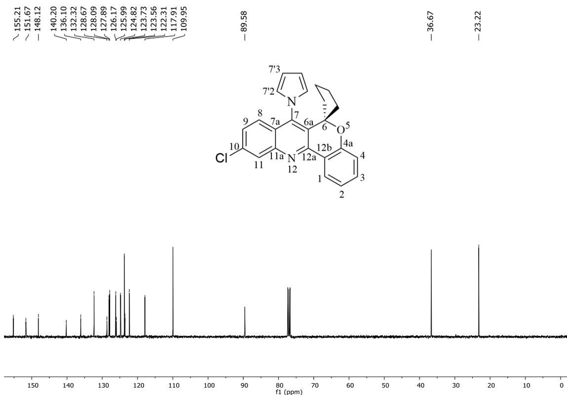
**Figure S23.**  $^{13}\text{C}$  NMR spectra at 100 MHz in  $\text{CDCl}_3$  of compound **3i**
