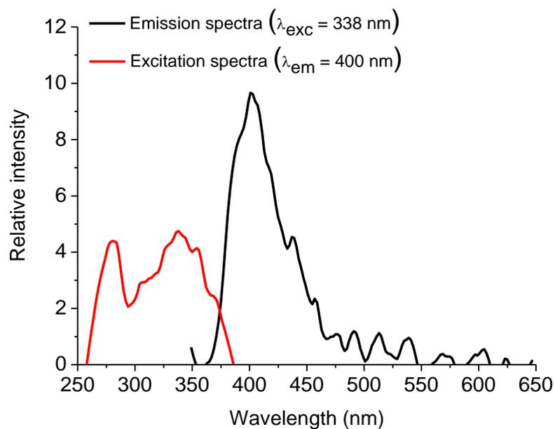
**Figure S44.** Steady-state emission and excitation spectra ( $[ ] = 10^{-6}$  M range) of derivative **1h** in DMSO solution.
