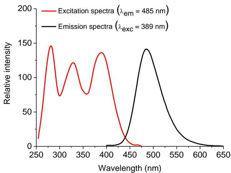
**Figure S48.** Steady-state emission and excitation spectra ( $[ ] = 10^{-6} \text{ M}$  range) of derivative **6** in DMSO solution.
