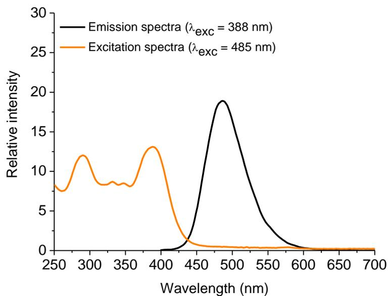
**Figure S42.** Steady-state emission and excitation spectra ( $[ ] = 10^{-6}$  M range) of derivative **5** in CH<sub>3</sub>CN solution.
