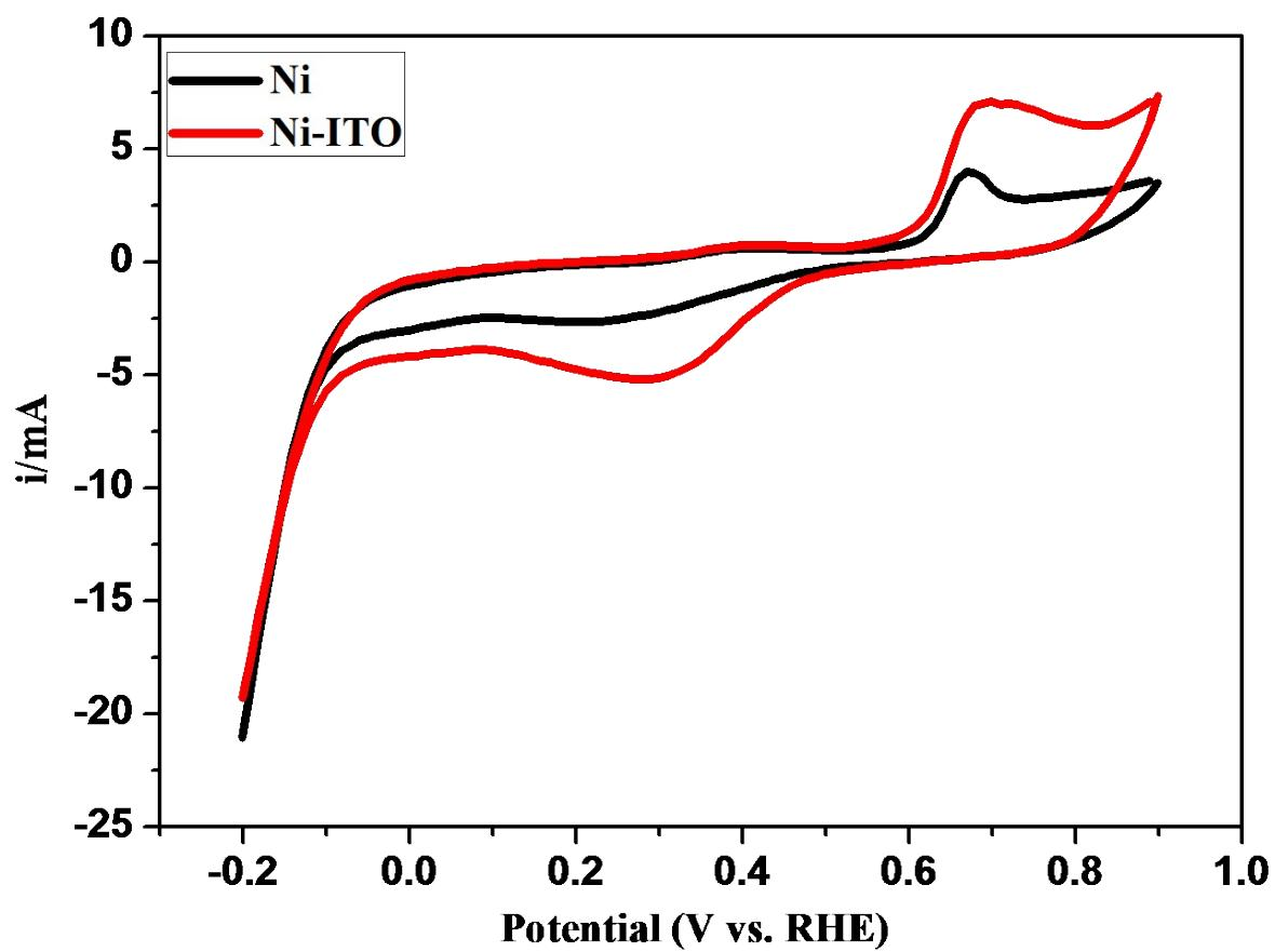
**Fig. S2** Cyclic voltammograms of Ni and Ni-ITO nanocomposites electrodes in 1 M KOH solution at 50  $\text{mVs}^{-1}$  in the cathodic region.
