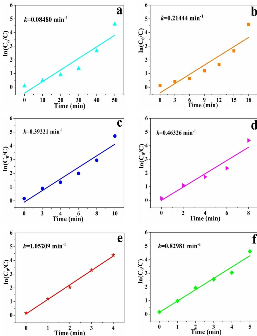
**Fig. S3** The quasi-first-order kinetic curves of AWO-based samples towards RhB degradation under simulated sunlight: (a) AWO, (b) AgBr/AWO-3%, (c) AgBr/AWO-6%, (d) AgBr/AWO-13%, (e) AgBr/AWO-20%, and (f) AgBr/AWO-24%.
