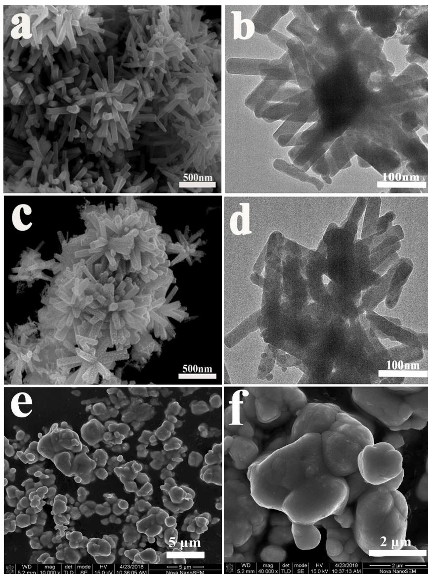
**Fig. S1** (a, b) SEM and TEM images of AWO clusters, (c, d) SEM and TEM images of AWO AgBr/AWO-20%, and (e-f) SEM images of AgBr microparticels.
