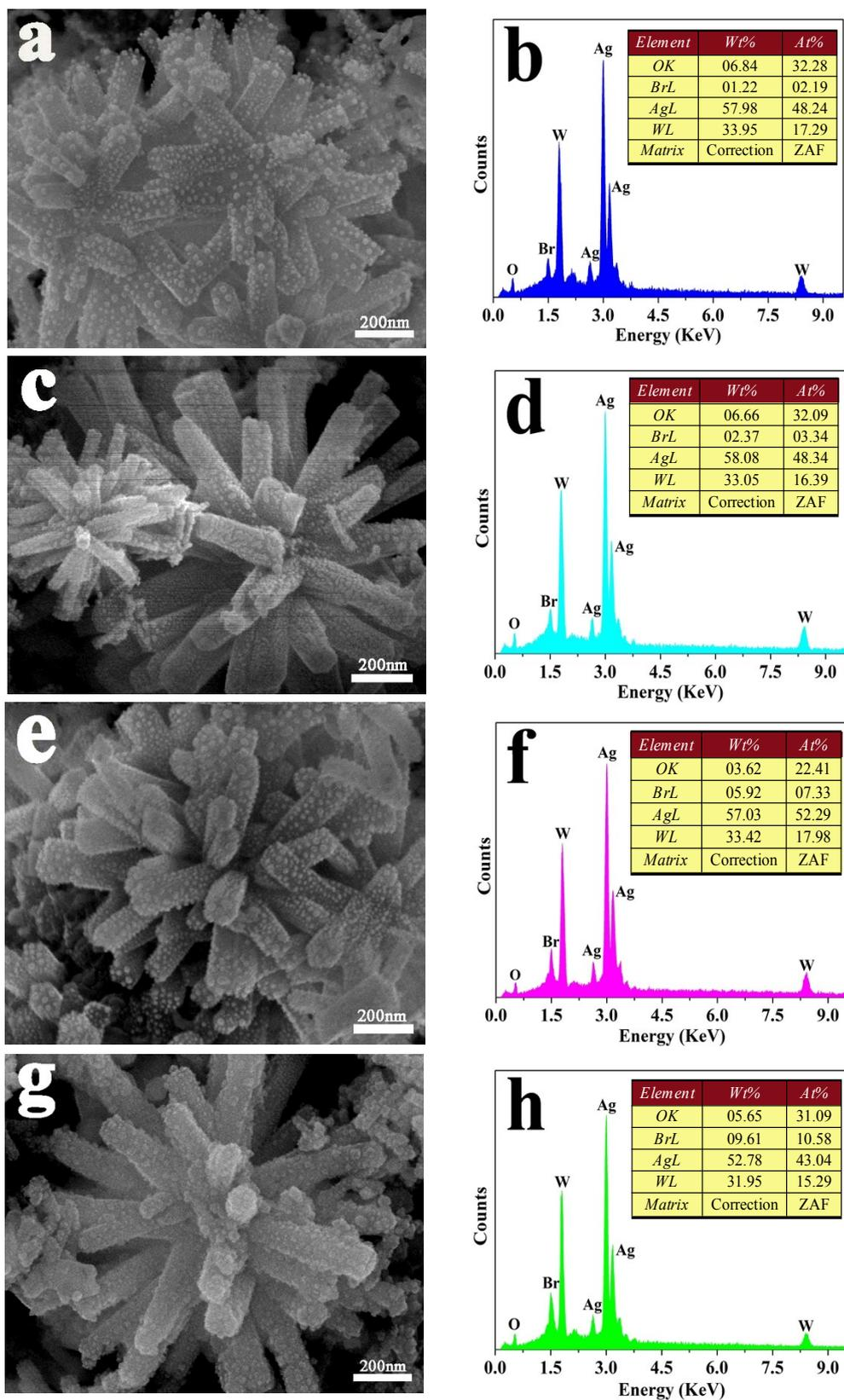
**Fig. S2** SEM images and corresponding EDS of the samples: (a, b) AgBr/AWO-3%, (c, d) AgBr/AWO-6%, (e, f) AgBr/AWO-13% and (g, h) AgBr/AWO-24%.
