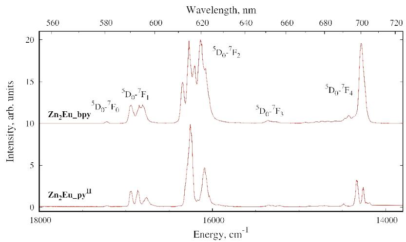
**Fig. S9.** Luminescence spectra of  $\text{Zn}_2\text{Eu\_bpy}$  (a) and  $\text{Zn}_2\text{Eu\_py}^{\text{II}}$  (b) recorded at  $\lambda_{\text{ex}} = 340$  nm and  $T = 77$  K.
