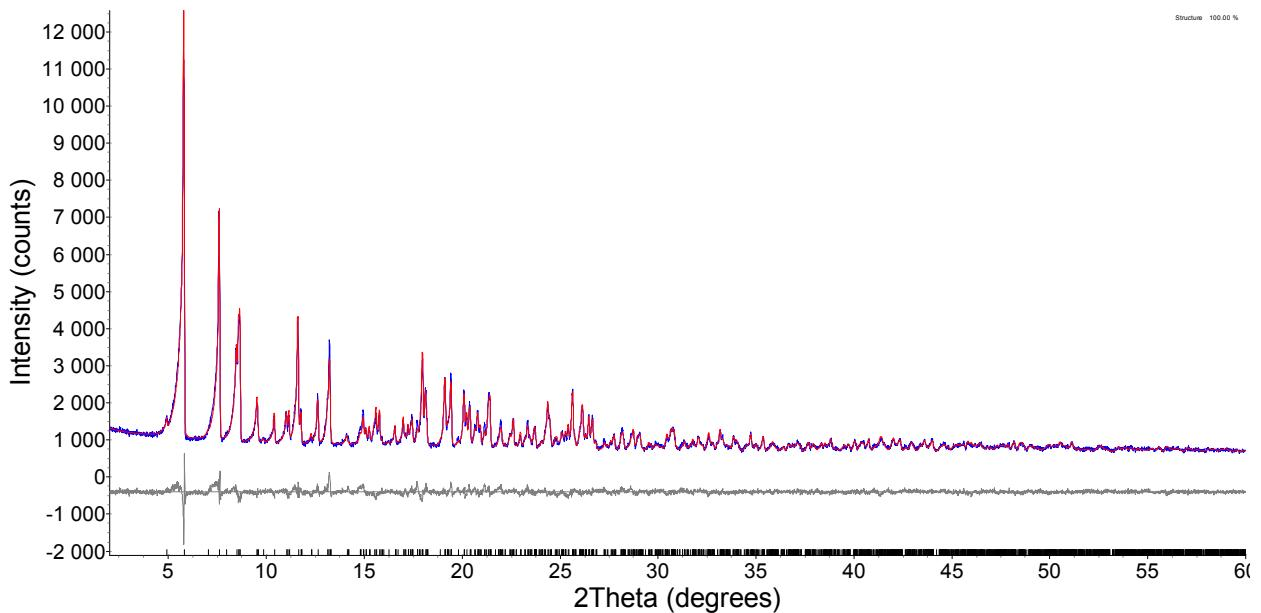
**Fig. S1.** Theoretical (red line) and experimental (blue line) patterns of **Zn<sub>2</sub>Eu\_py<sup>II</sup>** and their difference (grey line).
