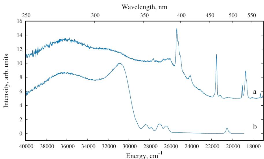
**Fig. S10.** Excitation spectra of  $[\text{Eu}(\text{phbz})_3]_n$  (a,  $\lambda_{\text{em}} = 615$  nm) and  $[\text{Tb}(\text{phbz})_3]_n$  (b,  $\lambda_{\text{em}} = 545$  nm) recorded at  $T = 300$  K.
