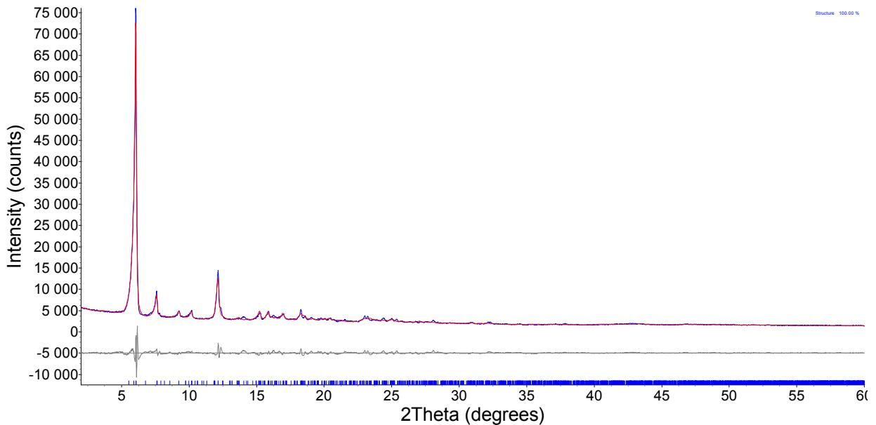
**Fig. S4.** Theoretical (red line) and experimental (blue line) patterns of **Zn<sub>2</sub>Eu\_lut** and their difference (grey line).
