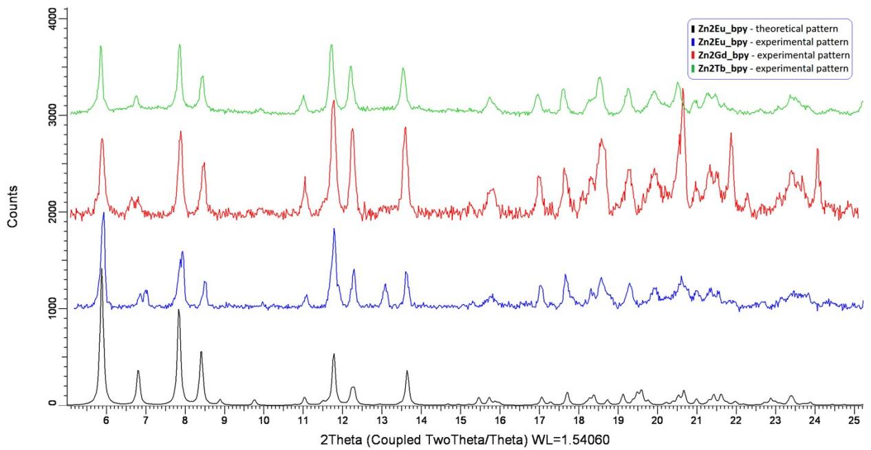
**Fig. S5.** Theoretical (black line) and experimental patterns of **Zn<sub>2</sub>Eu\_bpy** (blue line), **Zn<sub>2</sub>Gd\_bpy** (red line) and **Zn<sub>2</sub>Tb\_bpy** (green line).
