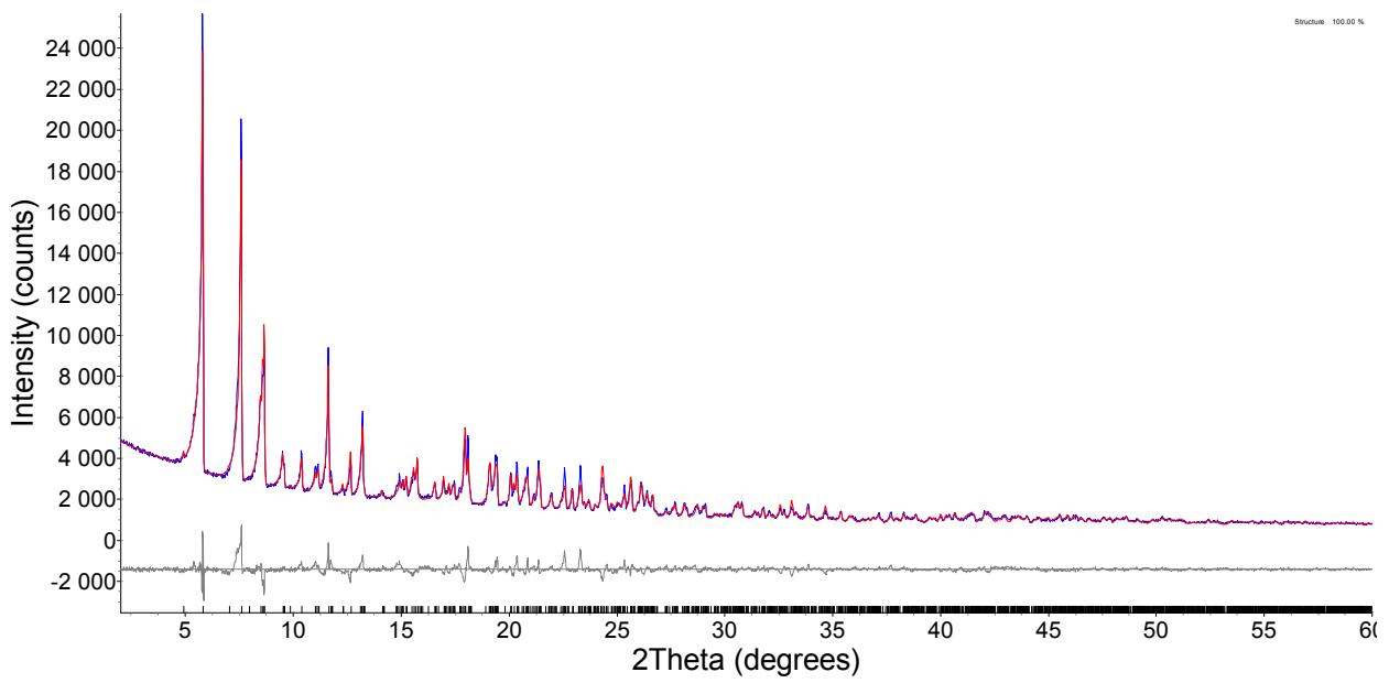
**Fig. S3.** Theoretical (red line) and experimental (blue line) patterns of **Zn<sub>2</sub>Tb\_py** and their difference (grey line).
