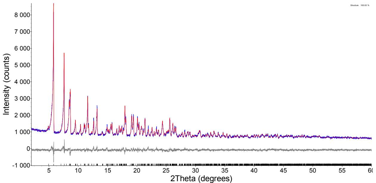
**Fig. S2.** Theoretical (red line) and experimental (blue line) patterns of **Zn<sub>2</sub>Gd\_py** and their difference (grey line).
