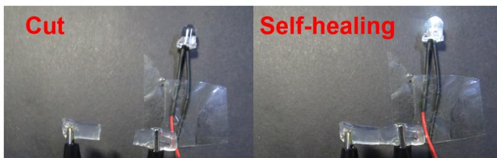
**Fig. S8** The luminance variation of LED during self-healing processes.
