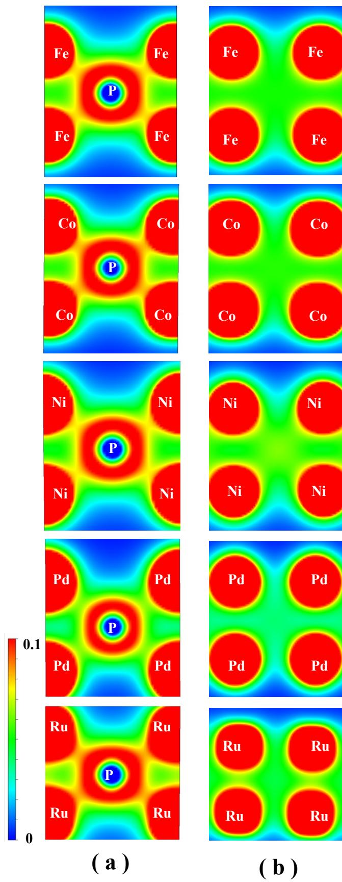
**Fig. S2** The charge density for TM<sub>2</sub>P monolayers on (a) (1 1 0) and (b) (0 1 0) face.
