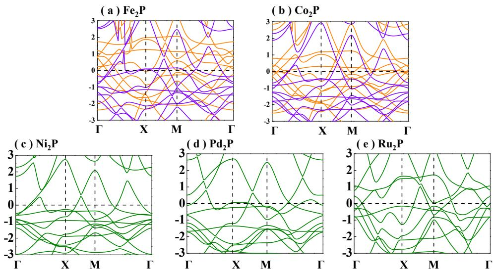
**Fig. S8** The band structures of 2D (a)  $\text{Fe}_2\text{P}$  and (b)  $\text{Co}_2\text{P}$ , (c)  $\text{Ni}_2\text{P}$ , (d)  $\text{Pd}_2\text{P}$  and (e)  $\text{Ru}_2\text{P}$  under critical tensile strain, respectively. The Fermi level is set to zero.
