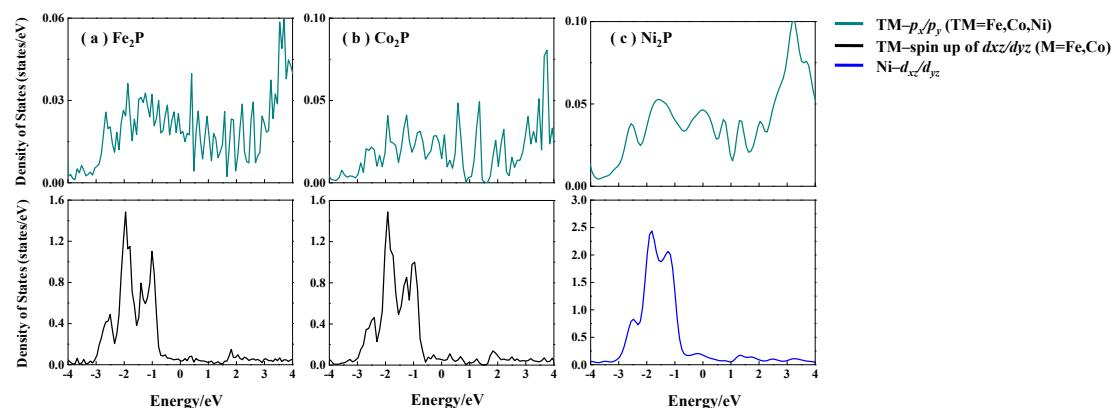
**Fig. S10** The orbital project density of states of (a) Fe<sub>2</sub>P, (b) Co<sub>2</sub>P and (c) Ni<sub>2</sub>P, respectively. The Fermi level is set zero.
