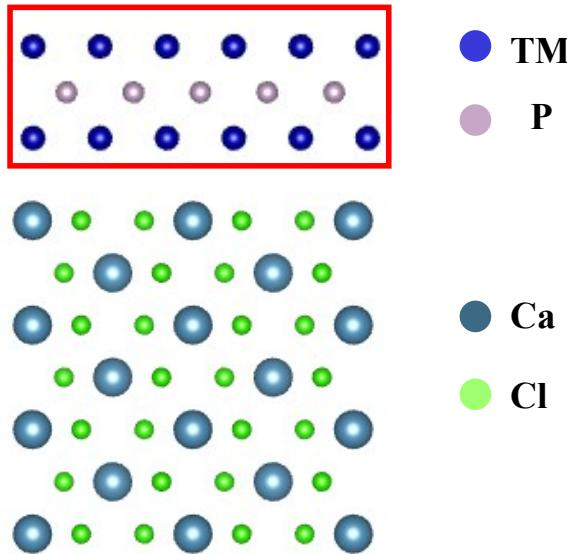
**Fig. S4** Schematic representation of  $\text{TM}_2\text{P}$  grown on the surface of  $\text{CaCl}_2$ .
