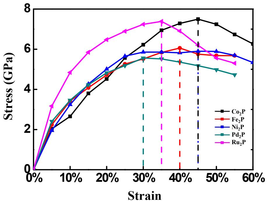
**Fig. S6** The uniaxial tensile stress-strain response of 2D TM<sub>2</sub>P monolayers along [100] direction.
