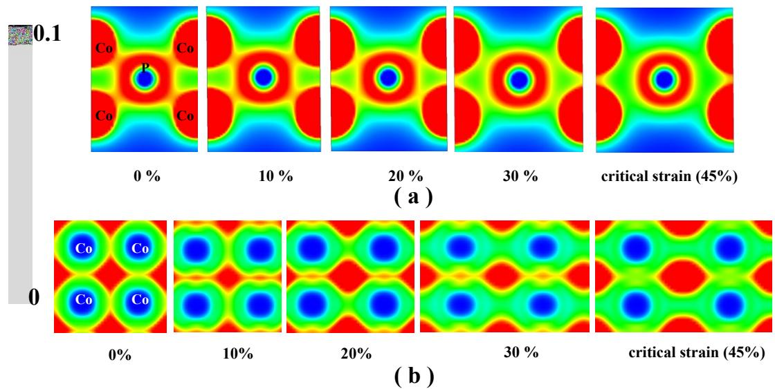
**Fig. S7** (a) Charge density on  $(110)$  face and (b) isosurface of electron localization function (ELF) on  $(001)$  face of  $\text{Co}_2\text{P}$  under various tensile strains.
