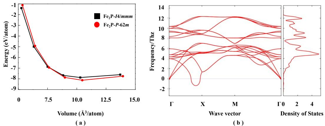
**Fig. S3** (a) Total energy variations along with unit cell volume change for the  $I4/mmm$  and  $P-62m$  phase. (b) Phonon dispersions of  $I4/mmm$   $\text{Fe}_2\text{P}$  along  $\Gamma - X - M - \Gamma$  directions in Brillouin zone.
