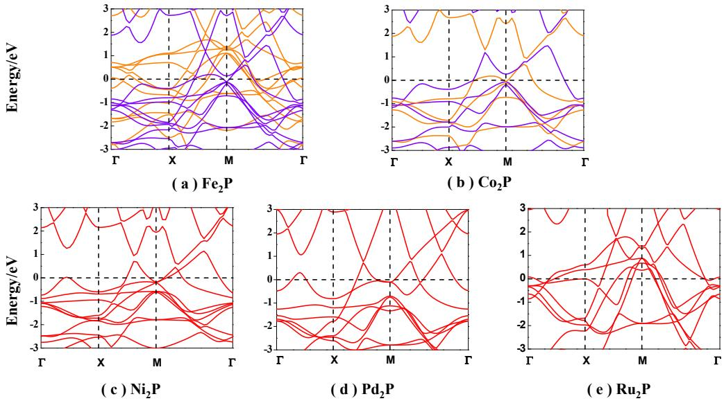
**Fig. S5** The band structures of 2D (a)  $\text{Fe}_2\text{P}$ , (b)  $\text{Co}_2\text{P}$ , (c)  $\text{Ni}_2\text{P}$ , (d)  $\text{Pd}_2\text{P}$  and (e)  $\text{Ru}_2\text{P}$ . The purple and orange lines are spin-up and down bands. The Fermi level is set to zero.
