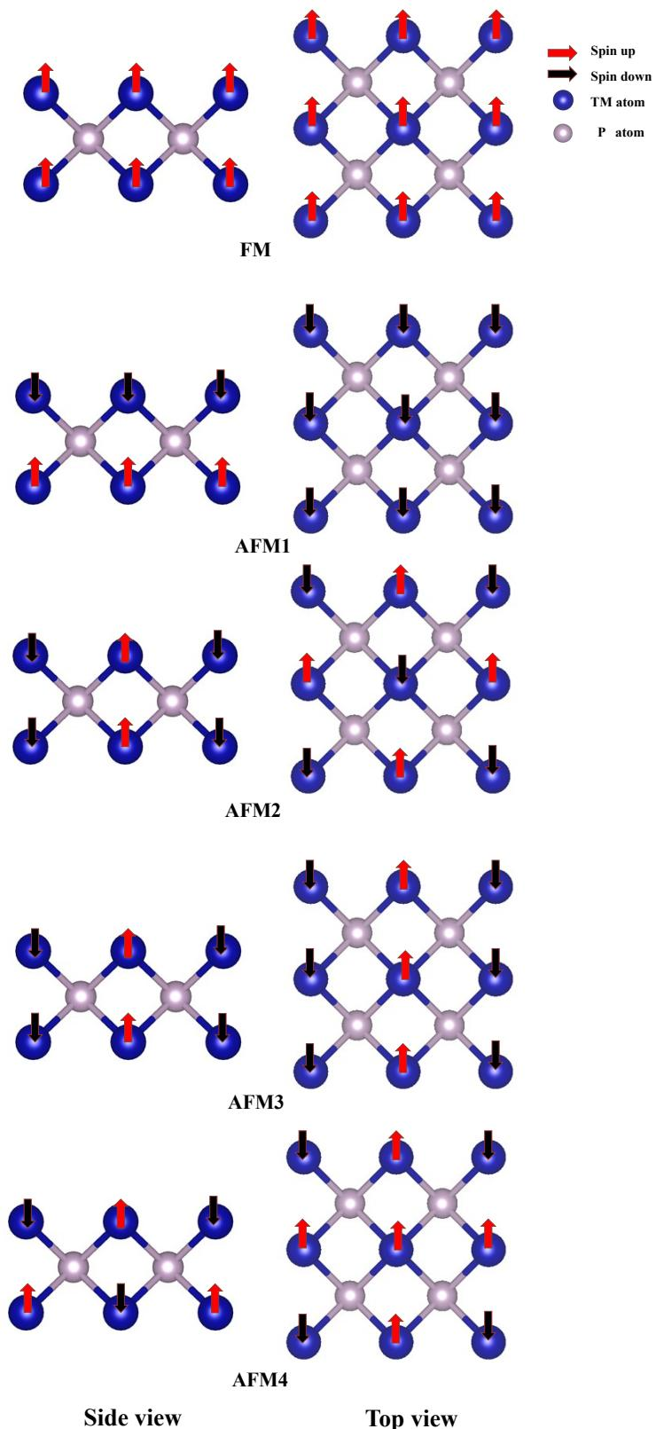
**Fig. S9** Schematic diagrams for Fe<sub>2</sub>P and Co<sub>2</sub>P monolayers in FM and various AFM magnetic configurations. The blue and pink balls represent TM (Fe, Co) and P atoms, respectively.
