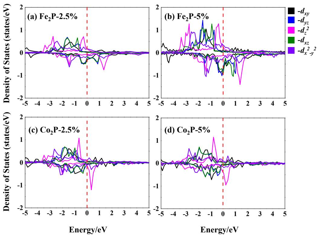
**Fig. S12** The orbital projected density of states for  $\text{Co}_2\text{P}$  and  $\text{Fe}_2\text{P}$  monolayers under tensile strains.
