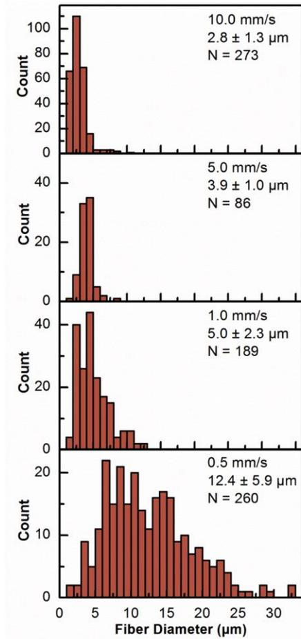
Figure S2: Histograms of 0.0035 gR6G/gPVA fiber size electrospun using stage speeds of 10.0 mm/s, 5.0 mm/s, 1.0 mm/s, and 0.5 mm/s.
