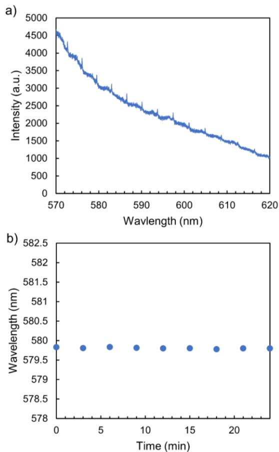
Figure S8: a) Representative fluorescence spectrum of a crosslinked R6G-PVA fiber in water. The spectrum was taken with a 50x long working distance objective under 532 nm CW illumination, using conditions similar to ethanol-water chemical sensing. The shutter was closed between measurements. b) The peak wavelength as a function of measurement time for mode near 580 nm. WGM resonance wavelength remains stable over time.
