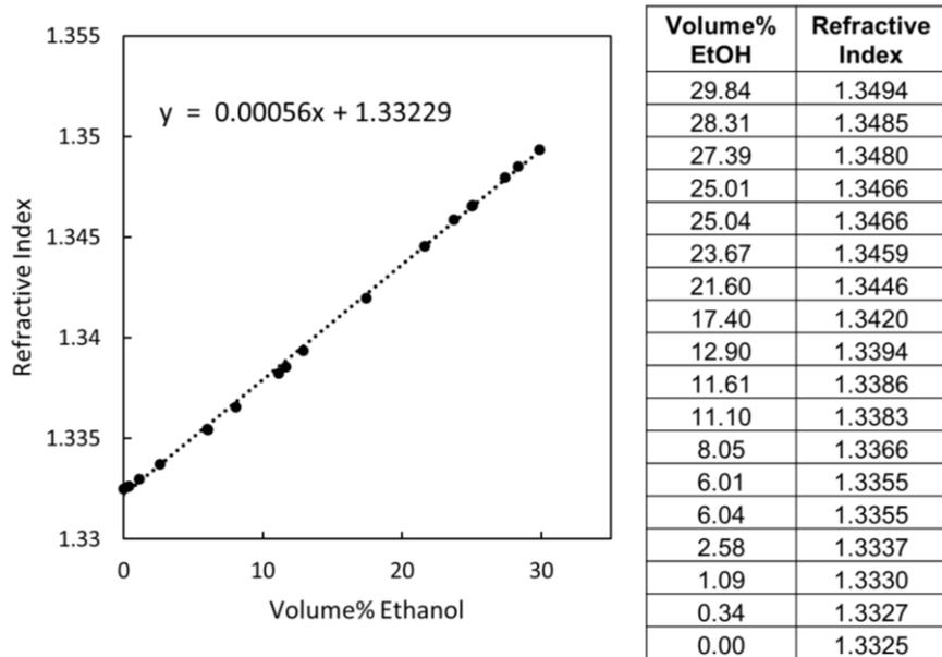
Figure S1: A plot of data and table of values which were obtained from Scott et al<sup>1</sup>, and used to calculate the refractive indices of ethanol-water solutions used for sensing experiments.
