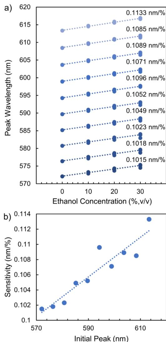
Figure S9: a) Peak emission wavelength as a function of ethanol concentration for the same 15.9  $\mu\text{m}$  fiber shown in Figure 7. b) Plot of sensitivity versus wavelength for each resonance peak. Sensor sensitivity increases for longer wavelength.
