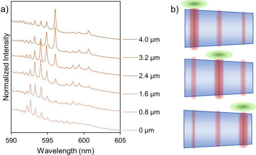
Figure S5: a) Spectra taken at 0.8  $\mu\text{m}$  increments along the length of a 4.2  $\mu\text{m}$  diameter fiber. b) A schematic representation of spectral measurements at three different axial positions along the length of the fiber.
