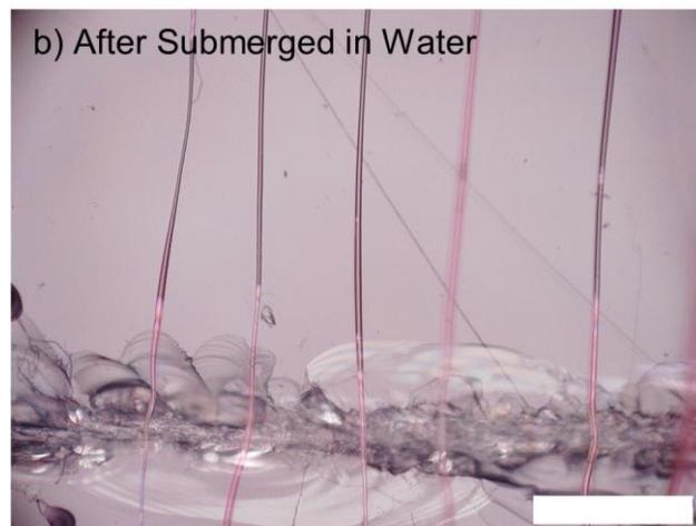
Figure S7: Optical images of crosslinked R6G-PVA fibers a) before and b) after immersion in water for 24 h. The fibers were water stable. Scale bar: 200  $\mu\text{m}$ .
