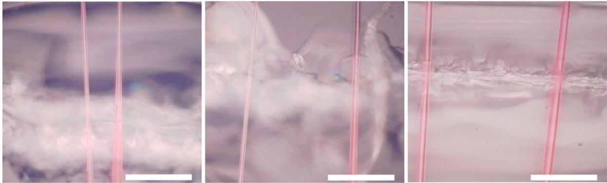
Figure S4: Optical microscopy images illustrating the range and degree of diameter variation observed in dye-doped, electrospun PVA fibers on a glass substrate. Background depicts the scribed trench over which the fibers were suspended. Scale bar: 100  $\mu\text{m}$ .
