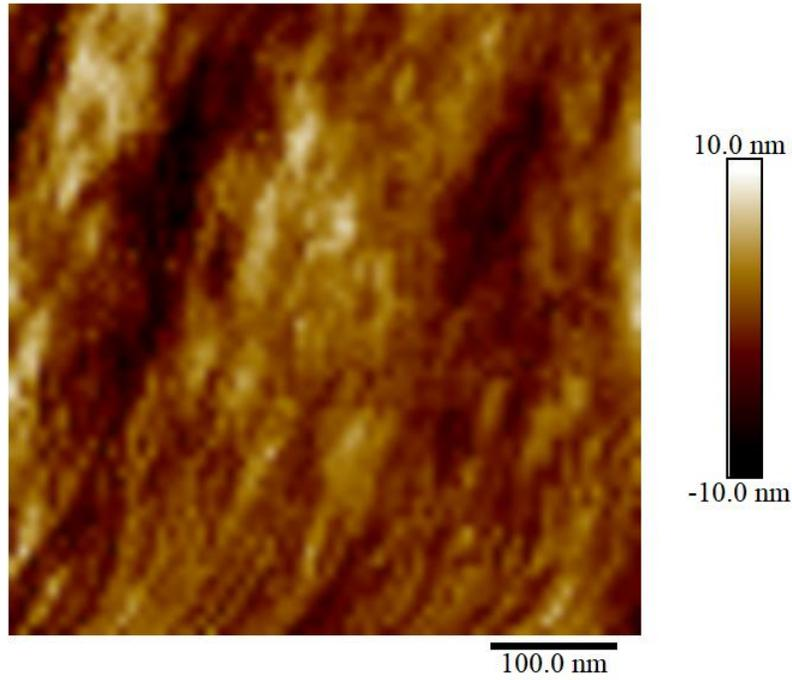
Figure S3: AFM image of the surface of a dye-doped PVA fiber electrospun with a stage speed of  $0.5 \text{ mm s}^{-1}$  and a R6G/PVA mass ratio of 0.0035. The measured root-mean-squared roughness was 2.4 nm.
