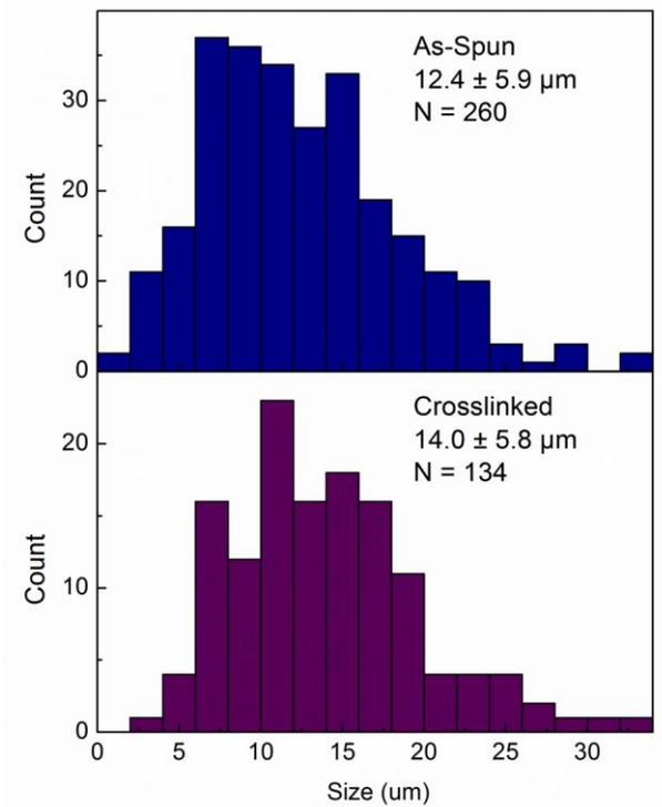
Figure S6: Histogram of as-spun and crosslinked R6G-PVA fiber size electrospun using a stage speed of 0.5 mm/s. A small increase in fiber diameter was caused by glutaraldehyde crosslinking treatment.
