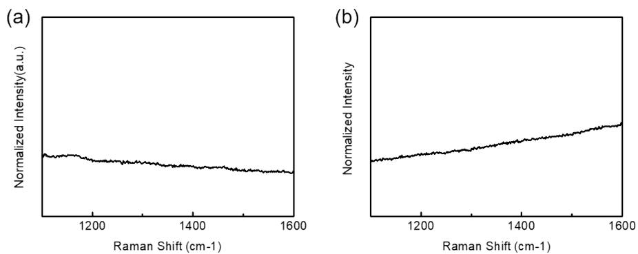
Figure S2. (a-b) Raman spectra of glucose absorbed onto monolayer MoS<sub>2</sub> and MoSe<sub>2</sub>. No visible peaks were observed because of weak interactions of glucose and MoS<sub>2</sub> and MoSe<sub>2</sub>.
