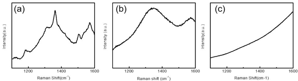
Figure S3. Raman spectra of glucose on monolayer Janus with various excitation lasers. (a) 532 nm laser (b) 633 nm laser (c) 785 nm laser. Raman spectra with 633 nm and 785 nm laser only show two wide peaks and a high broad background. Careful deconvolution is needed to identify hidden peaks in the broad peaks and background.
