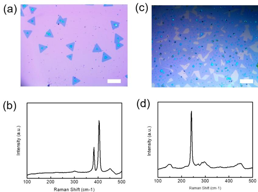
Figure S1. (a-b) Optical images and Raman spectra of CVD-grown monolayer MoS<sub>2</sub>. (c-d) Optical images and Raman spectra of CVD-grown monolayer MoSe<sub>2</sub>. Scale bar is 50  $\mu\text{m}$ .
