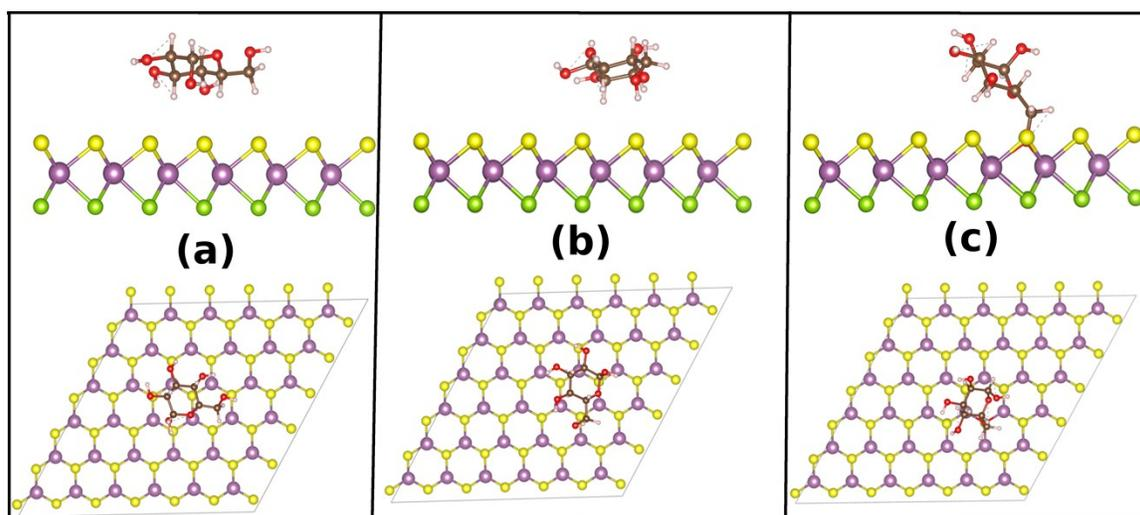
Figure S5. Various configurations of glucose on monolayer Janus. The grey, red and white atoms are carbon, oxygen and hydrogen in glucose respectively. The yellow, purple and green atoms are sulfur, molybdenum and selenium in Janus respectively. (a) the free  $\text{CH}_2\text{OH}$  group of glucose pointing away from the surface. (b) the free  $\text{CH}_2\text{OH}$  group of glucose pointing towards the surface. (c) glucose is covalently bonded onto Janus.
