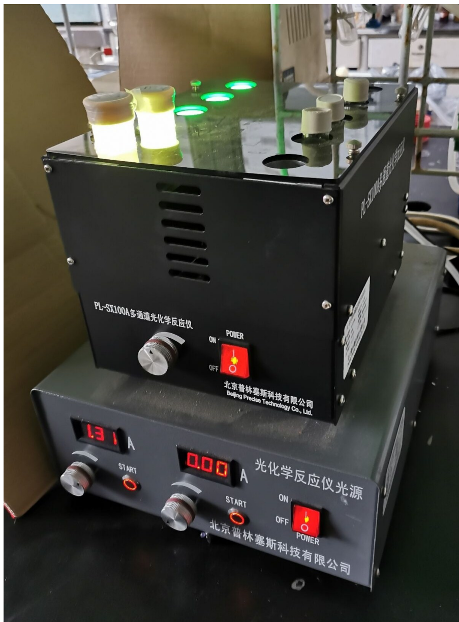
Figure S7. Experimental setup for photo-polymerization using blue LED light.
