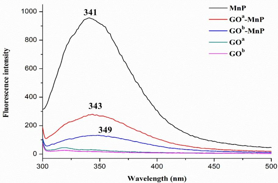
**Fig. S1.** Fluorescence spectra of MnP and GO-MnP. The MnP concentration was 100  $\mu\text{g}/\text{mL}$  in 0.01 M sodium acetate buffer solutions (1 mL, pH 5.9), and GO concentration was 30 and 60  $\mu\text{g}/\text{ml}$  (GO<sup>a</sup> and GO<sup>b</sup>) , respectively.
