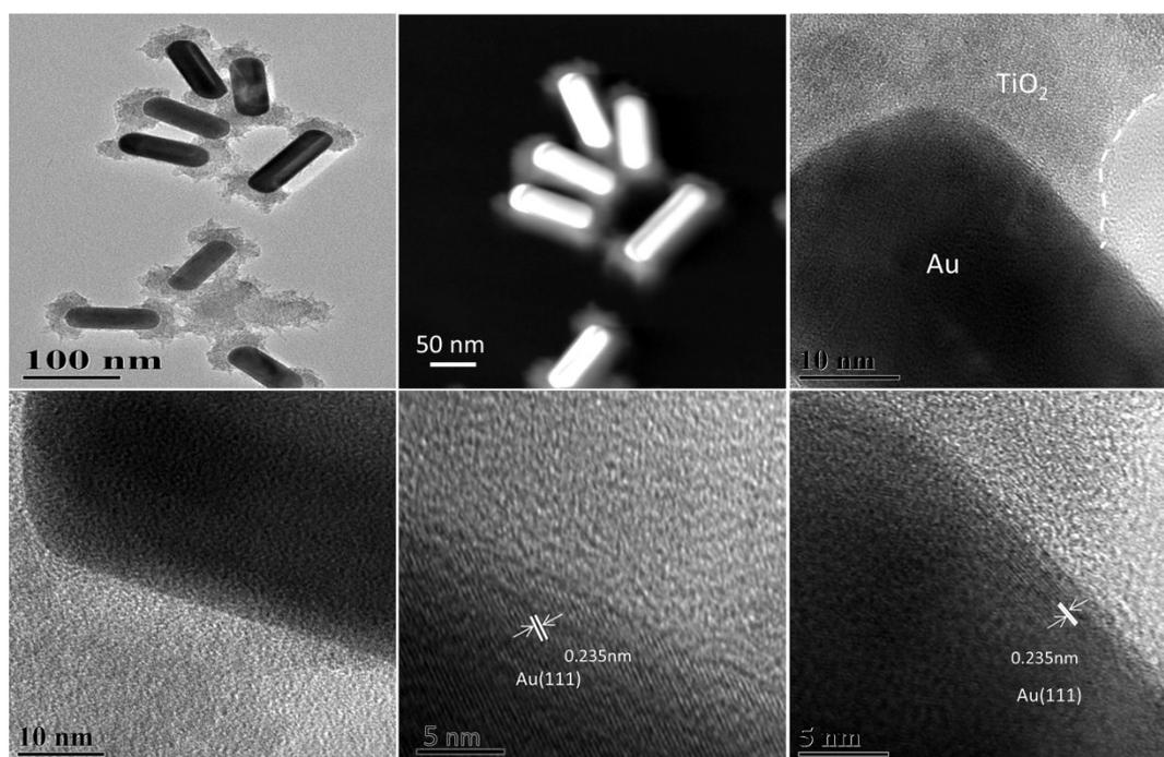
**Figure S2** (a) TEM (b) STEM and (c-f) HRTEM images of Au-TiO<sub>2</sub> nanodumbbell. (c-f) corresponding HRTEM images from parts indicated in Figure 2b.
