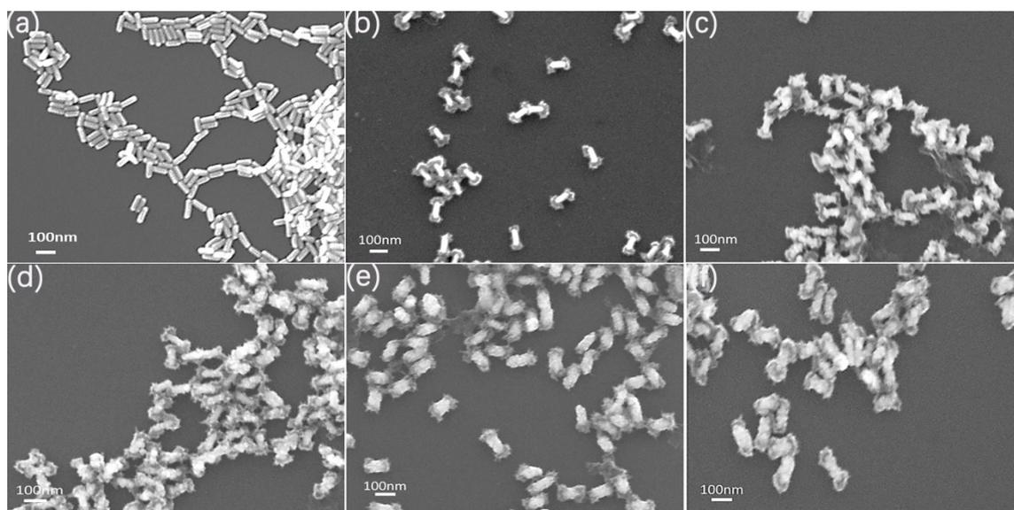
**Figure S4** (a) SEM of bare Au NRs (b-f) SEM images of Au-TiO<sub>2</sub>-Pt with different amounts of 2 mM Pt (b: 0 ul, c: 25 ul, d: 50 ul, e: 100 ul, f: 200 ul).
