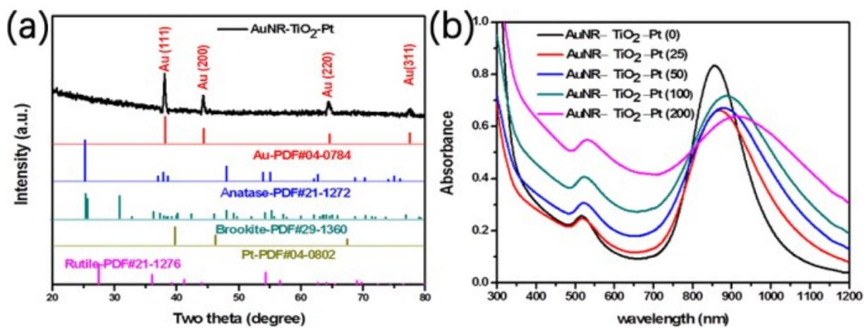
**Figure S6** (a) XRD patterns of AuNR-TiO<sub>2</sub>-Pt (50ul), (b) UV-vis absorption spectra of Au-TiO<sub>2</sub>-Pt with different amounts of Pt.
