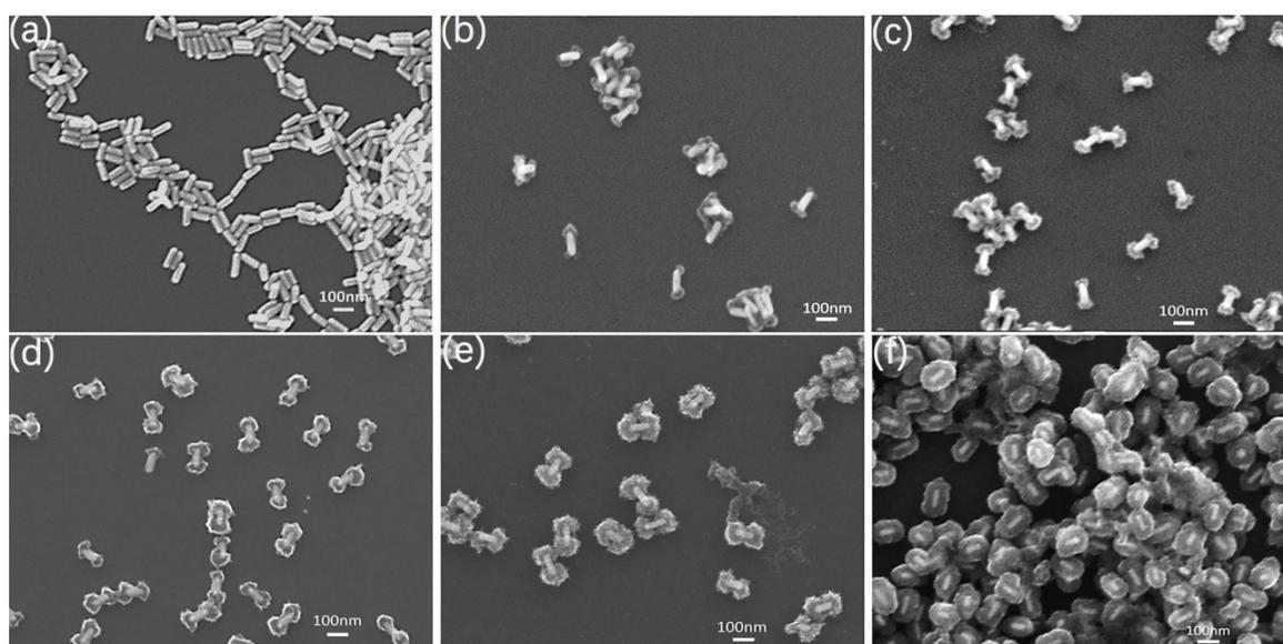
**Figure S3** (a) SEM image of bare Au NRs and (b-f) SEM images of Au-TiO<sub>2</sub> with different reaction time for TiCl<sub>3</sub> (b:10min,c:30min,d:60min,e:120min,f:300min).
