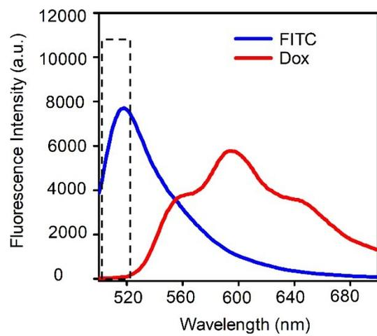
**Figure S14.** Emission spectra of Dox and FITC at the excitation wavelength of 488 nm.
