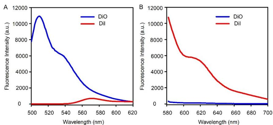
**Figure S12.** Emission spectra of DiO and DiI at the excitation wavelength of 488 nm (A) and 561 nm (B).
