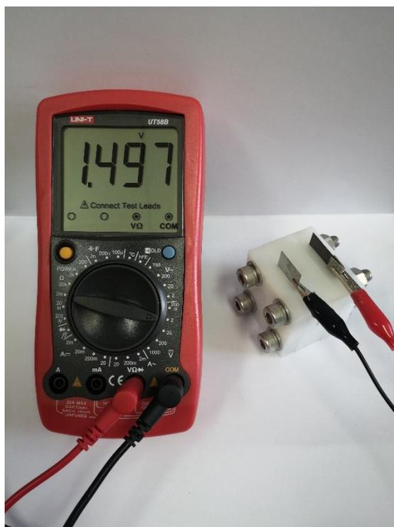
**Figure S6.** Photograph of the Pt/C-RuO<sub>2</sub> based Zn-air battery exhibiting an open circuit voltage of 1.497 V measured with a voltmeter.
