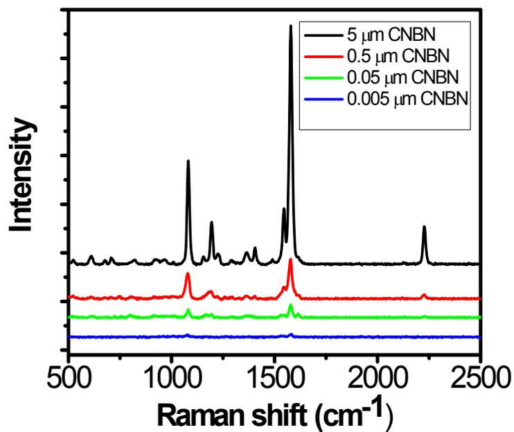
Fig S1. Concentration-dependent SERS spectrum using CNBN Raman reporter
