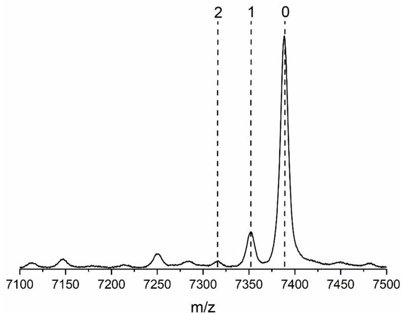
**Figure S8:** Positive ion MALDI-MS spectrum of  $\text{Au}_{25}(\text{PET})_{18-x}(\text{PA})_x$  obtained after mixing  $\text{Au}_{25}(\text{PET})_{18}$  with 10 eq. of lithium phenylacetylide in DCM under argon for 5 minutes. Other peaks correspond to fragmentation products.
