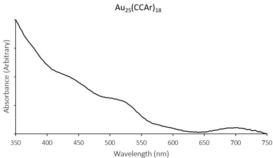
**Figure S10:** UV/Visible absorbance spectrum of crystal-pure  $\text{Au}_{25}(\text{CCAr})_{18}$ . The position and relative intensity of absorption peaks matches well with that reported by Li et al. (reference 3).
