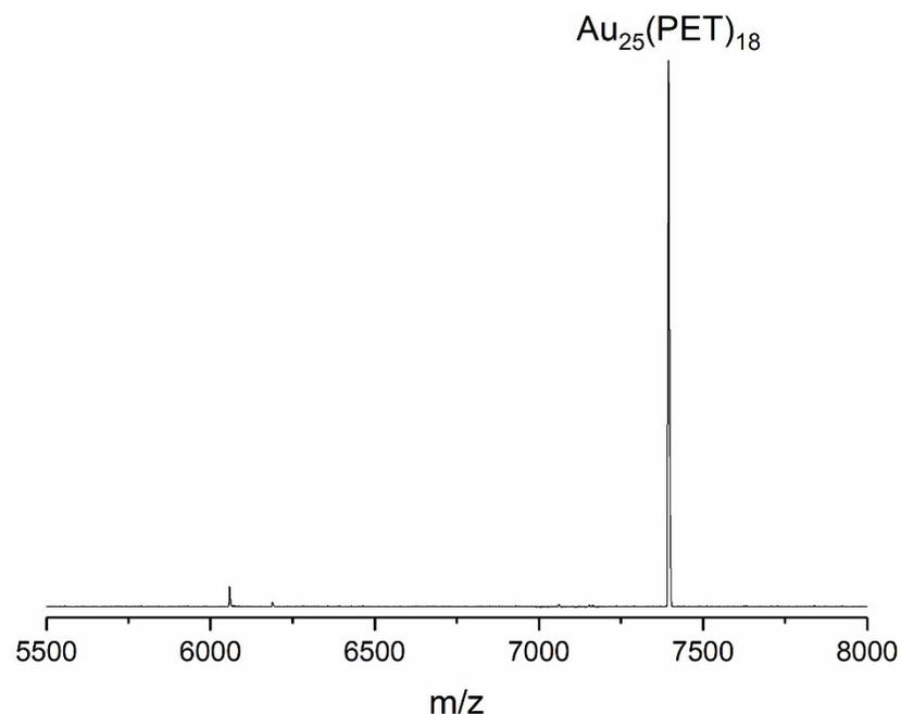
**Figure S1:** Positive ion MALDI-MS of Au<sub>25</sub>(PET)<sub>18</sub>. The peak corresponding to this compound is labelled. Other peaks correspond to fragmentation products.
