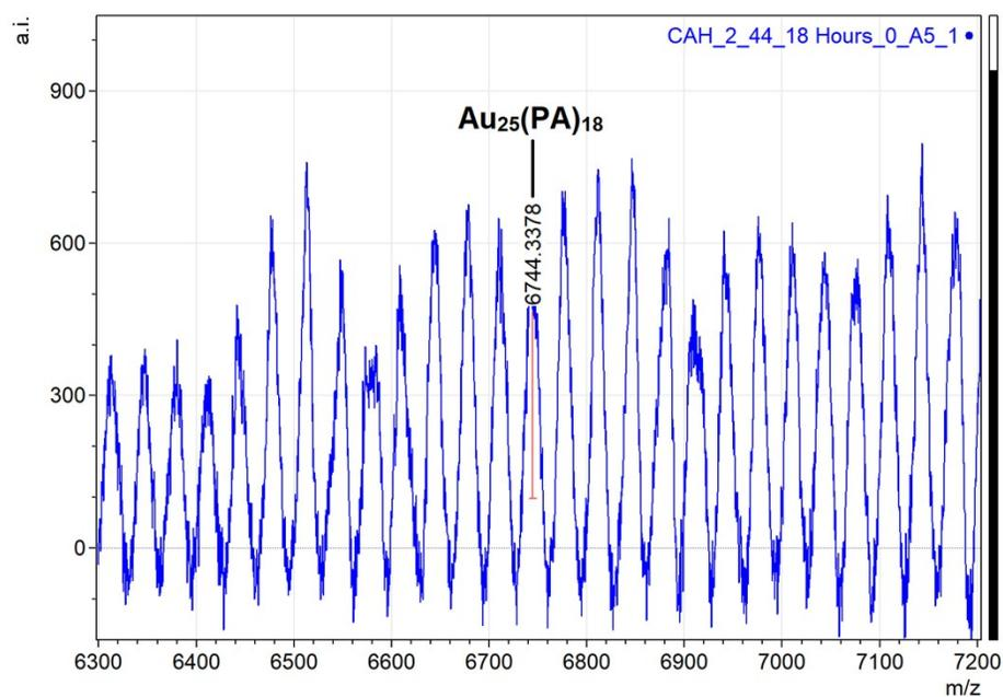
**Figure S7:** Positive ion MALDI-MS spectrum after mixing  $\text{Au}_{25}(\text{PET})_{18}$  with 100 eq. gold(I)-phenylacetylide in DCM for 18 hours. The peak corresponding to the mass of  $\text{Au}_{25}(\text{PA})_{18}$  is labelled.
