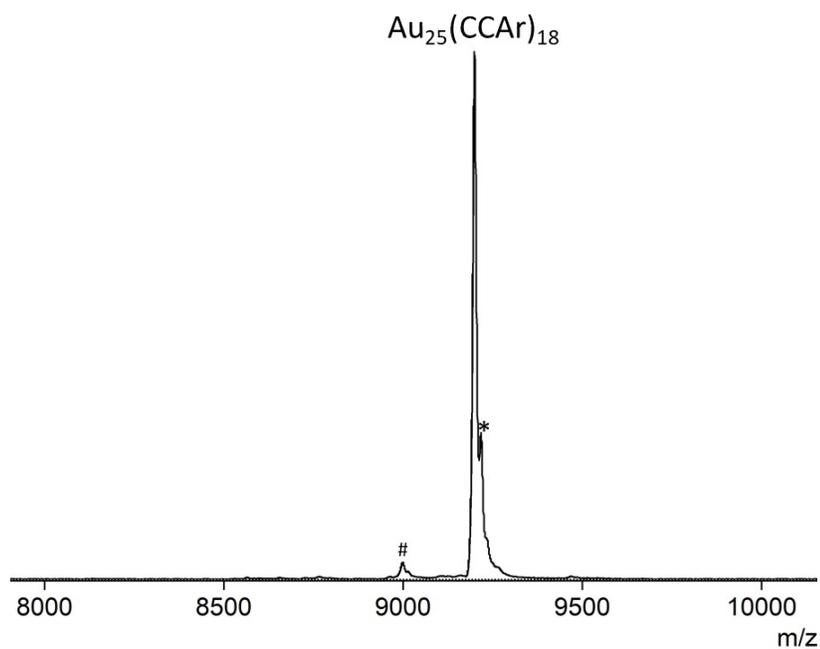
**Figure S9:** Negative ion MALDI-MS spectrum of crystal-pure  $\text{Au}_{25}(\text{CCAr})_{18}$ . The peak corresponding to the compound is labelled. The peak labelled # is a fragment peak corresponding to the loss of gold from the parent cluster. The peak labelled \* is an adduct peak corresponding to the parent peak plus a fluorine.
