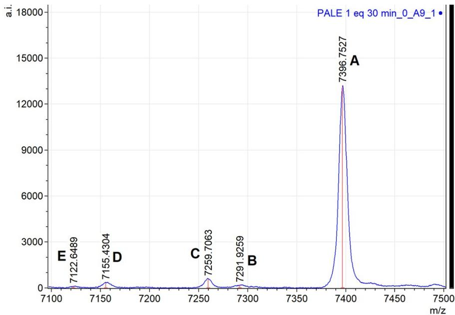
**Figure S2:** Positive ion MALDI-MS spectrum after mixing  $\text{Au}_{25}(\text{PET})_{18}$  with 1 eq. phenylacetylene in DCM for 30 minutes. The peaks are labelled as the following species: A)  $\text{Au}_{25}(\text{PET})_{18}$  B)  $\text{Au}_{25}(\text{PET})_{17}\text{S}_1$  C)  $\text{Au}_{25}(\text{PET})_{17}$  D)  $\text{Au}_{25}(\text{PET})_{16}\text{S}_1$  E)  $\text{Au}_{25}(\text{PET})_{16}$
