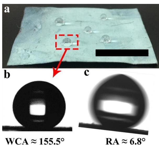
**Fig. S9** (a) Optical image of P25@PDMS@COM is shown, where water drop keep in sphere on the surface. (b-c) The average WCA and RA of 155.5° and 6.8° were respectively found on such surface. Scale bar: 1 cm.
