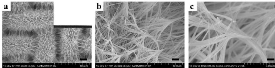
**Fig. S2** (a) SEM images of copper mesh after alkaline oxidation, (b) is the enlarged view of (a), (c) is the enlarged view of (b). The inset (a) is WCA of oxidized copper mesh. Scale bar: 20  $\mu\text{m}$  (a), 2  $\mu\text{m}$  (b), 0.6  $\mu\text{m}$  (c).
