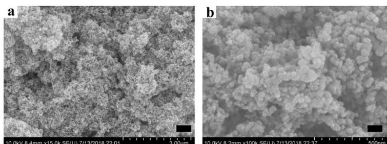
**Fig. S7** (a) SEM images of P25 NPs, (b) is the enlarged view of (a). Scale bar: 0.6  $\mu\text{m}$  (a), 200 nm (b).
