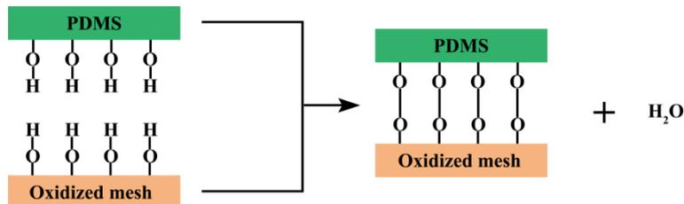
**Fig. S3** Hydroxyl group in PDMS was in full contact with copper hydroxide on such mesh to hydrolyze and form covalent bonds, so PDMS was introduced on the Cu mesh.
