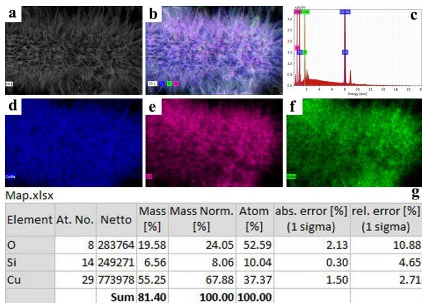
**Fig. S5** (a-f) EDS analysis on the PDMS-treated copper mesh. It showed Cu and Si were well distributed on the surface, introducing PDMS was grafted on copper mesh. (g) Elements content of O, Si, Cu were showed.
