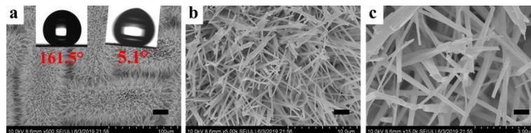
**Fig. S4** (a-c) SEM images of PDMS@COM, (b) is the enlarged view of (a), (c) is the enlarged view of (b). The inset (a) is WCA of 161.5° and RA of 5.1° on PDMS treated copper mesh. Scale bar: 20  $\mu\text{m}$  (a), 2  $\mu\text{m}$  (b), 0.6  $\mu\text{m}$  (c).
