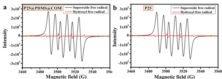
**Fig. S10** Superoxide free and hydroxyl free radicals were abundant on P25@PDMS@COM and fluorosilane-treated P25 NPs, which could decompose the organic matters.
