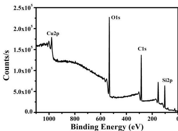
**Fig. S6** (a) XPS data of PDMS-treated copper mesh. Si2p appeared at the binding energy of 98.5 eV, also indicating PDMS was grafted on the surface.
