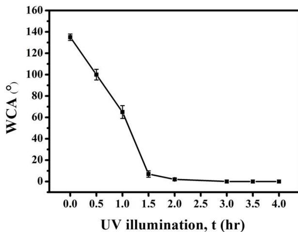
**Fig. S12** As for fluorosilane-treated P25 NPs, the high hydrophobicity would change into superhydrophilicity under UV irradiation.
