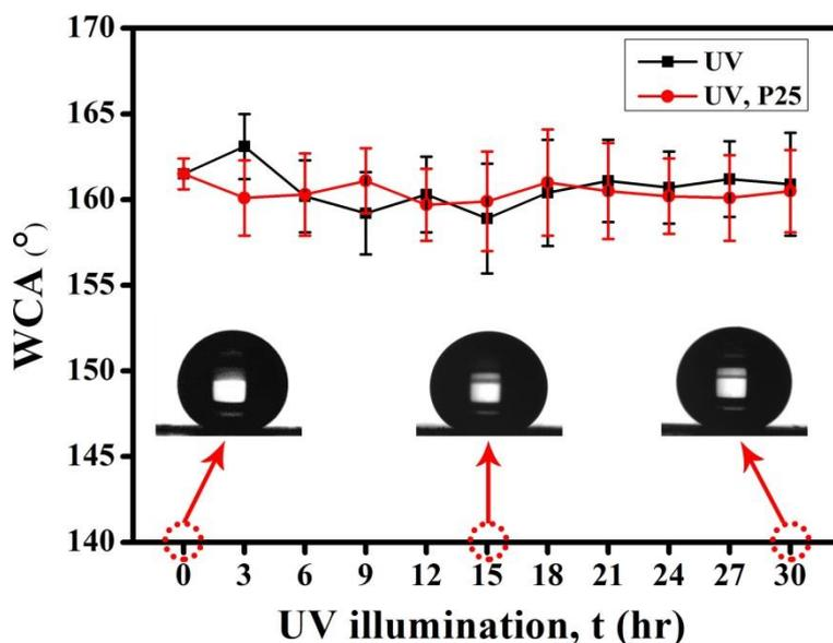
**Fig. S13** Under UV light, superhydrophobicity was still kept on PDMS@COM surface. In presence of P25 under UV light, PDMS@COM also showed stable superhydrophobicity.
