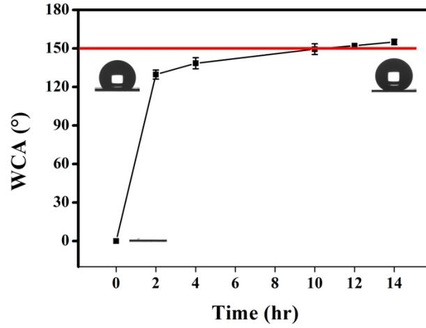
**Fig. S15** For O<sub>2</sub> plasma-treated surface, it showed superhydrophobicity with the WCA of nearly 0°. Upon the extending period, the WCA got larger and regained the WCA > 150° till to about 12 hr.
