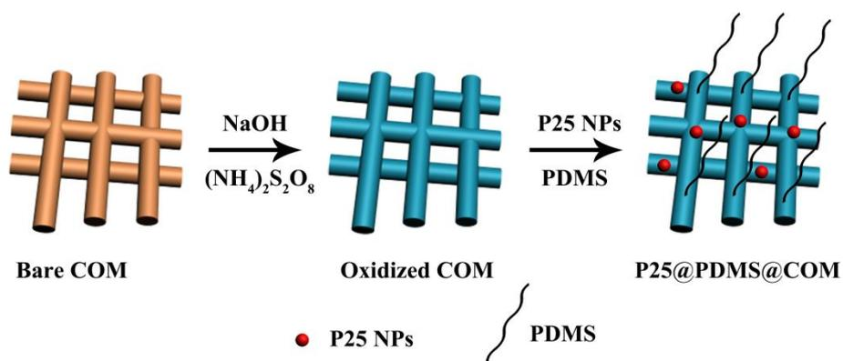
**Fig. S8** Schematic fabrication of P25@PDMS@COM.
