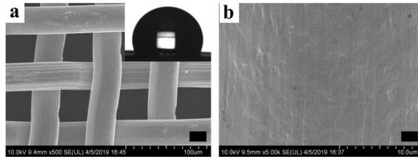
**Fig. S1** (a-b) SEM images of fresh copper mesh, (d) is the enlarged view of (c). The inset (a) is WCA of fresh mesh. Scale bar: 20  $\mu\text{m}$  (a), 2  $\mu\text{m}$  (b).
