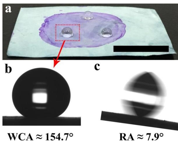
**Fig. S14** On Nile red contaminated area (a), superhydrophobicity was still kept with the average WCA and RA of 154.7° (b) and 7.9° (c). Scale bar: 1 cm.
