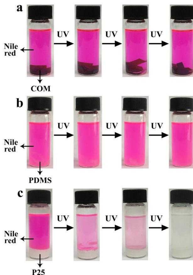
**Fig. S11** Nile red in ethanol was respectively placed in presence of 0.25 g of COM (a), PDMS (b), P25 (c) under UV illumination. The red dye could not be decomposed by COM and PDMS but P25.
