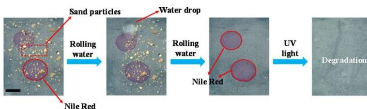
**Fig. S15** (a) On Nile red contaminated P25@PDMS@COM, sand particles still could be removed away from such surface by rolling water. Then, Under UV light, the red dyes was decomposed with no obvious color.
