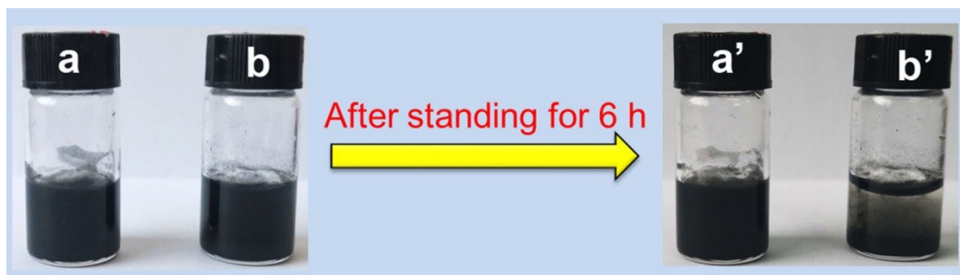
Figure S10. Digital photos of PMo 12 /PPy/CNT hybrid hydrogel (a and a') and conventional PMo 12 /PPy/CNT composite (b and b') after ultrasounding in water for 30 min (a and b) and continue standing for 6 h (a' and b')
