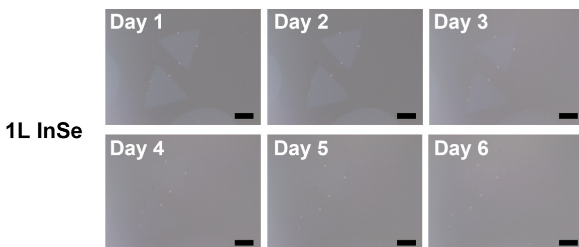
Figure S8. Sequence of OM images acquired at different times for monolayer InSe under ambient conditions. (Day n: after exposure to ambient conditions n days). Scale bar is 10 \mu\text{m} in length.
