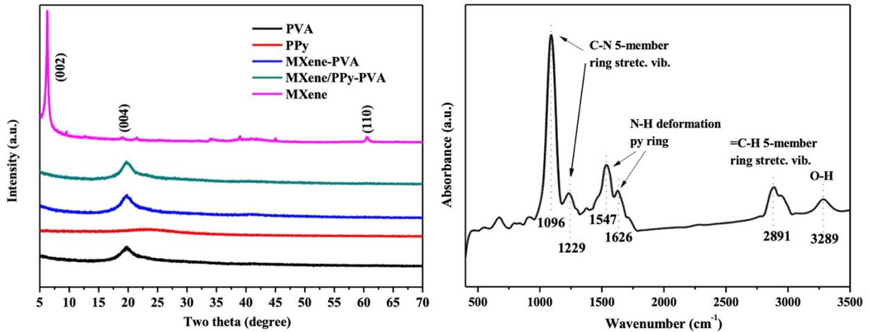
**Figure S2.** (a) XRD patterns of the PVA, PPy, MXene-PVA, MXene/PPy-PVA and MXene; (b) FTIR spectrum of the MXene/PPy-PVA hydrogel.
