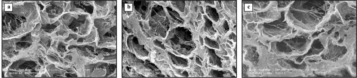
**Figure S1:** SEM images of MXene-PVA hydrogels with different MXene concentrations: (a)  $0.2 \text{ mg cm}^{-3}$ ; (b)  $0.4 \text{ mg cm}^{-3}$ ; and (c)  $2.0 \text{ mg cm}^{-3}$ .
