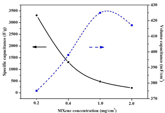
**Figure S7.** Specific capacitance and volume capacitance of MXene-PVA electrodes with different MXene concentration.
