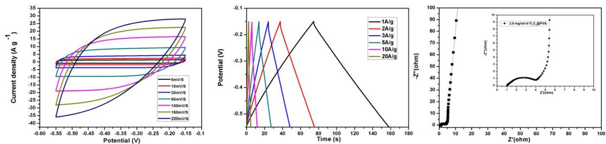
**Figure S6.** Electrochemical characterizations of 2 mg cm<sup>-3</sup> MXene hydrogel electrodes: (a) CV, (b) charge/ discharge, and (c) EIS curves.
