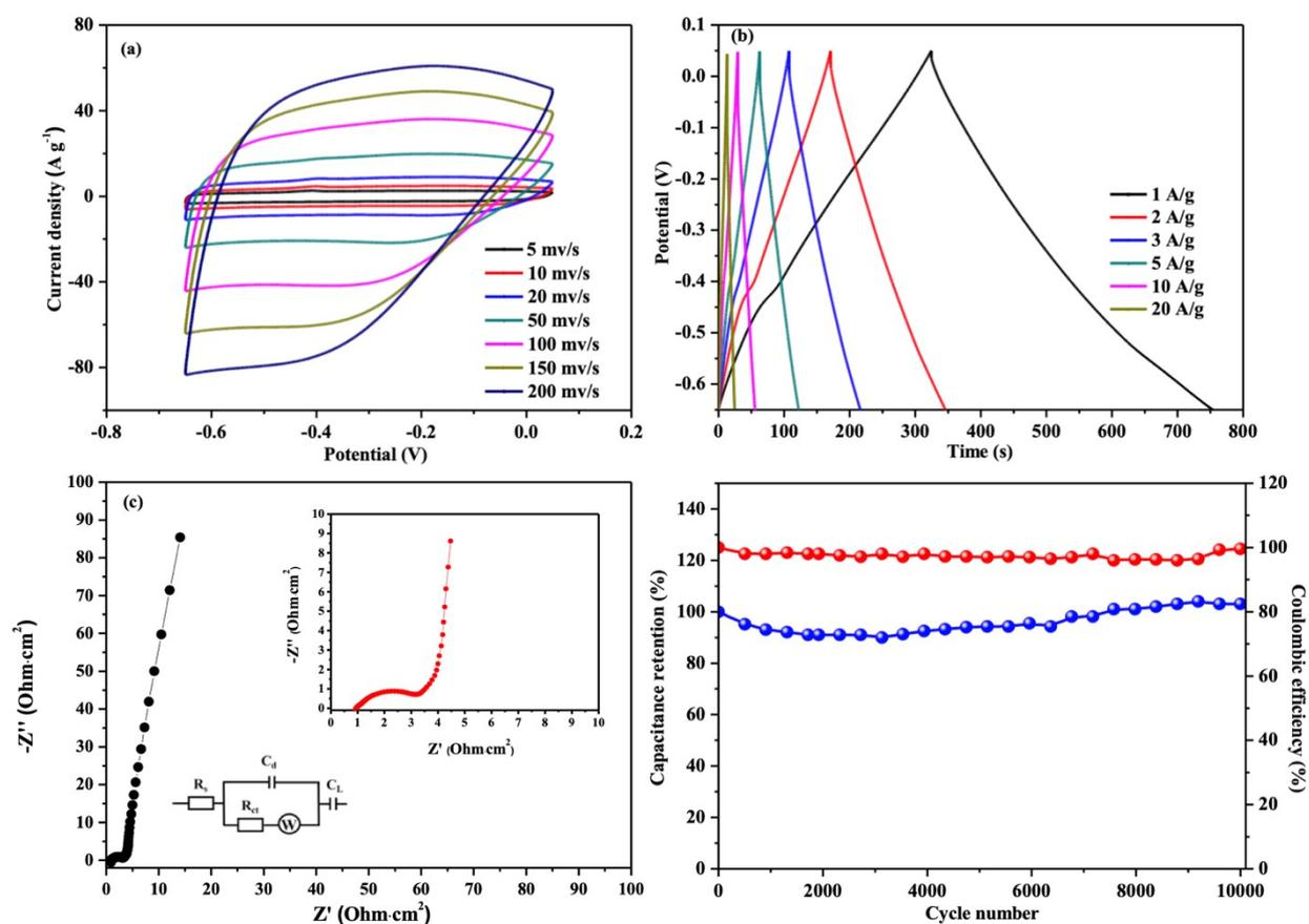
**Figure S8.** Electrochemical characterizations of MXene/PPy-PVA hydrogel electrodes: (a) CV, (b) charge/ discharge, (c) EIS curves, and (d) The cycle life and coulombic efficiency.
