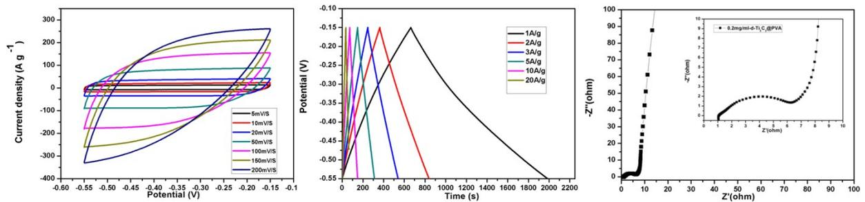
**Figure S4.** Electrochemical characterizations of 0.2 mg cm<sup>-3</sup> MXene hydrogel electrodes: (a) CV, (b) charge/ discharge, and (c) EIS curves.
