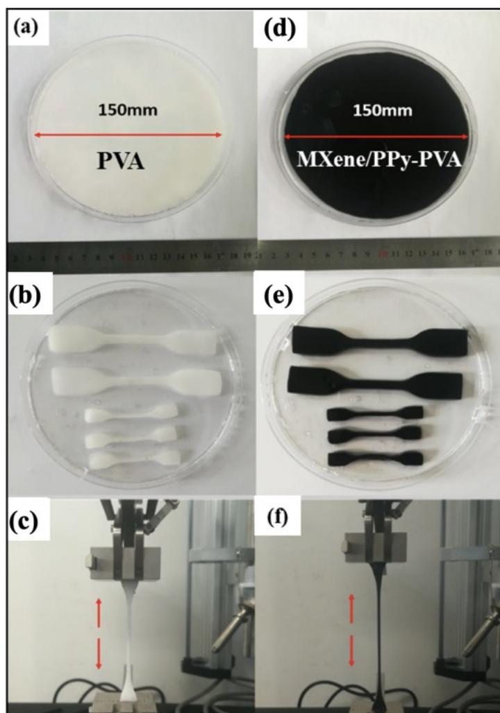
**Figure S10.** Photographs of PVA and MXene/PPy-PVA hydrogels during tensile tests: (a), (b) and (c) were PVA hydrogels; (d), (e) and (f) were MXene/PPy-PVA hydrogels.
