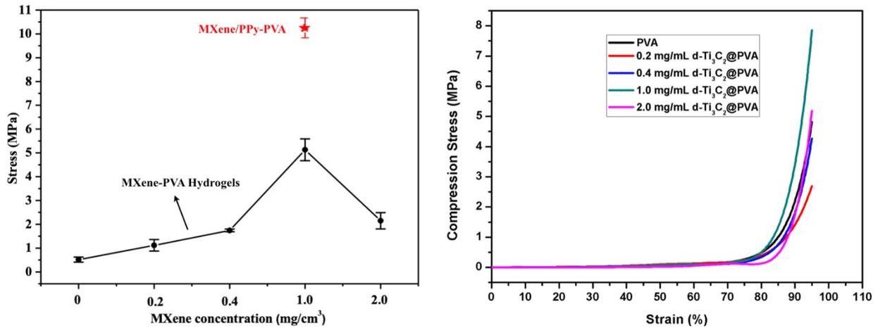
**Figure S3.** (a) The Maximum tensile stress of MXene-PVA hydrogels with different MXene concentrations, (b) Compression stress-strain curves of PVA and different concentration MXene-PVA hydrogels
