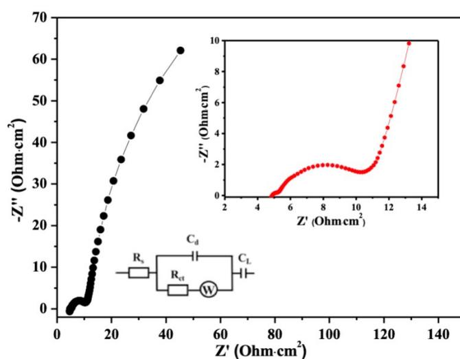
**Figure S9.** EIS curves of the assembled flexible supercapacitor.
