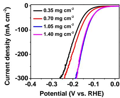
**Fig. S8** LSV polarization curves of MC-V-CoP in alkaline medium with different loading weight at the scan rate of 5 mV s<sup>-1</sup>.
