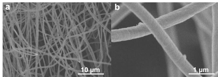
**Fig. S4** (a) low magnification and (b) high magnification SEM images of precursor nanofibers for NMC-V-CoP.
