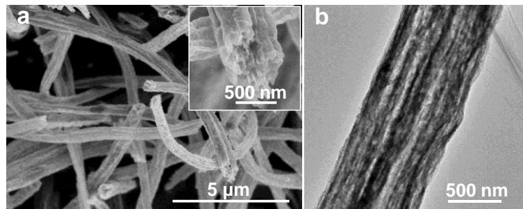
**Fig. S13** (a) SEM and TEM image of MC-V-CoP nanofiber fabricated by the weight ratio of PAN to PS as 2:3.
