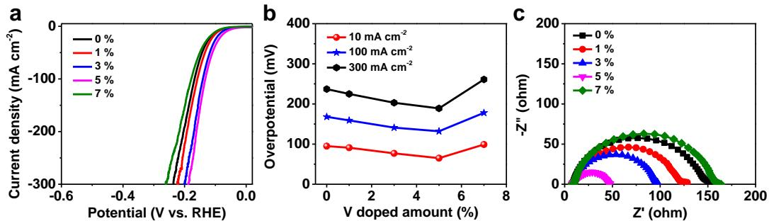
**Fig. S11** (a) LSV polarization curves, (b) overpotential at different current densities, and (c) EIS Nyquist plots of MC-CoP with different V doping amount.
