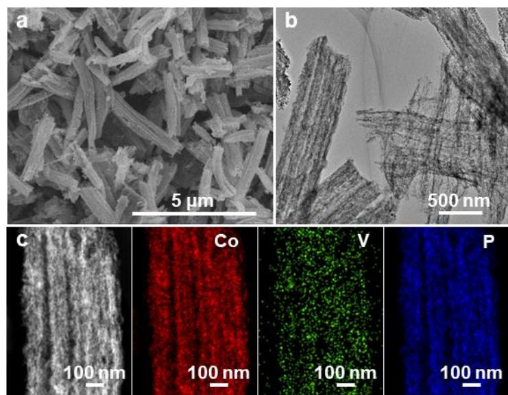
**Fig. S18** (a) SEM image, (b) TEM image and (c) element mapping of MC-V-CoP nanofiber after cycling stability test in neutral medium.
