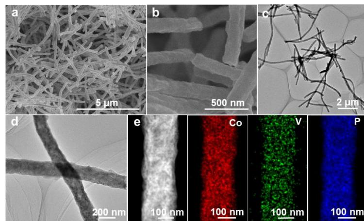
**Fig. S5** (a) low magnification and (b) high magnification SEM images of NMC-V-CoP nanofiber, (c) low magnification and (d) high magnification TEM images of MC-V-CoP nanofiber, (e) element mapping of MC-V-CoP nanofiber.
