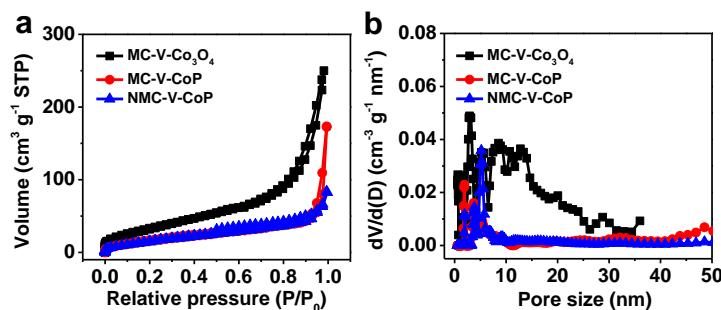
**Fig. S6** (a) N<sub>2</sub> adsorption-desorption curves and (b) corresponding pore size distribution of MC-V-Co<sub>3</sub>O<sub>4</sub>, MC-V-CoP and NMC-V-CoP.
