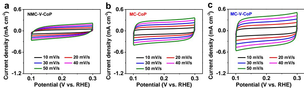
**Fig. S15** CV curves of NMC-V-CoP, MC-CoP and MC-V-CoP in neutral medium with different scan rates.
