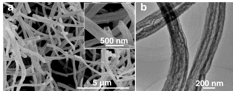
**Fig. S12** (a) SEM and TEM image of MC-V-CoP nanofiber fabricated by the weight ratio of PAN to PS as 2:1.
