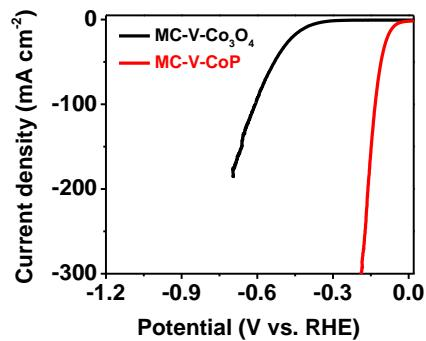
**Fig. S9** LSV polarization curves of MC-V-Co<sub>3</sub>O<sub>4</sub> and MC-V-CoP in alkaline medium at the scan rate of 5 mV s<sup>-1</sup>.
