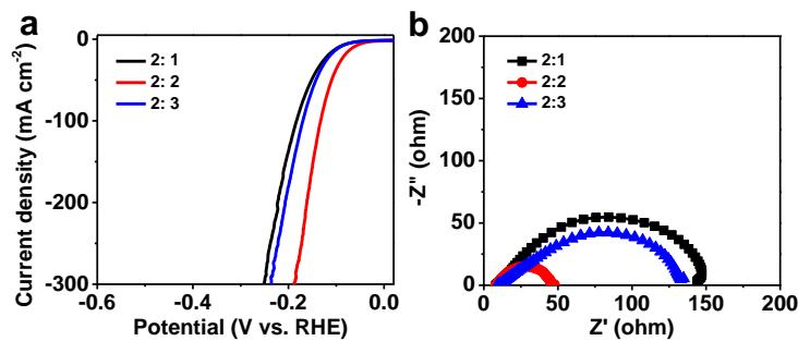
**Fig. S14** (a) LSV polarization curves and (b) EIS Nyquist plots of MC-V-CoP nanofiber fabricated by different addition ratio of PA N and PS.
