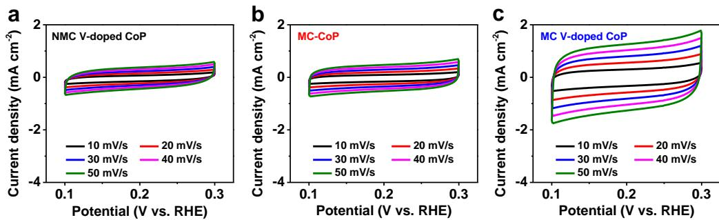
**Fig. S10** CV curves of NMC-V-CoP, MC-CoP and MC-V-CoP in alkaline medium with different scan rates.
