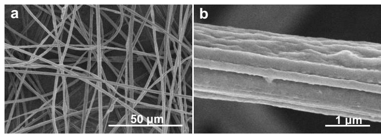
**Fig. S1** (a) low magnification and (b) high magnification SEM images for precursor fiber of MC-V-CoP.
