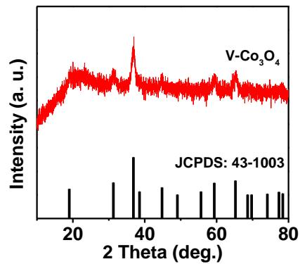
**Fig. S2** XRD patterns of V doped  $\text{Co}_3\text{O}_4$
