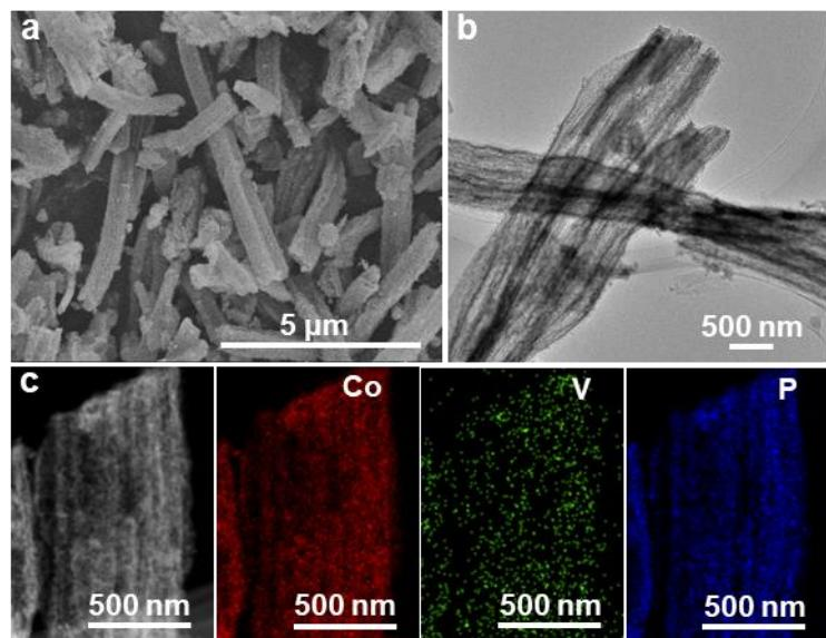
**Fig. S17** (a) SEM image, (b) TEM image and (c) element mapping of MC-V-CoP nanofiber after cycling stability test in alkaline medium.
