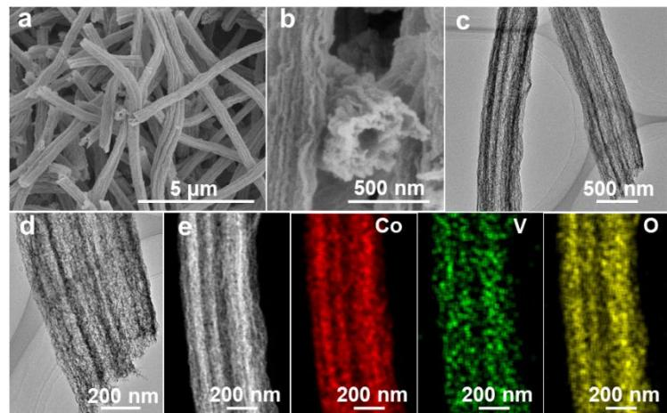
**Fig. S3** (a) low magnification and (b) high magnification SEM images of MC-V- $\text{Co}_3\text{O}_4$  nanofiber, (c) low magnification and (d) high magnification TEM images of MC-V- $\text{Co}_3\text{O}_4$  nanofiber, (e) element mapping of MC-V- $\text{Co}_3\text{O}_4$  nanofiber.
