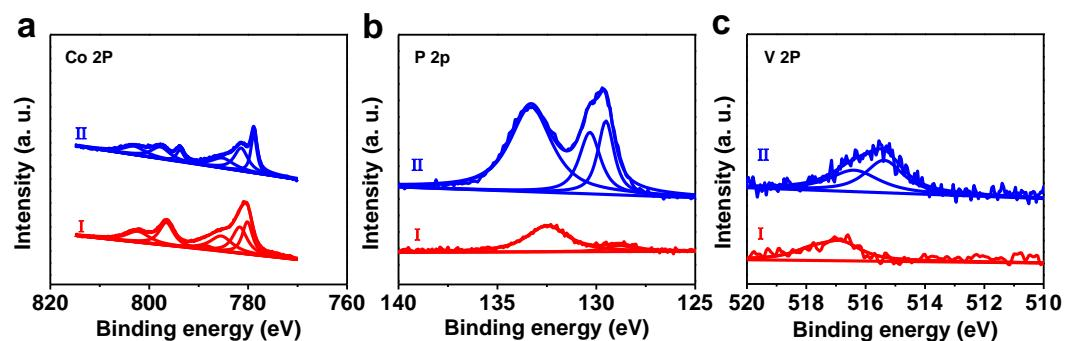
**Fig. S19** High-resolution XPS spectrum of MC-V-CoP after long-term test in (I) alkaline and (II) neutral medium, (a) Co 2p, (b) P 2p, (c) V 2p.
