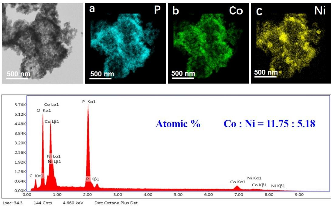
**Figure S5.** TEM image and EDS elemental mapping of Ni-Co-P HNCs.
