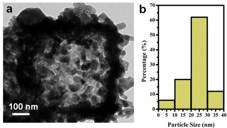
**Figure S7.** (a)TEM image and (b) coral-horned nanoparticle size statistics of N-Ni-Co-P HNCs.
