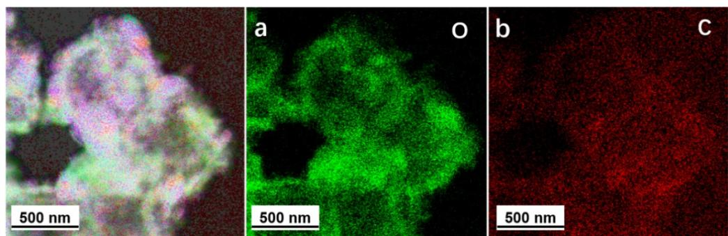
**Figure S8.** EDX elemental mapping for (a) O, (b) C of N-Ni-Co-P HNCs, corresponding to Figure 3g in the text.
