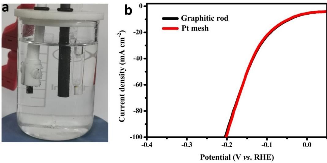
**Figure S13.** (a) Optical photo showing three-electrode test system (graphite rod as the electrode counter), (b) Catalytic performance of N-Ni-Co-P HNCs using a graphitic rod or a Pt mesh as the counter electrode in 1.0 M KOH, respectively.
