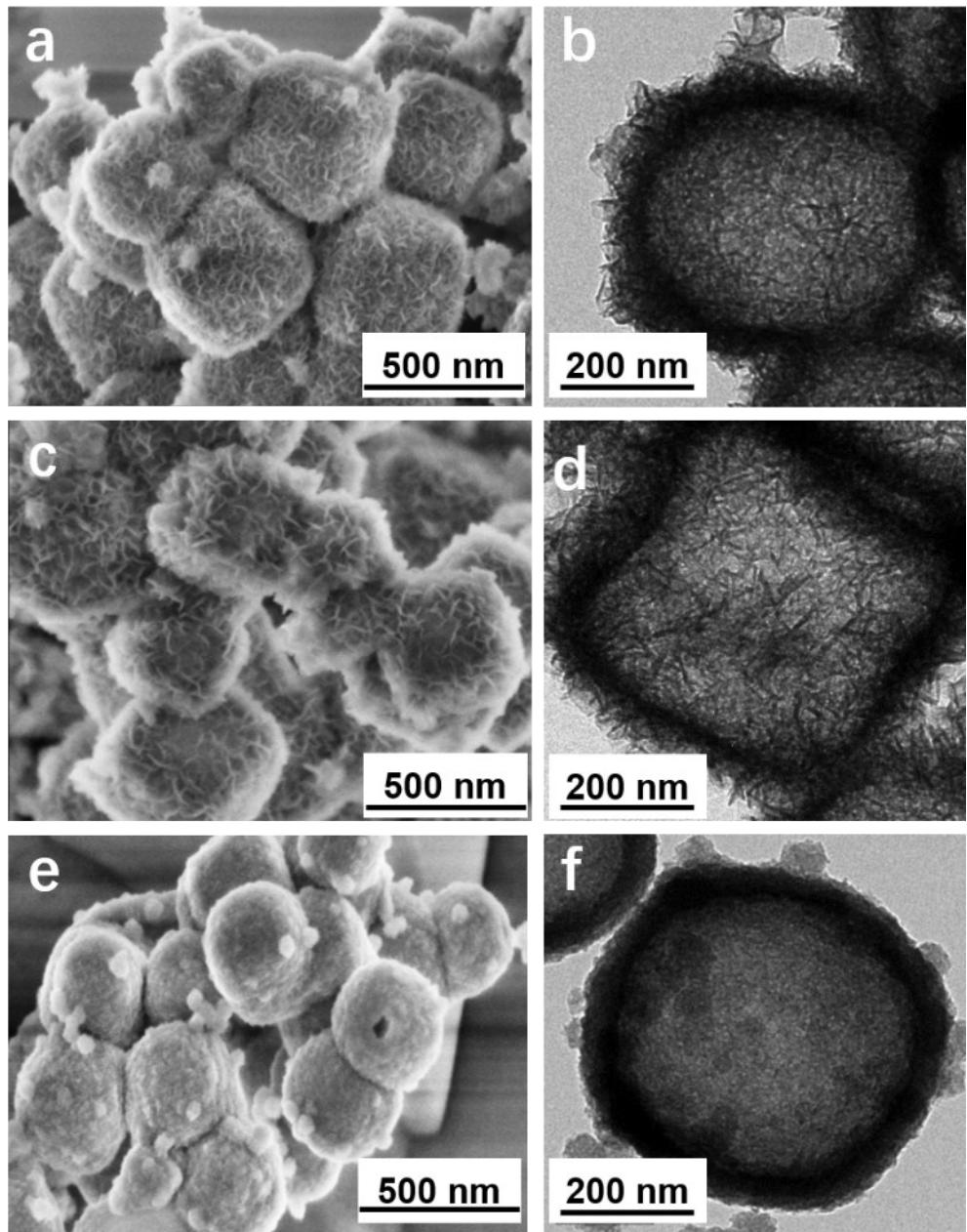
**Figure S2.** SEM and TEM images of Ni-Co LDHs with different molar ratio of Ni:Co ( a, b)1:1, (c, d) 1:3 and (e, f) 3:1.
