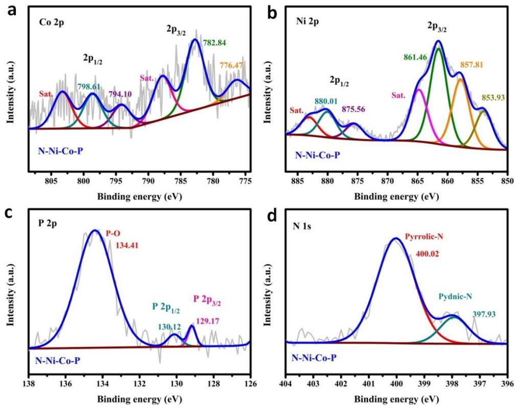
**Figure S12.** XPS spectra of (a) Co 2p, (b) Ni 2p, (c) P 2p and (d) N 1s of N-Ni-Co-P HNCs after the HER durability test.
