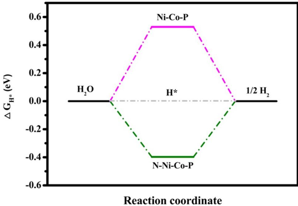
**Figure S20.** The calculated HER free-energy diagram (FED) on N-Ni-Co-P (001) and Ni-Co-P (001) surface.
