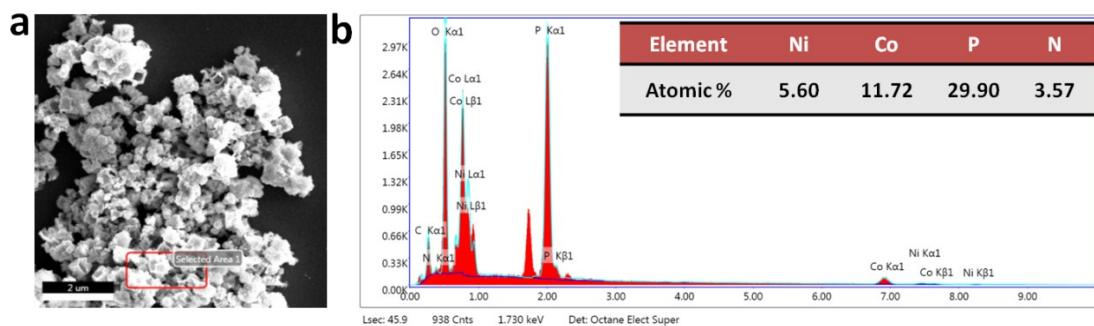
**Figure S6.** (a) SEM image and (b) EDS N-Ni-Co-P HNCs.
