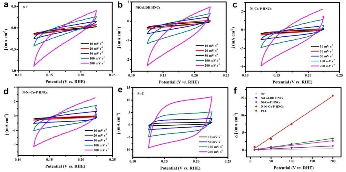
**Figure S14.** The electrochemical double-layer capacitance ( $C_{\text{dl}}$ ) measurements with different scanning rates of 10, 20, 50, 100 and 200  $\text{mV s}^{-1}$  for (a) bare NF, (b) Ni-Co LDH HNCs, (c) Ni-Co-P HNCs (d) N-Ni-Co-P HNCs, (e) Pt-C, (f) The Double-layer capacity currents vs. scan rates of the as-prepared samples.
