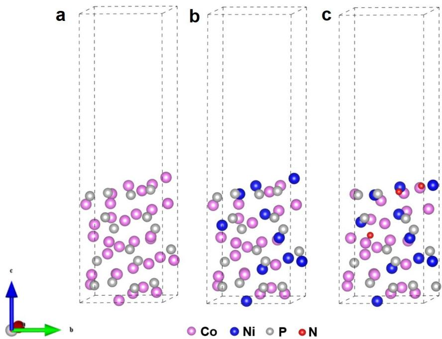
**Figure S18.** The crystal models of (a)  $\text{Co}_2\text{P}$ , (b) Ni-Co-P and (c) N-Ni-Co-P.
