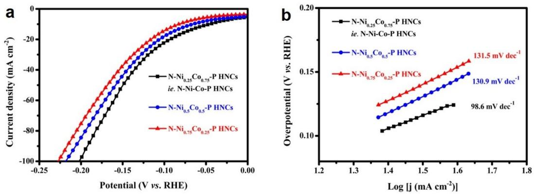
**Figure S10.** (a) The LSV curves of catalysts with different Ni/Co ratios, (b) The calculated Tafel slopes of the catalysts.
