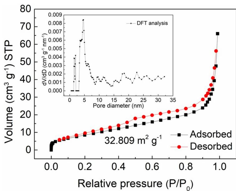
**Fig. S3** (a) N<sub>2</sub> adsorption-desorption isotherm of CoSe@FeSe<sub>2</sub>. (b) The corresponding pore distribution curve.
