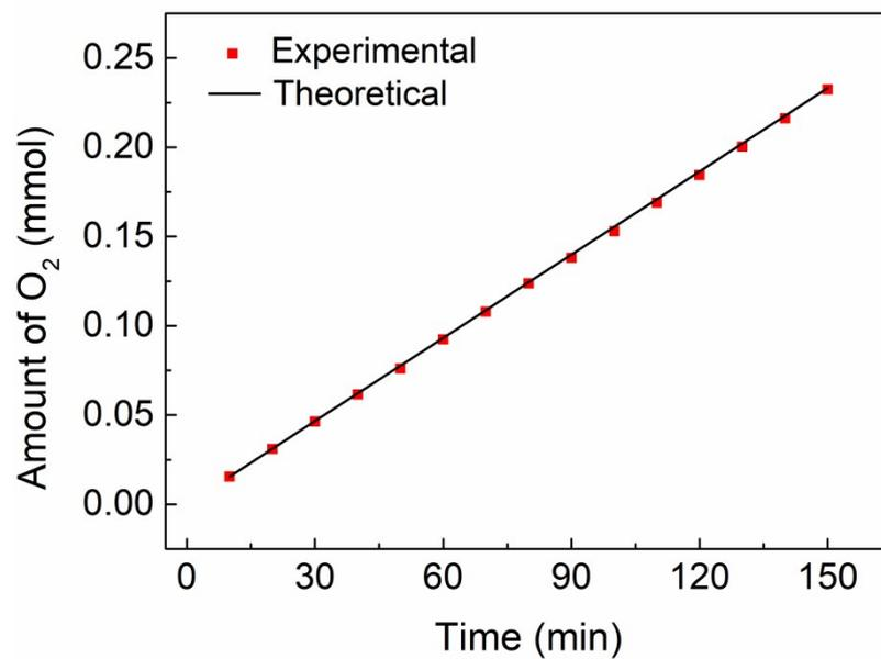
**Fig. S8** The amount of generated O<sub>2</sub> gas for CoSe@FeSe<sub>2</sub> in 150 min.
