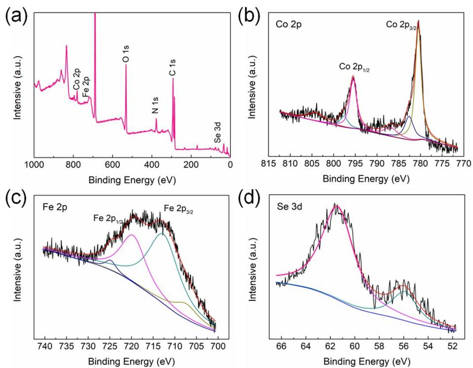
**Fig. S9** XPS spectra of CoSe@FeSe<sub>2</sub> after 12h durability test towards OER: (a) survey scan, (b) Co 2p, (c) Fe 2p and (d) Se 3d.
