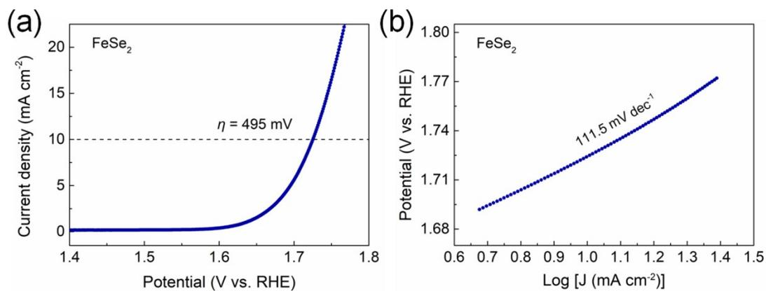
**Fig. S5** (a) Polarization curves with *i*R compensation and (b) Tafel slope curves of FeSe<sub>2</sub>.
