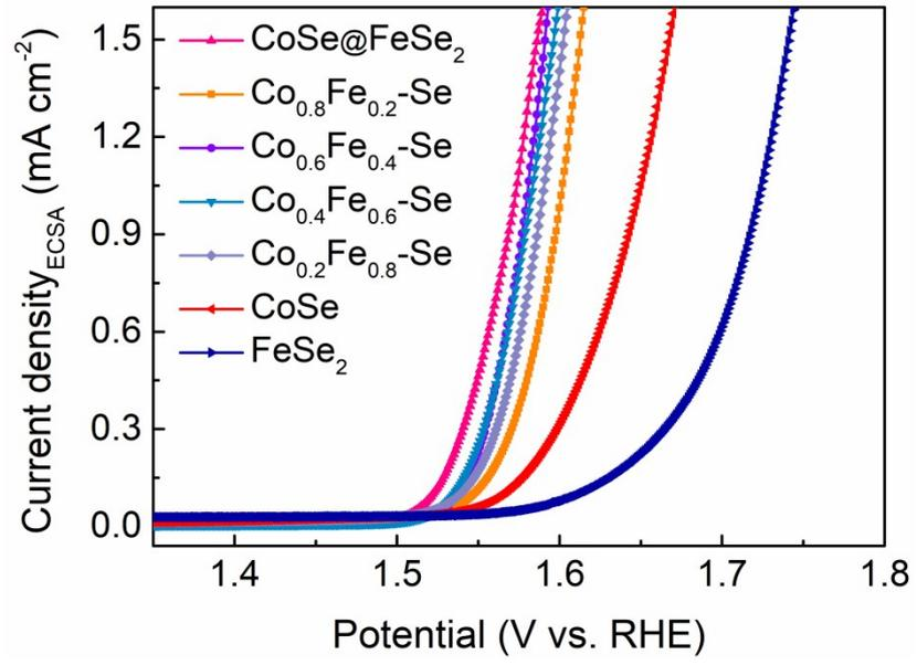
**Fig. S7** The OER polarization curves normalized to the ECSA.
