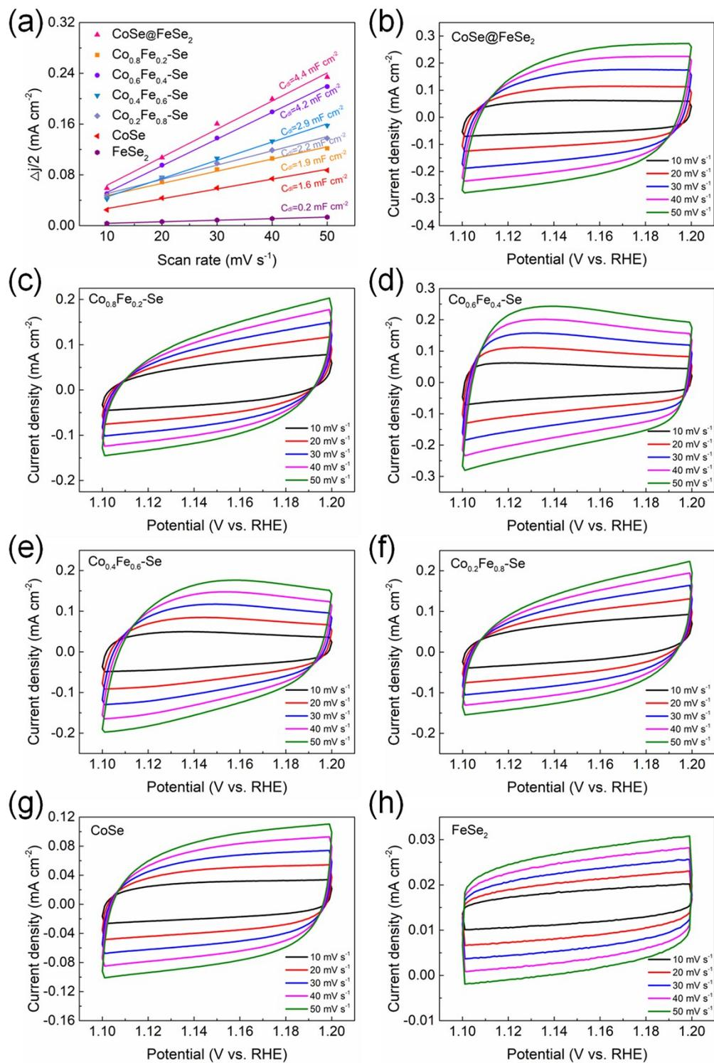
**Fig. S6** (a) Plots of current density vs. scan rate (at 1.15 V). (b-h) CV curves of Co-Fe selenides with different metal atomic ratios (1:1, 4:1, 3:2, 2:3, 1:4, 1:0 and 0:1) in the potential range of 1.1-1.2 V vs. RHE.
