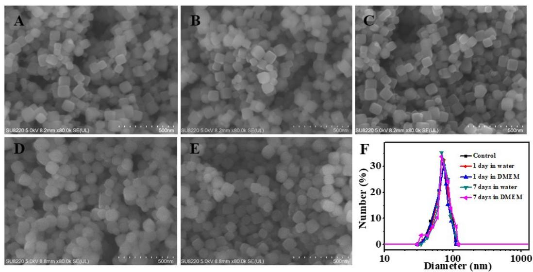
**Fig. S1.** SEM images (A-E) and hydrodynamic diameter (F) of RhB@ZIF-8 after dispersion in aqueous solution (B, D) and cell culture medium (C, E) for one and seven days, respectively.
