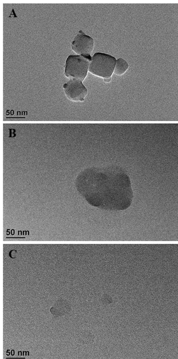
**Fig. S2.** TEM images of RhB@ZIF-8 before (A) and after (B, C) ATP treatment. RhB@ZIF-8 ( $0.1 \text{ mg}\cdot\text{mL}^{-1}$ ) was incubated with  $0.6 \text{ mM}$  (B) and  $6 \text{ mM}$  (C) ATP for 3 min, respectively.
