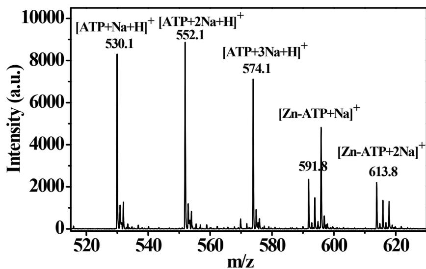
**Fig. S3.** Positive ion MALDI-TOF mass spectrum of reaction products of ATP and ZIF-8.
