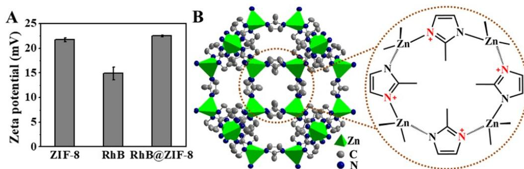
**Fig. S9.** (A) Zeta potential of free ZIF-8, RhB, and RhB@ZIF-8 in H<sub>2</sub>O. (B) A unit framework and local molecular structure of ZIF-8.
