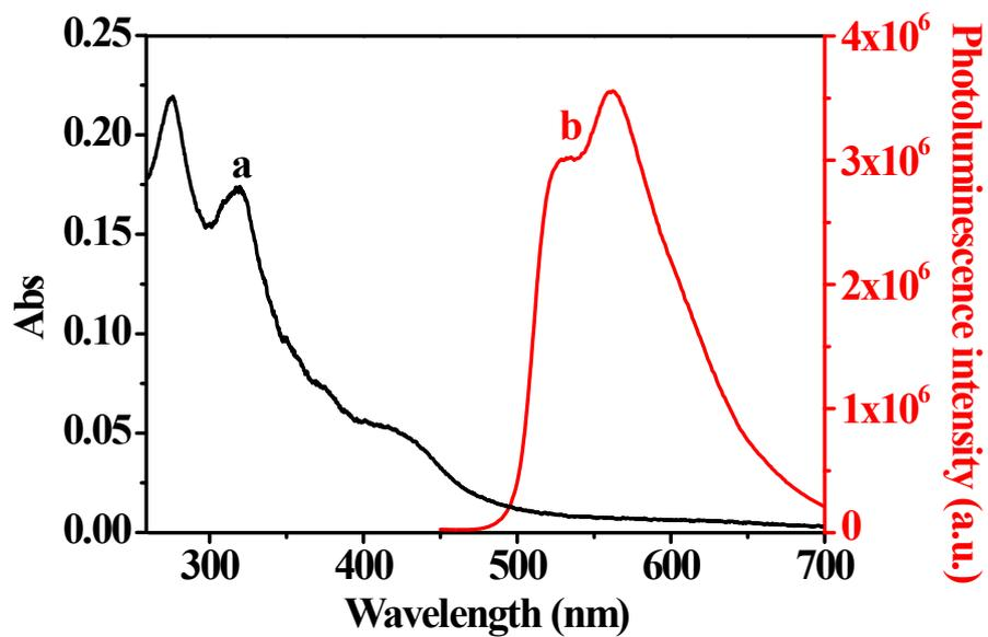
**Fig. S14.** UV-Vis absorption spectrum (a) and photoluminescence spectrum (b) of PS-Ir (6  $\mu$ M) in 25 mM PBS (pH 7.4),  $\lambda_{\text{ex}} = 320$  nm.
