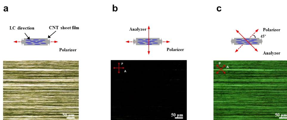
**Figure S6.** Polarized optical microscopy measurement to evaluate LC alignment: LC-coated P-ECS film ( $n = 5$ ) with (a) one polarizer (parallel direction, bright state), (b) crossed polarizer-analyzer (dark state), and (c)  $45^\circ$  tilted polarizer-analyzer (medium bright state).
