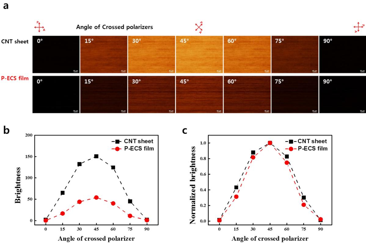
**Figure S2.** (a) Polarized optical microscopy image of CNT sheet and polymer-embedded CNT sheet (P-ECS) film under the crossed polarizer (polarizer-analyzer) with a step of  $15^\circ$  from  $0$  to  $90^\circ$ . The number of CNT layers is 10. (b) Relative brightness and (c) normalized brightness of CNT sheet and P-ECS film. The relative brightness is calculated by an image analysis software.
