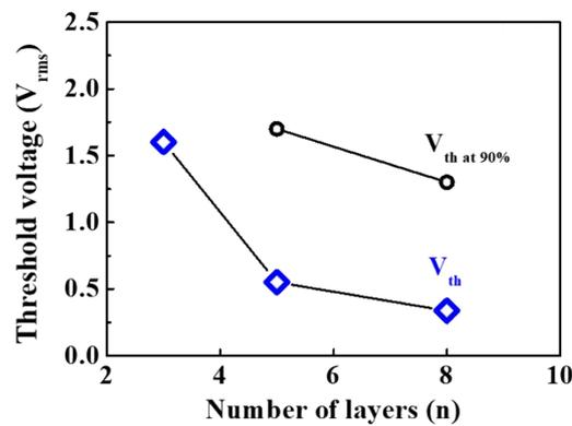
**Figure S9.** Threshold voltage ( $V_{th}$ , blue open rhombus symbols) and  $V_{th}$  at 90% of normalized intensity (black open circle symbols).
