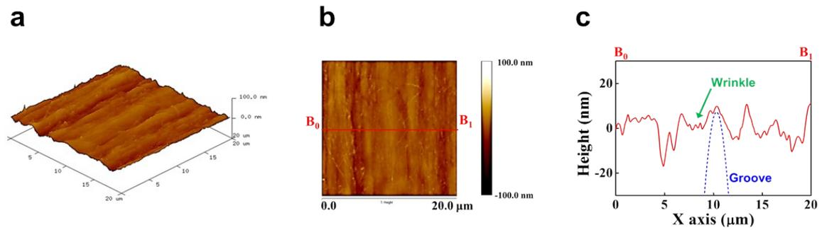
**Figure S4.** AFM imaging of the surface of P-ECS film ( $n = 5$ ): (a) 3D image, (b) 2D height morphology, and (c) line profile corresponding to the red line in (b).
