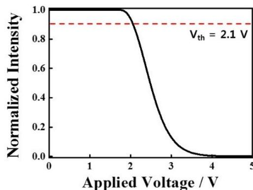
**Figure S10.** Simulation results of voltage-dependent transmittance of standard cell (ITO/Polyamide).
