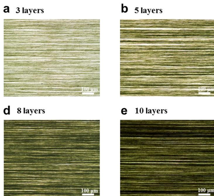
**Figure S5.** Optical microscopy images of P-ECS films with different number of CNT layers.
