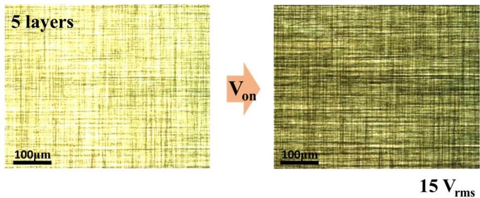
**Figure S11.** Optical microscopy images of the LC cell device ( $n = 5$ ) in voltage-off and -on states ( $15 V_{rms}$ ).
