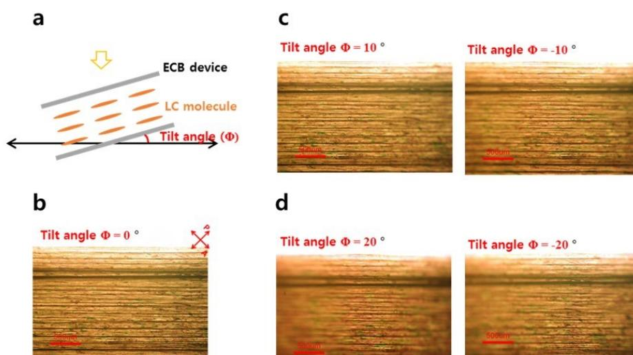
**Figure S7.** Polarized optical microscopy (POM) measurement of cell device under tilt angle ( $\Phi$ ) with  $45^\circ$  tilted polarizer-analyzer: (a) Schematic of the cell device consisting of two parallel aligned P-ECS film. The LC molecules are injected into the gap ( $5 \mu\text{m}$ ). POM image at (b)  $\Phi = 0^\circ$ , (c)  $\Phi = \pm 10^\circ$ , and (d)  $\Phi = \pm 20^\circ$ .
