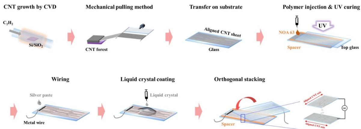
**Figure S12.** Schematics showing the steps in the fabrication of a LC cell device (one drop filling method).
