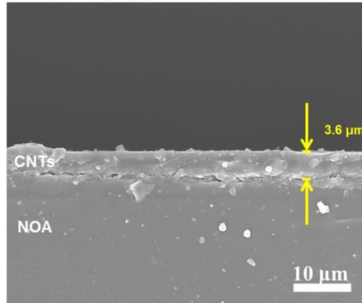
**Figure S3.** SEM image of the cross-section of polymer embedded CNT sheet film.
