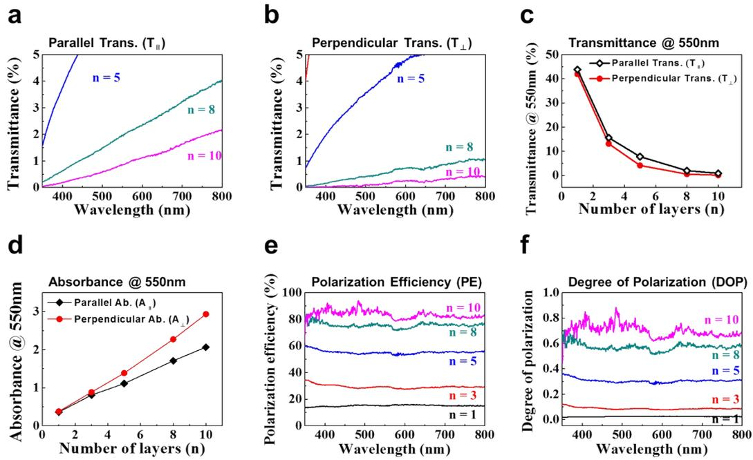
**Figure S8.** Optical anisotropy performance of two overlapped P-ECS films with various numbers of CNT layers: (a) parallel transmittance, (b) perpendicular transmittance, (c) transmittance at  $\lambda = 550$  nm as a function of CNT layers, (d) absorbance at  $\lambda = 550$  nm as a function of CNT layers. (e) Polarization efficiency and (f) degree of polarization.  $n$  is the number of CNT layers.
