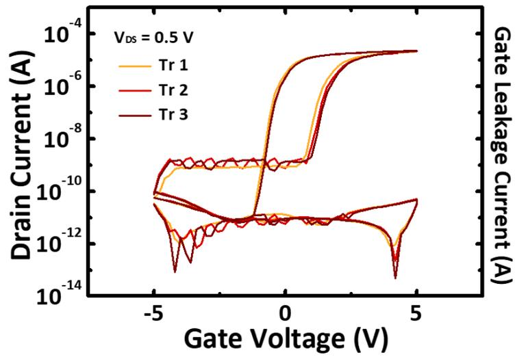
**Fig. S5.** Variations in  $I_{DS}$ - $V_{GS}$  transfer characteristics and gate leakage currents of three transistors located in the same column sharing the same S/D lines. The devices exhibited almost the same operations including ferroelectric memory windows without marked variations.
