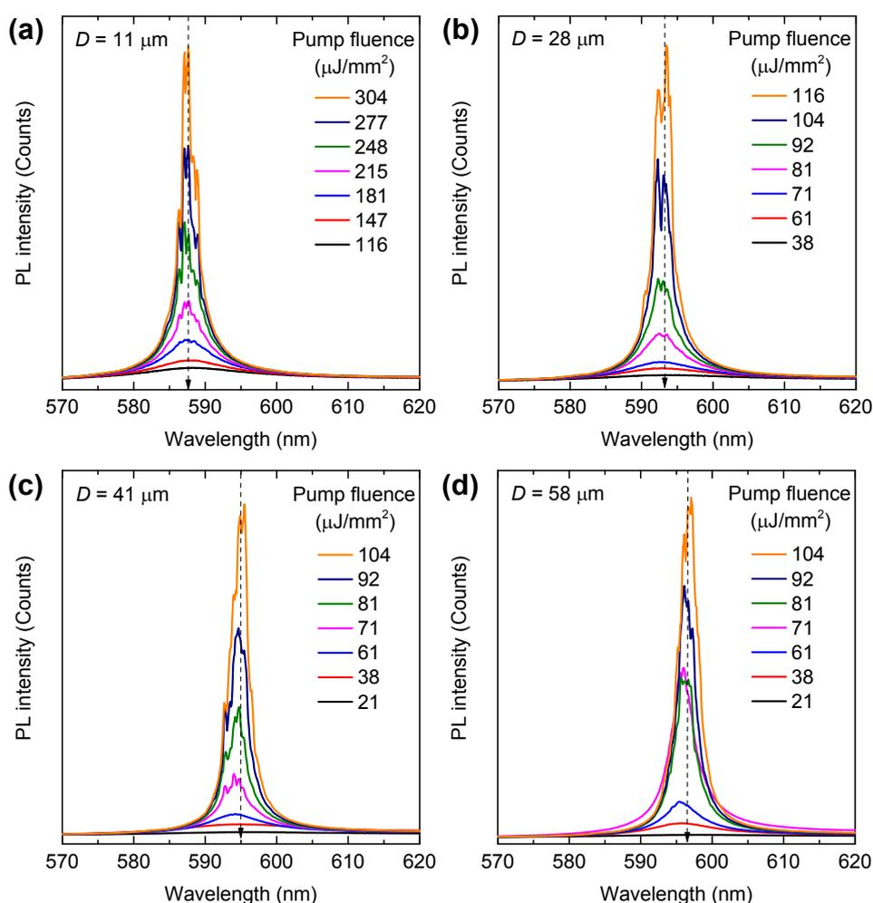
**Fig. S4.** Emission spectra of four different fibers under various pump pulse fluences. The dashed line denotes the center of the lasing spectrum.
