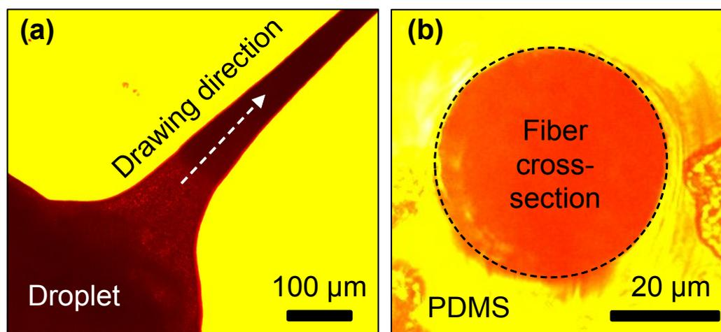
**Fig. S1.** Optical microscope image of (a) a direct drawing microporous fiber from a droplet and (b) a fiber's cross-section.
