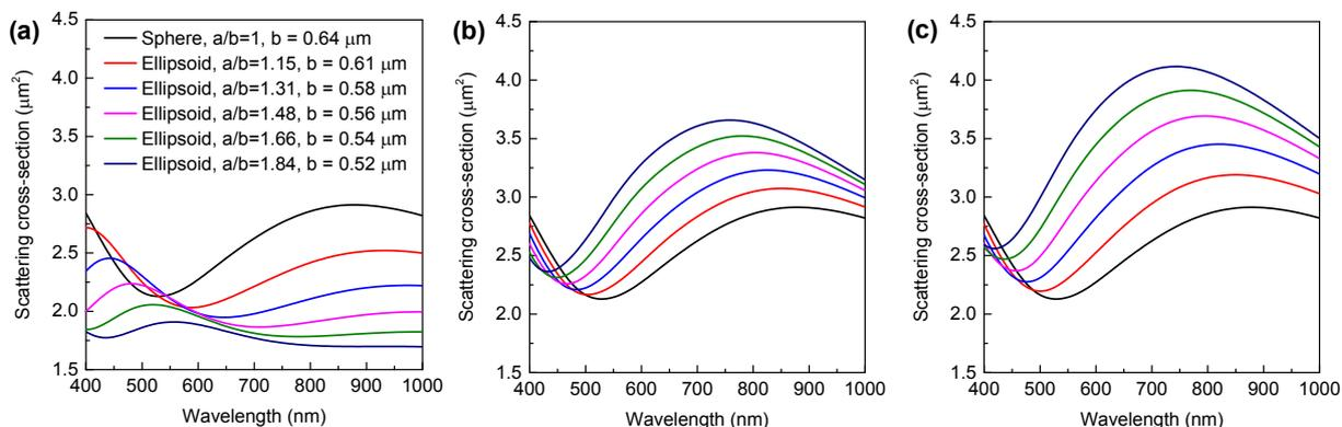
**Fig. S7.** Scattering cross-section of a single ellipsoid air void in polymer, considering all three different orientations concerning the incident plane wave. The plane wave is propagating: (a) parallel to the stretched direction and in (b), (c) transverse to the stretched pore.
