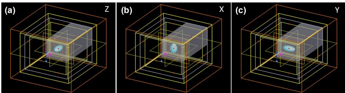
**Fig. S6.** Simulation geometry for calculating scattering cross-section of a single ellipsoid air void in polymer, considering all three different orientations with respect to the incident plane wave. The plane wave is propagating parallel to (a) the stretched direction and (b), (c) in transverse to the stretched pore. The incident light is polarized and the polarized direction is vertically shown by blue arrows.
