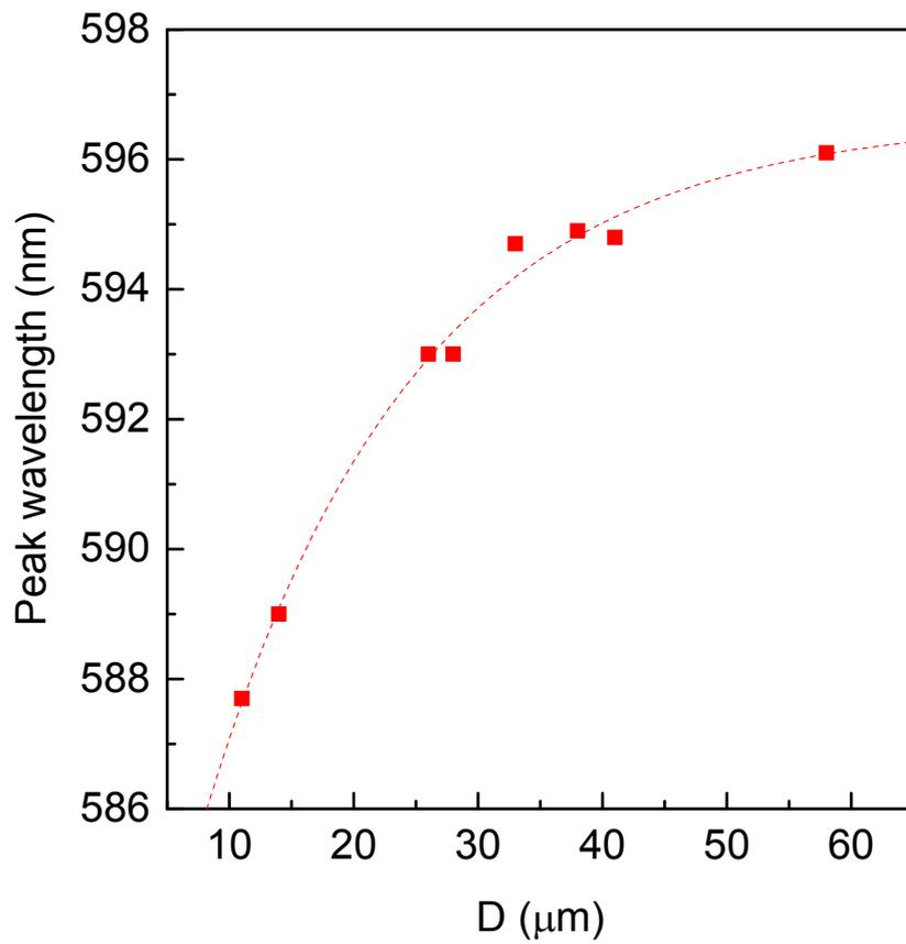
**Fig. S5.** Peak wavelength as a function of fiber diameter.
