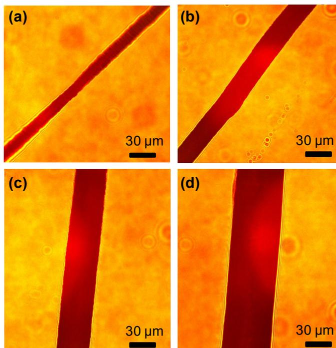
**Fig. S2.** Optical microscope images of different microporous PVA fibers. (a)-(d) Diameter of the fibers are around 14, 26, 38, 58  $\mu\text{m}$ , respectively.
