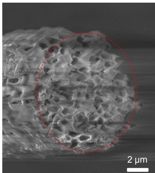
**Fig. S3.** SEM image of the cross-section of a microporous PVA fiber
