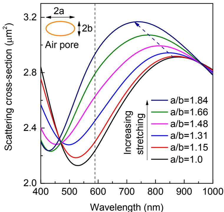
**Fig. S8.** Average scattering cross-section of air pore with various deformations in a polymer medium versus wavelength. The dashed line highlights the wavelength of 590 nm.
