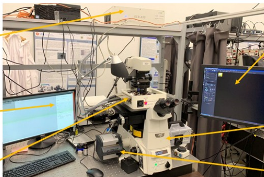
Figure S2. Overview of the magnetic field generator and fluorescence microscopy imaging system.
