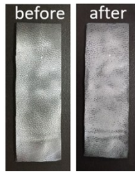
Fig. S2 Photograph of leather coating surface before and after 140 cycles of abrasion in the sandpaper abrasion test.
