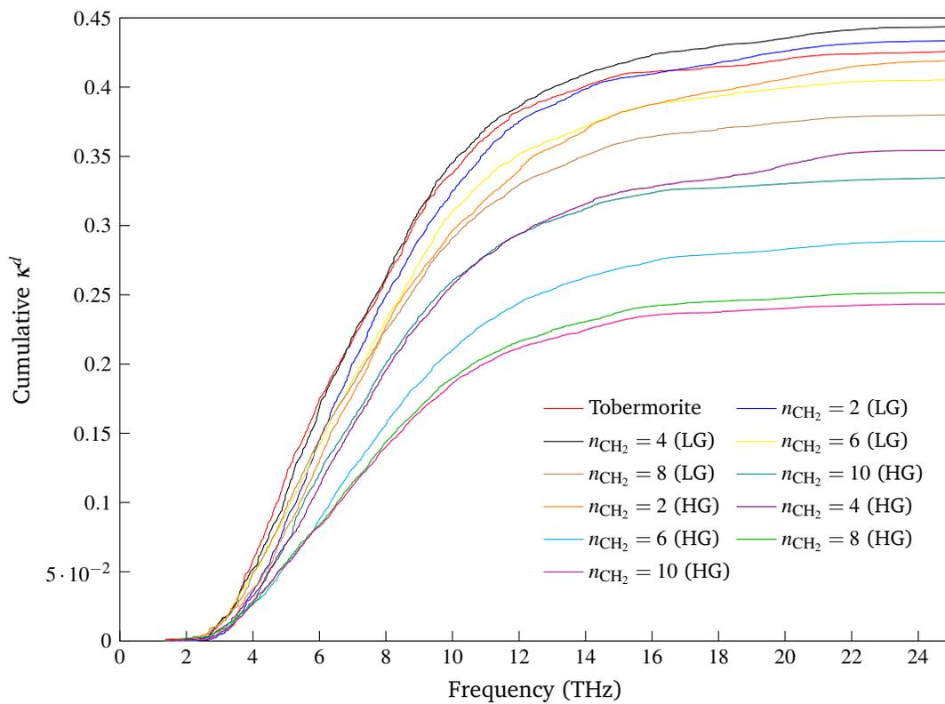
Fig. 2 S Cumulative diffusive contribution to the thermal conductivity. For small chain length and low grafting percentage, we do not observe a significant change in  $\kappa^d$  compared to the pristine TB. The reduction is most significant for large chain lengths and high grafting percentages.
