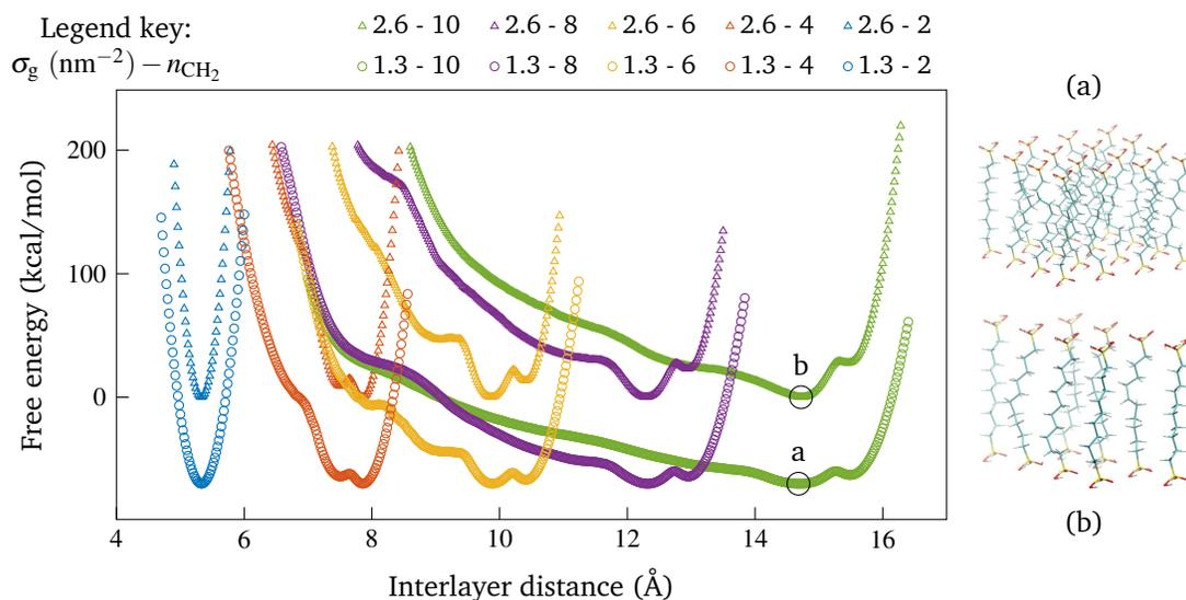
Fig. 1 S PMF computed for polymer chain groups as displayed in schematics on the right. Except the case with the smallest chain length, multiple minima are observed for PMF.
