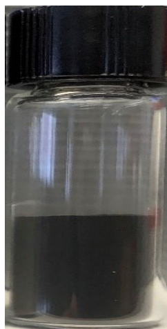
Figure S3. Illustration of tape density measurement of 2.5 g LTSO/C in a 4 ml glass vial.
