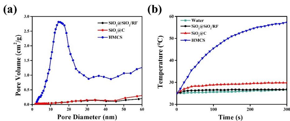
**Fig. S3.** (a) Nitrogen adsorption-desorption isotherms of pore volume distribution curves and (b) photothermal effects of SiO<sub>2</sub>@SiO<sub>2</sub>/RF, SiO<sub>2</sub>@C and HMCS.
