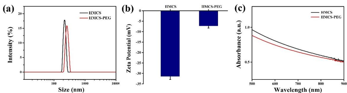
**Fig. S2.** (a) DLS diagram, (b)  $\zeta$ -potential data and (c) UV absorption of HMCS before and after PEG modification.
