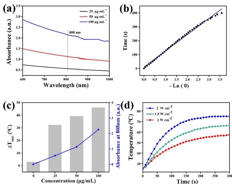
**Fig. S5.** (a) The UV absorbance of HMCS-PEG with different concentration, (b) linear relationship of time versus  $-\ln\theta$  obtained from the cooling periods, (c) a summary of the maximum temperature change of the nanoparticle suspensions during laser exposure, together with their relative absorbance at 808 nm, (d) photothermal performance of HMCS-PEG dispersion irradiated with different power densities.
