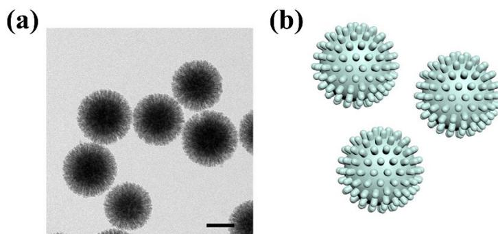
**Fig. S1.** (a) TEM image of SiO<sub>2</sub> template with solid core and radial spines, (b) 3D model of SiO<sub>2</sub> template. The scale bar is 100 nm.
