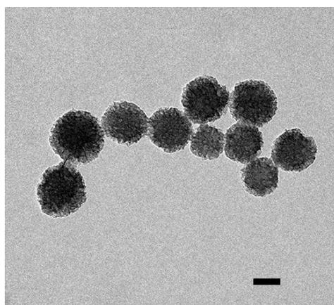
**Fig. S6.** TEM images of HMCS-PEG-GA. The scale bar is 100 nm.
