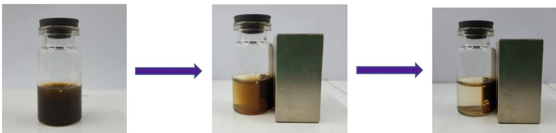
Figure S10. Images of a dispersion of MNG (1.6 mg / mL) exposed to a magnetic field at different times 0, 30 and 60 s.
