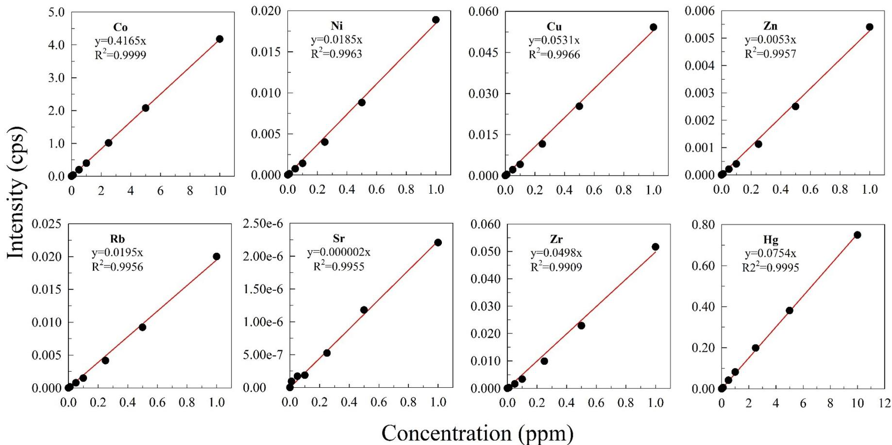
Figure S2. Calibration curves for individual elements (Co, Ni, Cu, Zn, Rb, Sr, Zr, Hg) measured by ICP-MS with solution-based calibration (standard additions mode).
