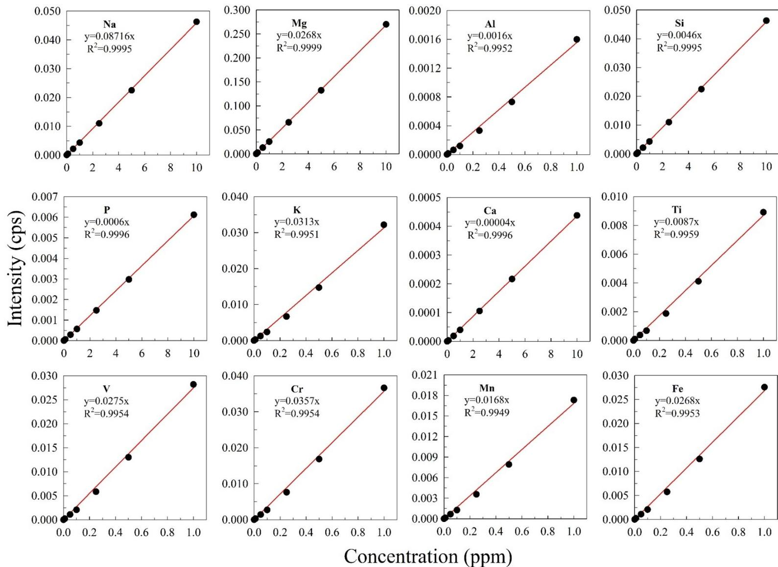
Figure S1. Calibration curves for individual elements (Na, Mg, Al, Si, P, K, Ca, Ti, V, Cr, Mn, Fe) measured by ICP-MS with solution-based calibration (standard additions mode).
