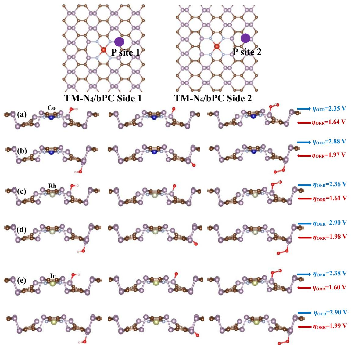
**Figure S9** Geometric structure of ORR/OER species ( $\text{OH}^*$ ,  $\text{O}^*$  and  $\text{OOH}^*$ ) adsorbed on (a) P side of Co-N<sub>4</sub>/bPC (side 1), (b) P side of Co-N<sub>4</sub>/bPC (side 2), (c) P side of Rh-N<sub>4</sub>/bPC (side 1), (d) P side of Rh-N<sub>4</sub>/bPC (side 2), (e) P side of Ir-N<sub>4</sub>/bPC (side 1), (f) P side of Ir-N<sub>4</sub>/bPC (side 2).
