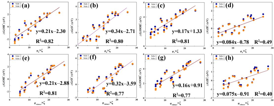
**Figure S7** Adsorption free energy of ORR and OER related species on transition metal-N<sub>4</sub> embedded b-PC monolayer; (a) to (d) relationship between  $\varphi_d \times \zeta$  with  $\Delta G(\text{OH}^*)$ ,  $\Delta G(\text{O}^*)$ ,  $\Delta G(\text{OOH}^*)$ , and  $\Delta G(\text{H}^*)$ ; (e) to (h) relationship between  $\varphi_{\text{valence}} \times \zeta$  with  $\Delta G(\text{OH}^*)$ ,  $\Delta G(\text{O}^*)$ ,  $\Delta G(\text{OOH}^*)$ , and  $\Delta G(\text{H}^*)$ .
