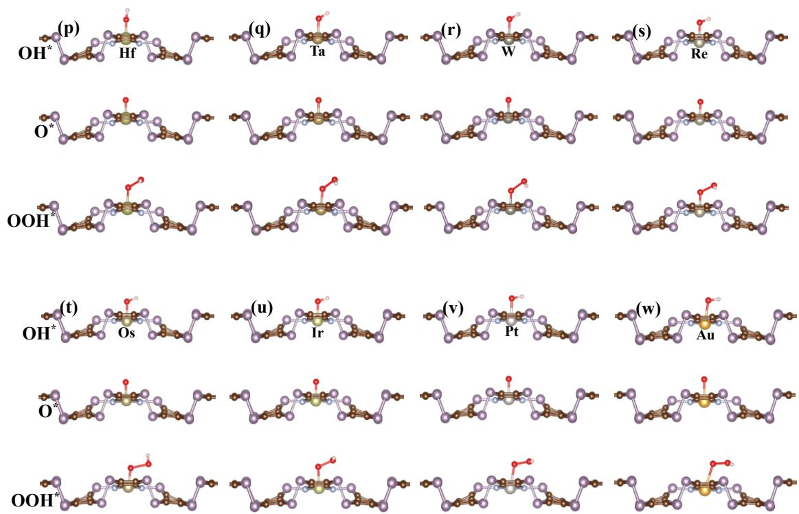
**Figure S4** Geometric structure of ORR/OER species ( $\text{OH}^*$ ,  $\text{O}^*$  and  $\text{OOH}^*$ ) adsorbed on transition metal- $\text{N}_4$  embedded b-PC monolayer (side 1).
