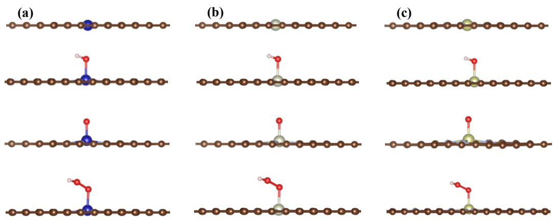
**Figure S10** Geometric structure of ORR/OER species ( $\text{OH}^*$ ,  $\text{O}^*$  and  $\text{OOH}^*$ ) adsorbed on (a) Co-N<sub>4</sub>/graphene, (b) Rh-N<sub>4</sub>/graphene, and (c) Ir-N<sub>4</sub>/graphene.
