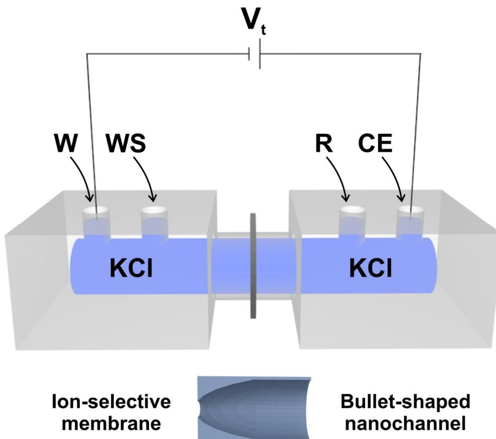
**Figure S4.** Scheme of experimental set-up used for the iontronic (not to scale) measurements consisting of two chambers separated by a PET membrane containing one single bullet-shaped nanochannel. The ionic flow of the KCl electrolyte through the nanochannel is monitored by a potentiostat with four-electrodes (working electrode W, working sense WS, reference R, counter-electrode CE).
