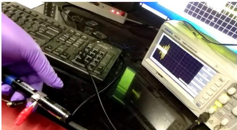
Figure S5: Photograph of output generation by touching a bent TENG.
