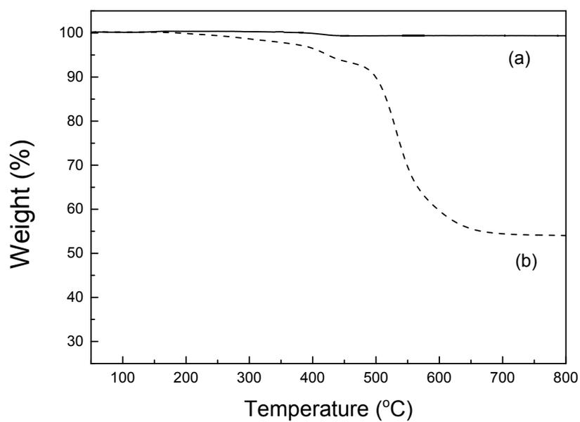
**Figure S6.** TGA curves of (a) AgNW aerogel and (b) AgNW/PDMS composite elastomer in nitrogen atmosphere. The heating rate was 10 °C/min.
