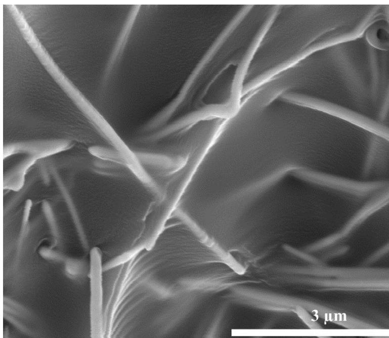
**Figure S7.** SEM image of AgNW/PDMS composite elastomer after 3 strain cycles.
