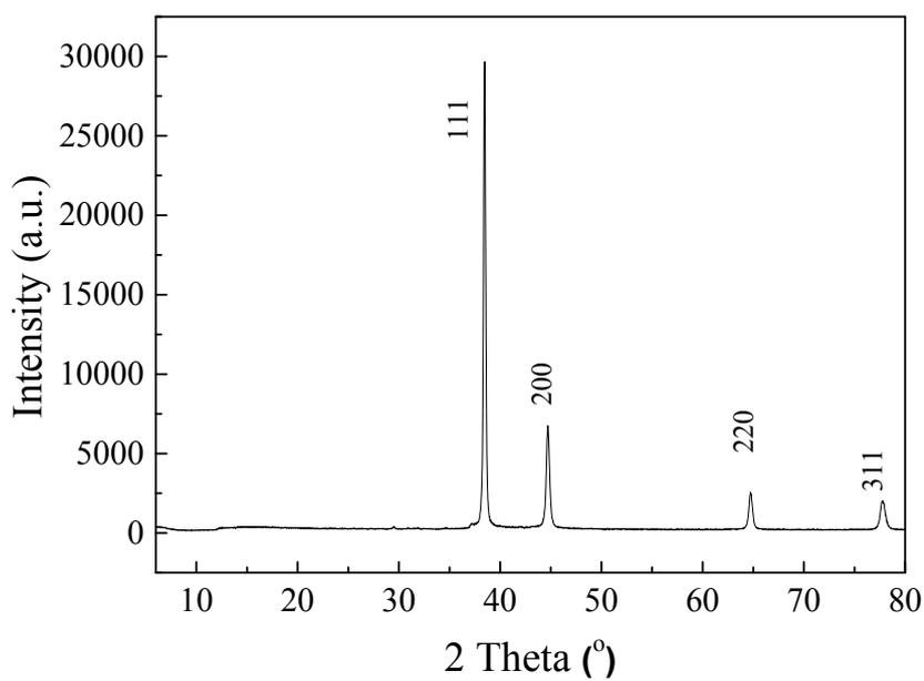
**Figure S5.** XRD pattern of the AgNW aerogels when exposed to air for 6 months.
