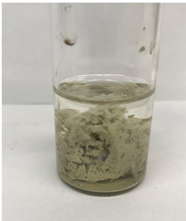
**Figure S3.** Photograph showing the synthesis of AgNW gel with initial  $\text{AgNO}_3$  concentration of 28.6 mg/mL at 160 °C. No robust gel was obtained.
