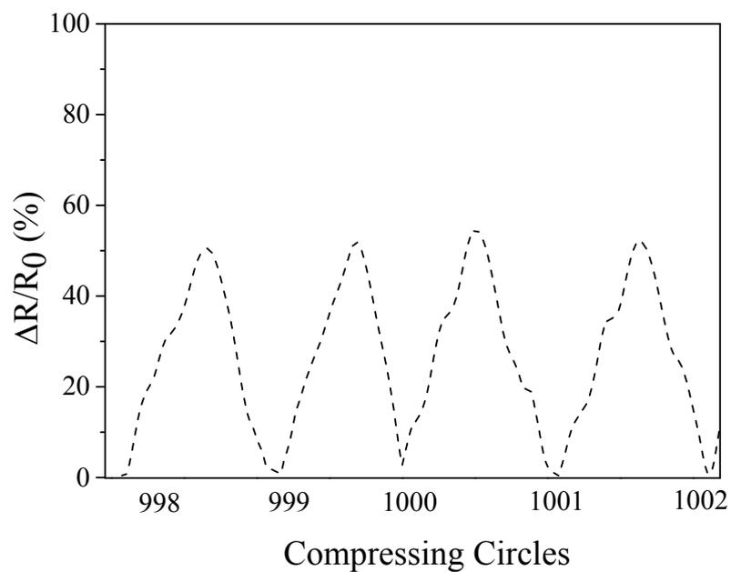
**Figure S8.** Electrical resistance change when repeatedly compressed at 1000 cycles.
