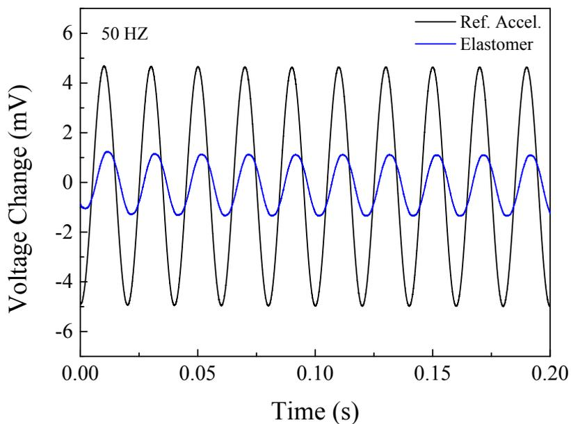
**Figure S9.** Dynamic piezoresistive response of AgNW/PDMS composites elastomer under a periodically sinusoidal excitation as a function of time. The loading frequency was 50 Hz. The blue curve represents AgNW/PDMS elastomer, and the black curve represents the commercial accelerometer.
