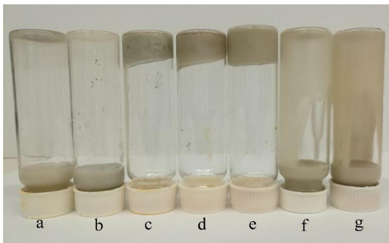
**Figure S2.** Photographs showing the synthesis of AgNW gels with different initial  $\text{AgNO}_3$  concentration. (a) 7.2 mg/mL, (b) 10.7 mg/mL, (c) 14.3 mg/mL, (d) 21.5 mg/mL, (e) 28.6 mg/mL, (f) 35.8 mg/mL, (g) 57.2 mg/mL. For all samples, the weight ratio of  $\text{AgNO}_3$  to PVP is fixed at 1.25.
