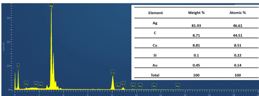
**Figure S4.** TEM/EDX spectrum analysis of AgNWs. The inset table in spectrum shows the elemental composition of an individual AgNW.
