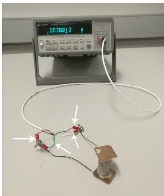
**Figure S1.** The electrical conductivities of AgNW aerogel and AgNW/PDMS aerogel were measured by a four-wire Kelvin method. To optimize the electrical contact, both ends of AgNW aerogel or aerogel composite were silver pasted to two pieces of flat copper foils. The four wires were then connected to the flat copper foils through two short wires. Then a high-sensitivity multimeter (Keysight 34420A. Nano Volt/Micro Ohm Meter) was used for resistance measurement.
