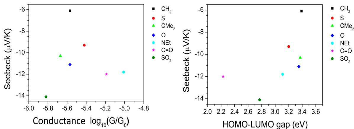
**Fig. S82** Correlation plot between measured conductance and measured Seebeck coefficient (left panel) and between theoretical HOMO-LUMO gap and measured Seebeck coefficient (right panel), for the *meta*-connected compounds 1-7 (1 ■ black square, 2 ● red circle, 3 ▲ light green triangle, 4 ◆ blue diamond, 5 ⬡ turquoise hexagon, 6 ★ magenta star, 7 ⬠ Olive green pentagon).
