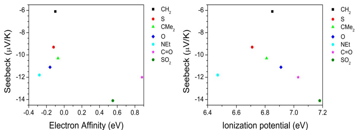
**Fig. S83** Correlation plot between theoretical electron affinity and measured Seebeck coefficient (left panel) and Correlation plot between theoretical ionization potential and measured Seebeck coefficient (right panel) for the *meta*-connected compounds 1-7 (1 ■ black square, 2 ● red circle, 3 ▲ light green triangle, 4 ◆ blue diamond, 5 ⬡ turquoise hexagon, 6 ★ magenta star, 7 ⬠ Olive green pentagon).
