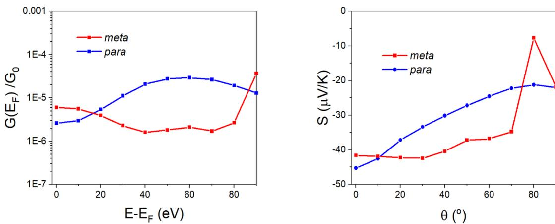
**Fig. S60** Conductance (left panel) and Seebeck coefficient (right panel) as a function of tilt angle  $\theta$  for  $X = \text{C=O}$  in a linear geometry.
