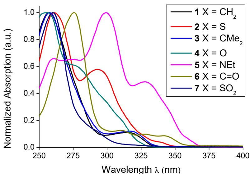
**Figure S78.** Normalized absorption spectra of **1-7** in dichloromethane.
