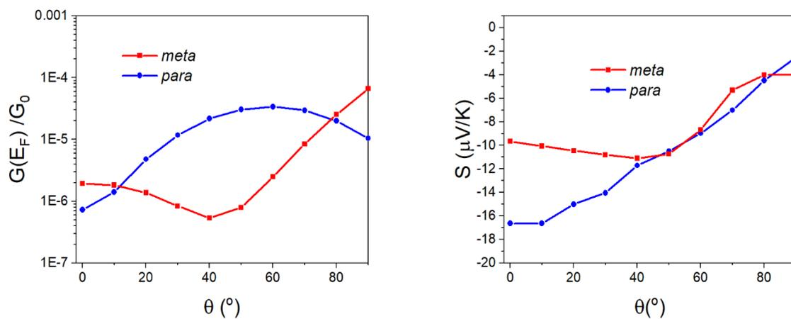
**Fig. S56** Conductance (left panel) and Seebeck coefficient (right panel) as a function of tilt angle  $\theta$  for  $\text{X} = \text{S}$  in a linear geometry.
