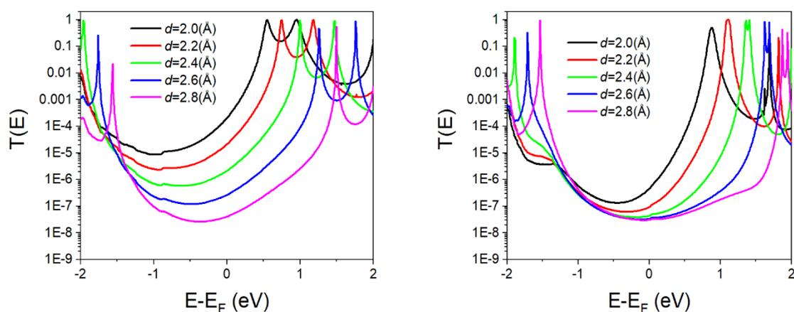
**Fig. S30** Transmission coefficient  $T(E)$  against electron energy of  $X = \text{CH}_2$  for varying contact separations  $d$  (Figure 7a and b) in the *para* connectivity (left panel) and *meta* connectivity (right panel).
