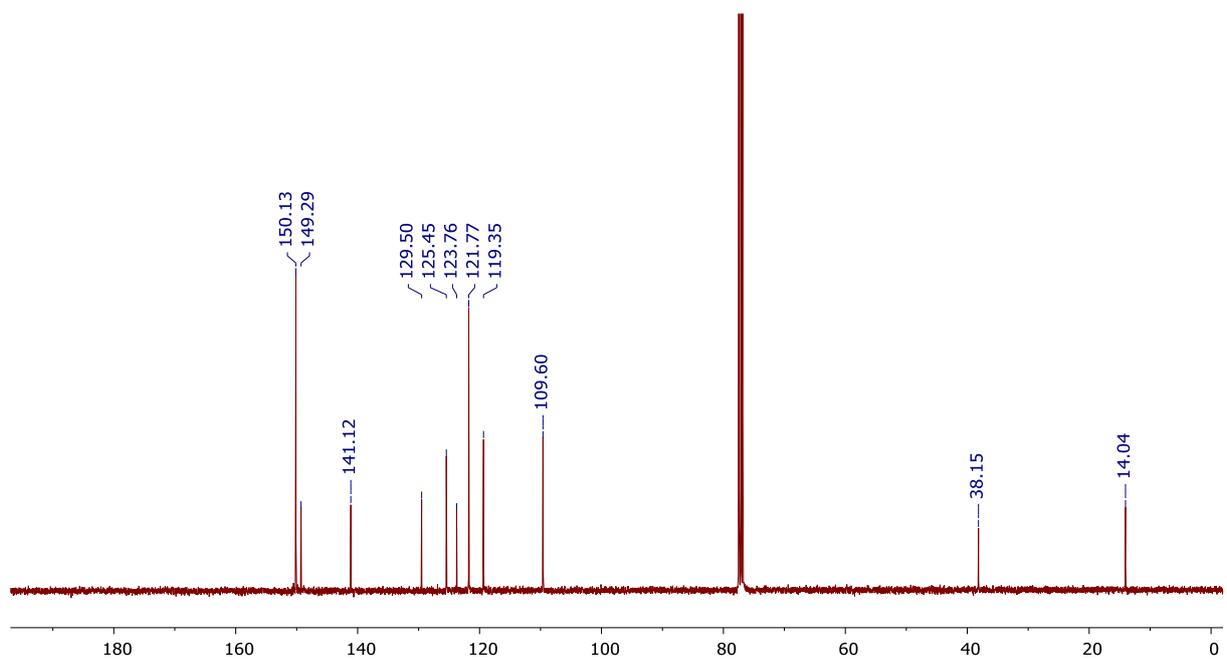
Figure S73 <sup>13</sup>C NMR Spectrum of 5 in CDCl<sub>3</sub> (δ 77.16 ppm)
