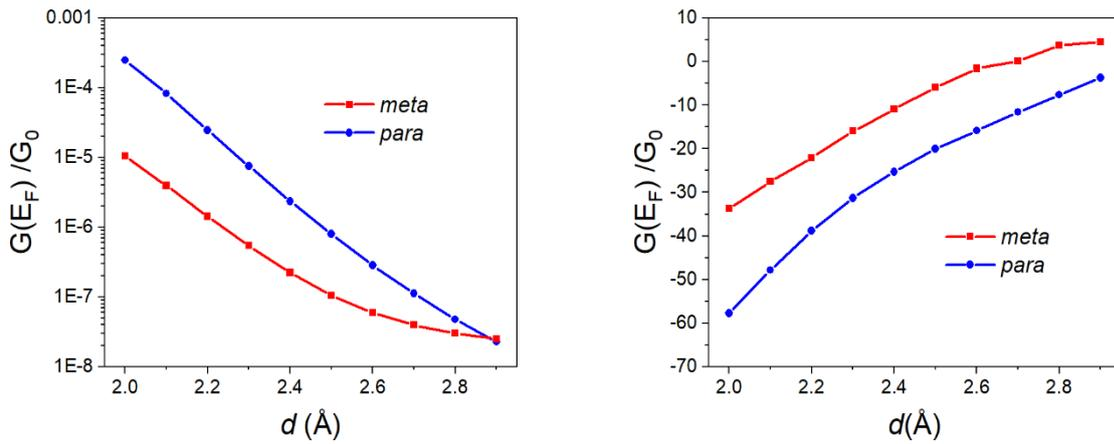
**Fig. S32** Molecule  $X = S$  (Left panel) Conductance vs contact distance  $d$ . (Right panel) Seebeck coefficient versus contact distance  $d$ .
