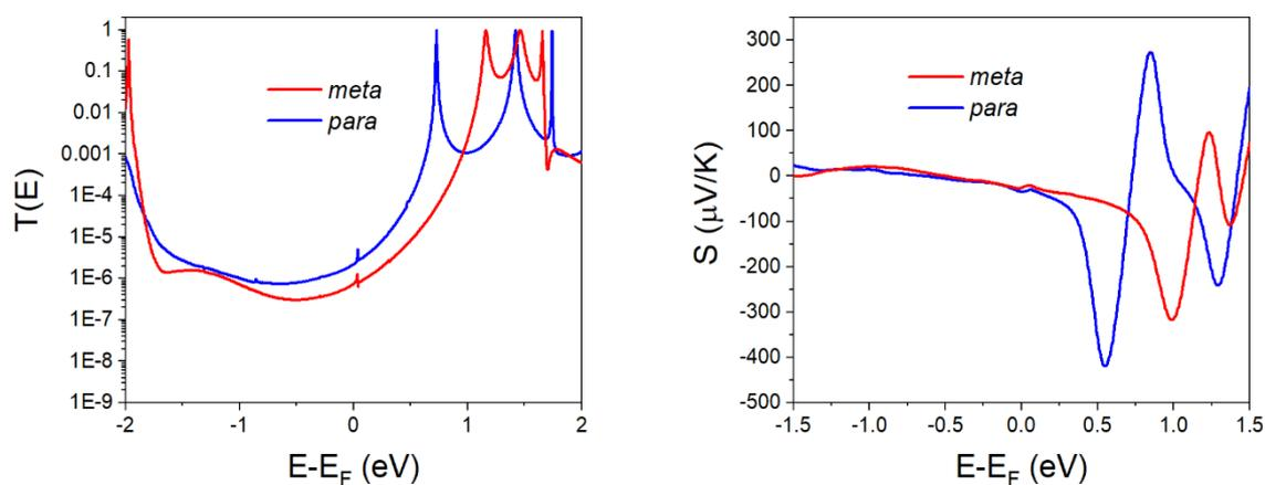
**Fig. S45** Linear contact geometry comparison between *para* and *meta* connectivity for  $X = \text{SO}_2$ . (left panel) Transmission coefficient (right panel) Seebeck coefficient.
