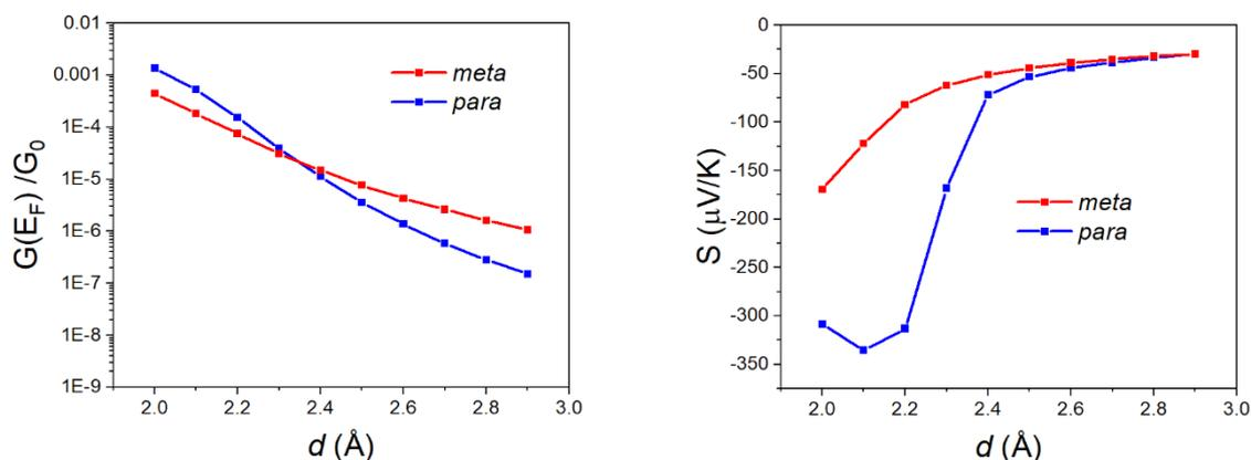
**Fig. S52**  $X = \text{C}=\text{O}$  in a linear geometry. (Left) Conductance vs contact distance  $d$ . (Right) Seebeck coefficient against contact distance  $d$ .
