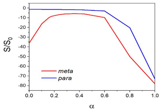
**Fig. S3** Room temperature Seebeck coefficient versus  $\alpha$  obtained from the transmission plots of Figure S1.
