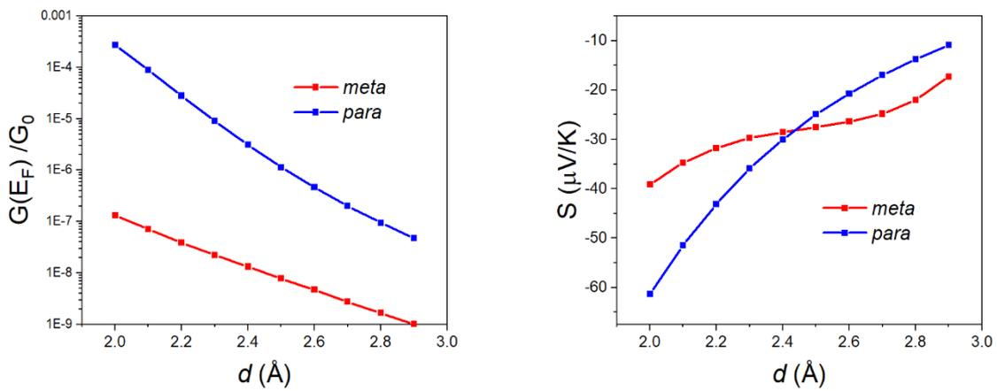
**Fig. S49** X = CMe<sub>2</sub> in a linear geometry. (Left) Conductance vs contact distance  $d$ . (Right) Seebeck coefficient against contact distance  $d$ .
