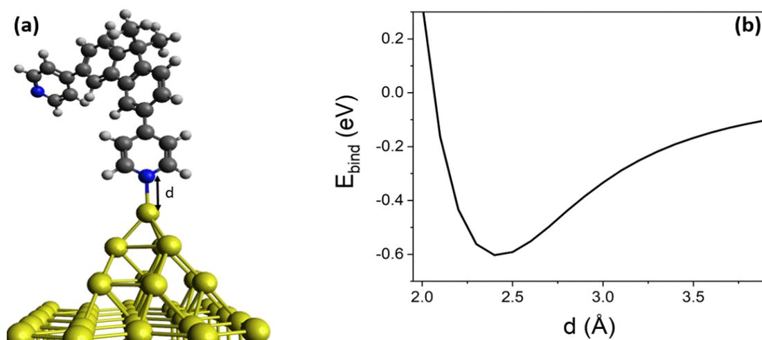
**Fig S19.** (a) Binding geometry as a function of the gold-nitrogen distance  $d$ . (b) Binding energy  $E_{\text{bind}}$  as a function of  $d$ .
