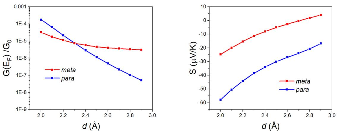
**Fig. S51** X = NEt in a linear geometry. (Left) Conductance vs contact distance  $d$ . (Right) Seebeck coefficient against contact distance  $d$ .
