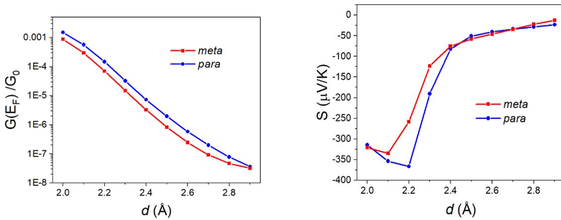
**Fig. S36** Molecule  $\mathbf{X} = \text{C=O}$  (Left panel) Conductance vs contact distance  $d$ . (Right panel) Seebeck coefficient versus contact distance  $d$ .
