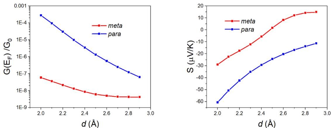
**Fig. S47**  $X = \text{CH}_2$  in a linear geometry. (Left) Conductance vs contact distance  $d$ . (Right) Seebeck coefficient against contact distance  $d$ .
