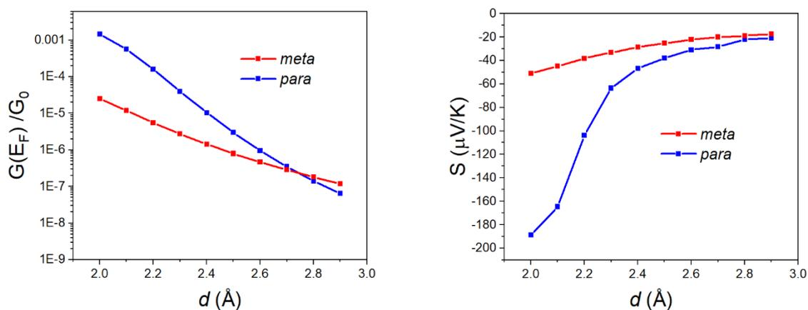
**Fig. S53**  $X=\text{SO}_2$  in a linear geometry. (Left panel) Conductance vs contact distance  $d$ . (Right panel) Seebeck coefficient against contact distance  $d$ .
