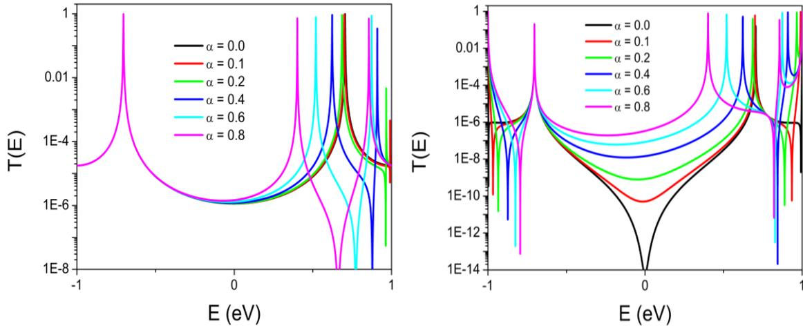
**Fig. S1** Transmission coefficients versus electron energy for the tight binding model of Figure 3a. Left panel: *para* connectivity. Right panel: *meta* connectivity ( $\Gamma=0.08y$ ).
