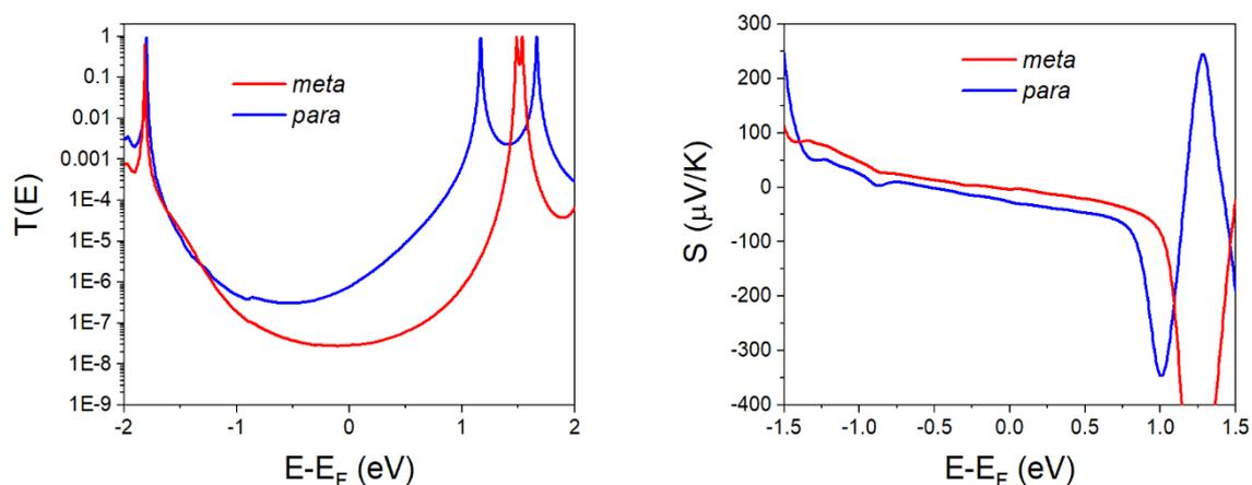
**Fig. S23** Comparison between *para* and *meta* connectivity for  $\mathbf{X} = \text{CH}_2$ . Transmission coefficient (left panel) Seebeck coefficient (right panel).
