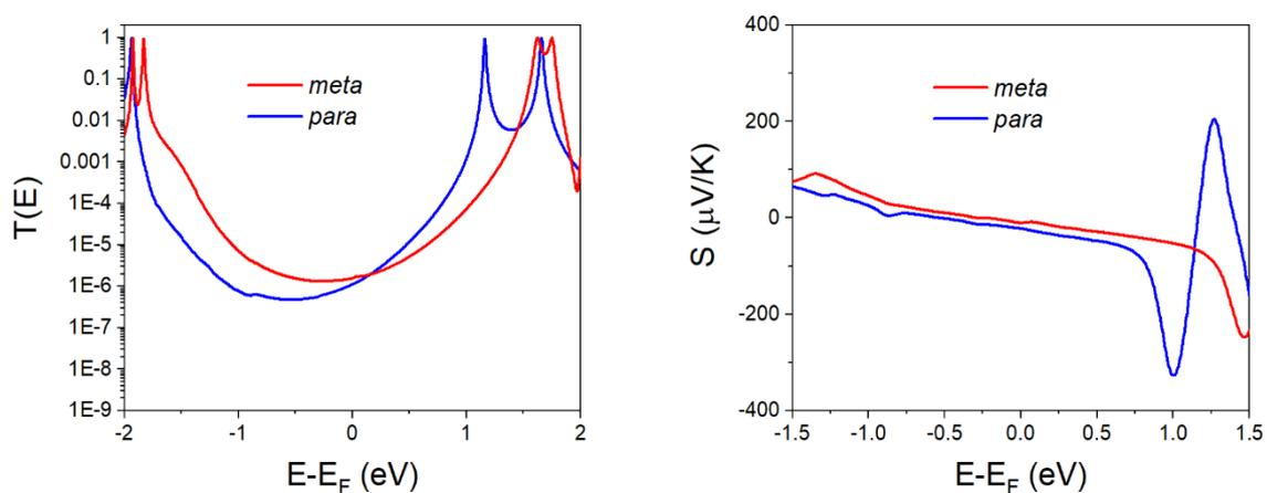
**Fig. S42** Linear contact geometry comparison between *para* and *meta* connectivity for  $\mathbf{X} = \text{O}$ . (left panel) Transmission coefficient (right panel) Seebeck coefficient.
