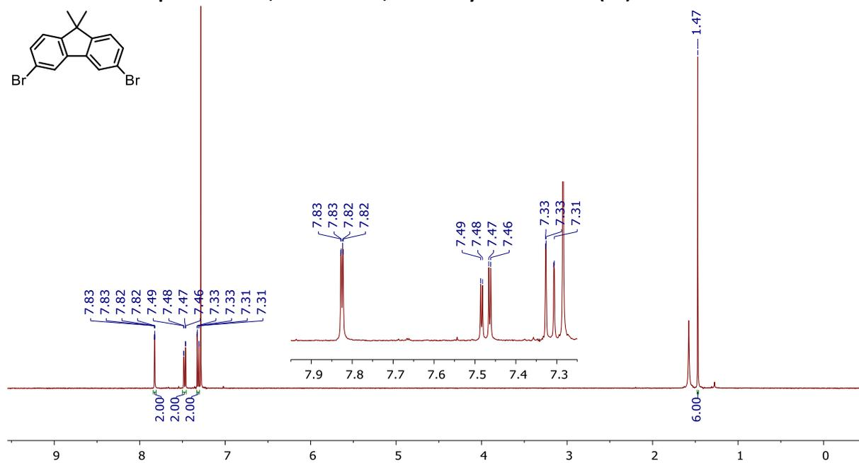
Fig. S63 <sup>1</sup>H NMR Spectrum of 3a in CDCl<sub>3</sub> (δ 7.26 ppm)
