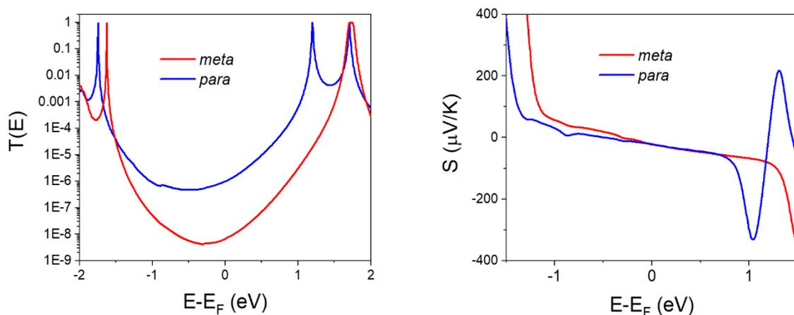
**Fig. S41** Linear contact geometry comparison between *para* and *meta* connectivity for  $\mathbf{X} = \text{CMe}_2$ . (left panel) Transmission coefficient (right panel) Seebeck coefficient.
