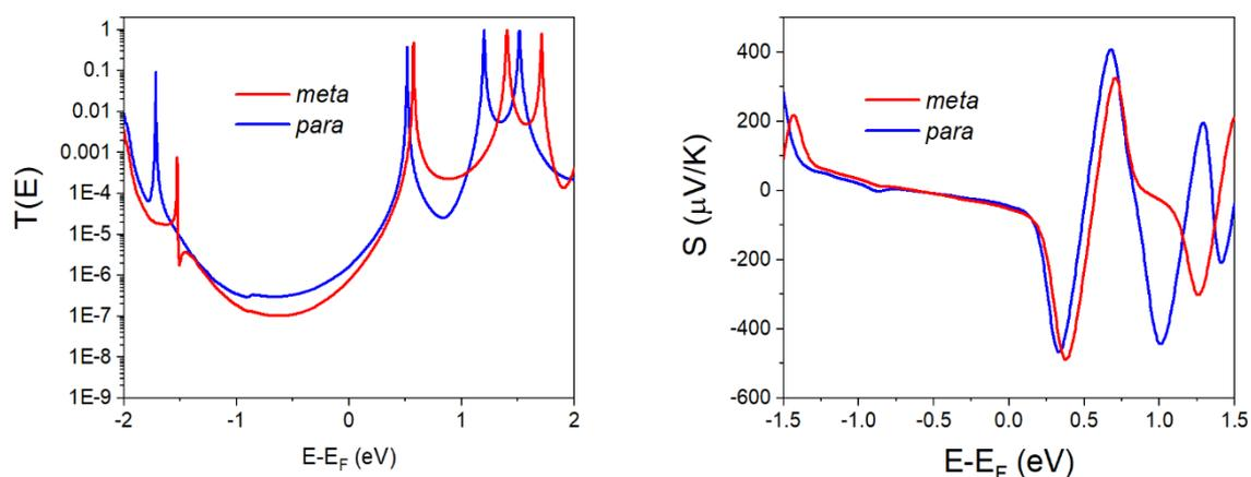
**Fig. S28** Comparison between *para* and *meta* connectivity for  $\mathbf{X} = \text{C}=\text{O}$ . Transmission coefficient (left panel) Seebeck coefficient (right panel).
