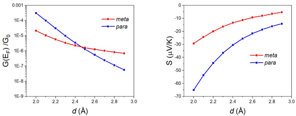
**Fig. S50** X = O in a linear geometry. (Left) Conductance vs contact distance  $d$ . (Right) Seebeck coefficient against contact distance  $d$ .
