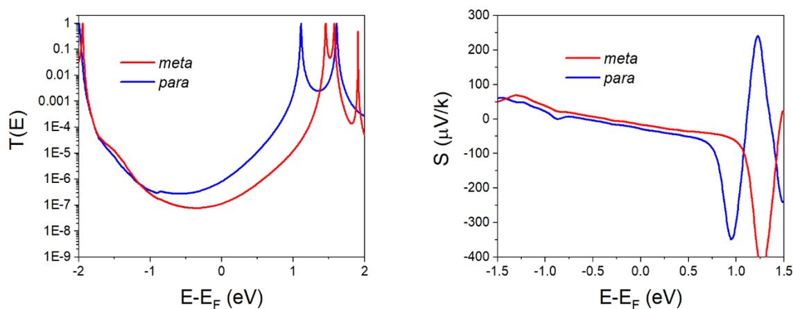
**Fig. S26** Comparison between *para* and *meta* connectivity for  $\mathbf{X} = \text{O}$ . Transmission coefficient (left panel) Seebeck coefficient (right panel).
