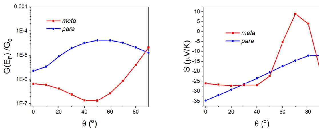
**Fig. S61** Conductance (left panel) and Seebeck coefficient (right panel) as a function of tilt angle  $\theta$  for  $\mathbf{X} = \text{SO}_2$  in a linear geometry.
