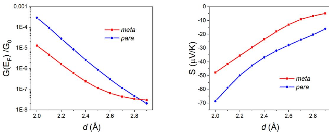
**Fig. S34** Molecule  $X = O$  (Left panel) Conductance vs contact distance  $d$ . (Right panel) Seebeck coefficient versus contact distance  $d$ .
