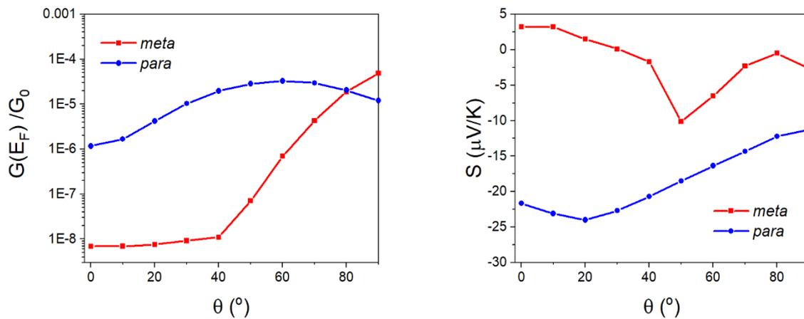
**Fig. S55** Conductance (left panel) and Seebeck coefficient (right panel) as a function of tilt angle  $\theta$  for  $\text{X} = \text{CH}_2$  in a linear geometry.
