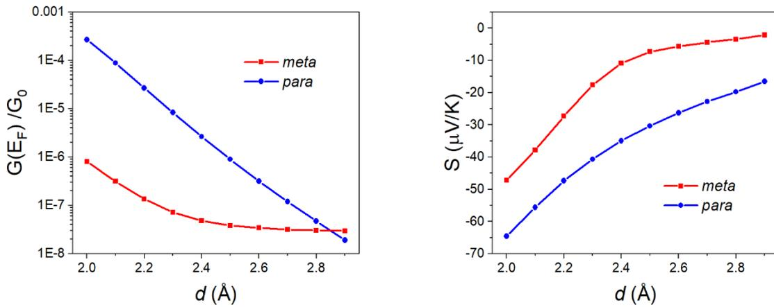
**Fig. S33** Molecule  $X = \text{CMe}_2$  (Left panel) Conductance vs contact distance  $d$ . (Right panel) Seebeck coefficient versus contact distance  $d$ .
