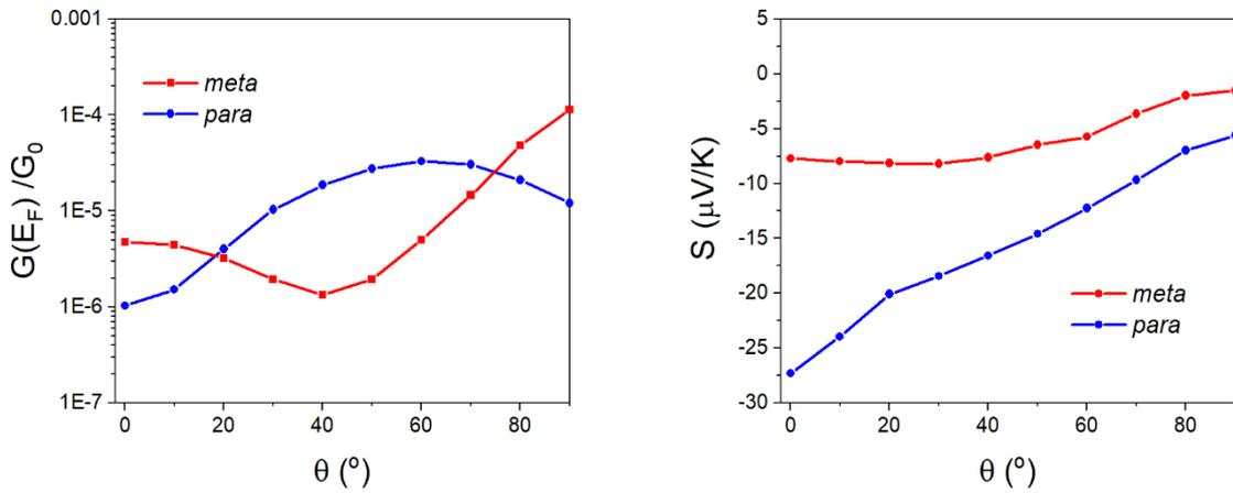
**Fig. S59** Conductance (left panel) and Seebeck coefficient (right panel) as a function of tilt angle  $\theta$  for  $X = \text{NEt}$  in a linear geometry.
