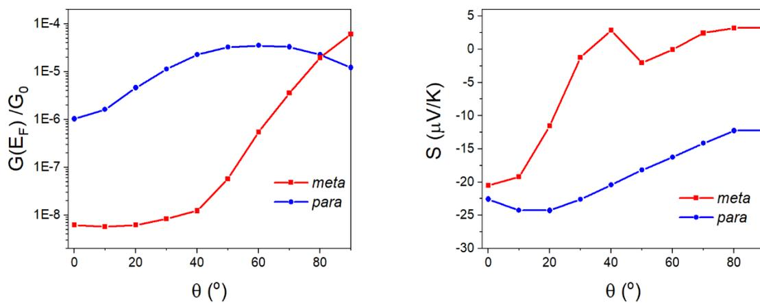
**Fig. S57** Conductance (left panel) and Seebeck coefficient (right panel) as a function of tilt angle  $\theta$  for  $\text{X} = \text{CMe}_2$  in a linear geometry.
