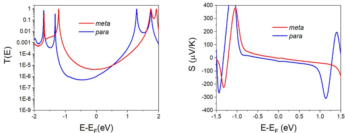
**Fig. S43** Linear contact geometry comparison between *para* and *meta* connectivity for  $X = \text{NEt}$ . (left panel) Transmission coefficient (right panel) Seebeck coefficient.
