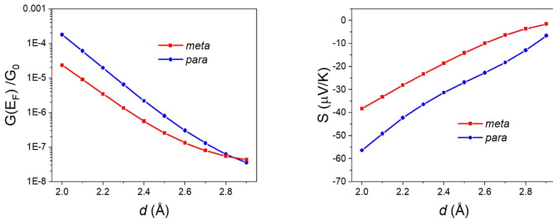
**Fig. S35** Molecule  $\mathbf{X} = \text{NEt}$  (Left panel) Conductance vs contact distance  $d$ . (Right panel) Seebeck coefficient versus contact distance  $d$ .
