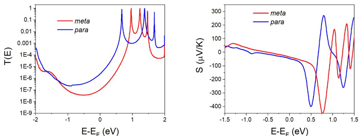
**Fig. S29** Comparison between *para* and *meta* connectivity for  $\mathbf{X} = \text{SO}_2$ . Transmission coefficient (left panel) Seebeck coefficient (right panel).
