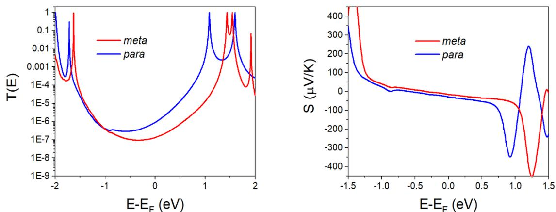
**Fig. S24** Comparison between *para* and *meta* connectivity for  $\mathbf{X} = \text{S}$ . Transmission coefficient (left panel) Seebeck coefficient (right panel).
