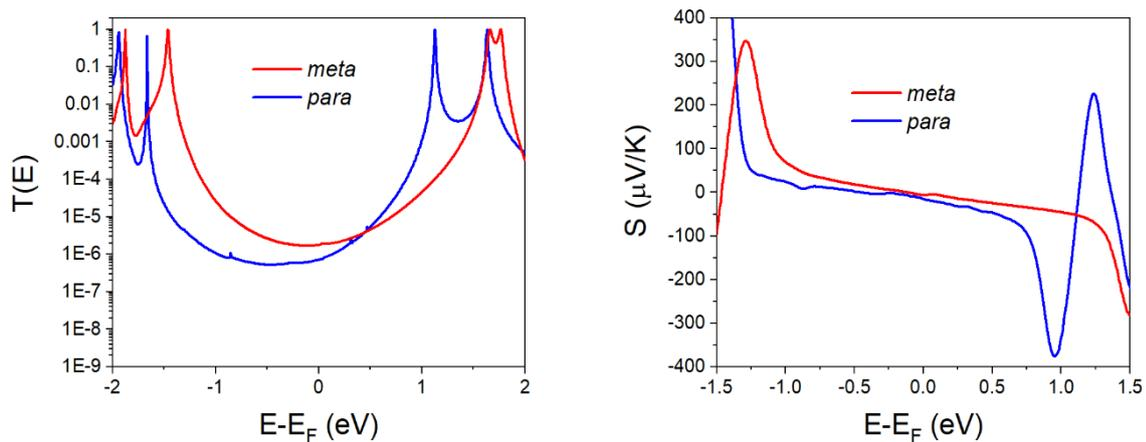
**Fig. S40** Linear contact geometry comparison between *para* and *meta* connectivity for  $\mathbf{X} = \text{S}$ . (left panel) Transmission coefficient (right panel) Seebeck coefficient.
