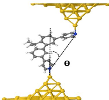
**Fig. S54** Geometry of the molecule junction for varying the contact angle  $\theta$  for a fixed contact distance  $d=2.5\text{\AA}$ .
