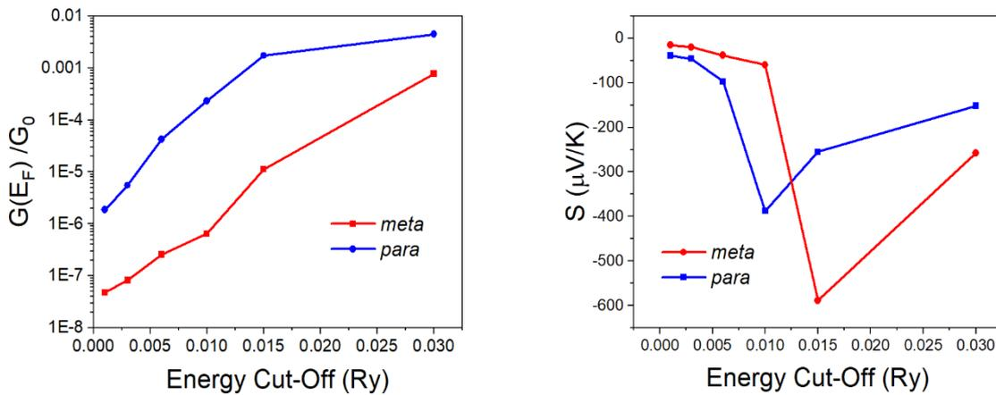
**Fig. S21** Conductance (left panel) and Seebeck coefficient (right panel) evaluated at  $E_F$  as a function of the basis set cut-off.
