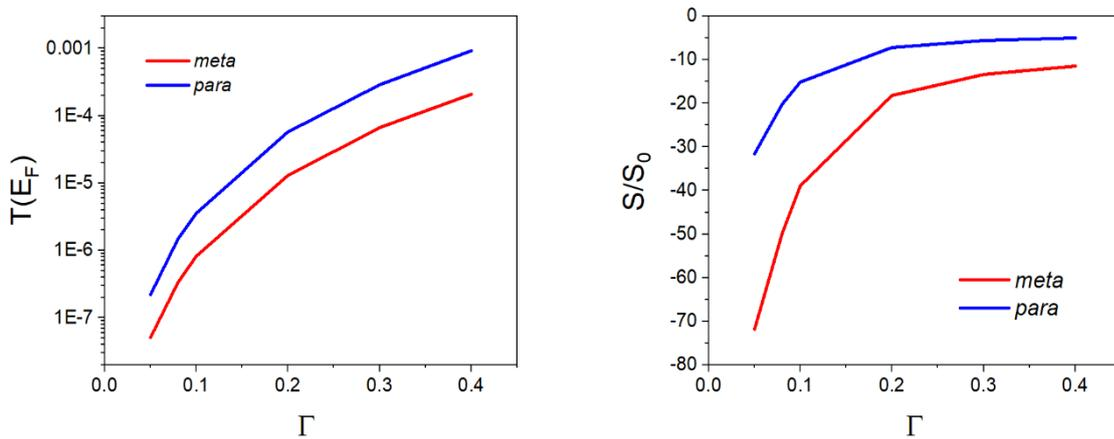
**Fig. S2** Left Panel: Plots of  $T(E_F)$  versus the coupling strength  $\Gamma$  to the leads. Right Panel: Plots of  $S/S_0$  versus the coupling strength  $\Gamma$  to the leads. ( $\alpha=0.8$ )
