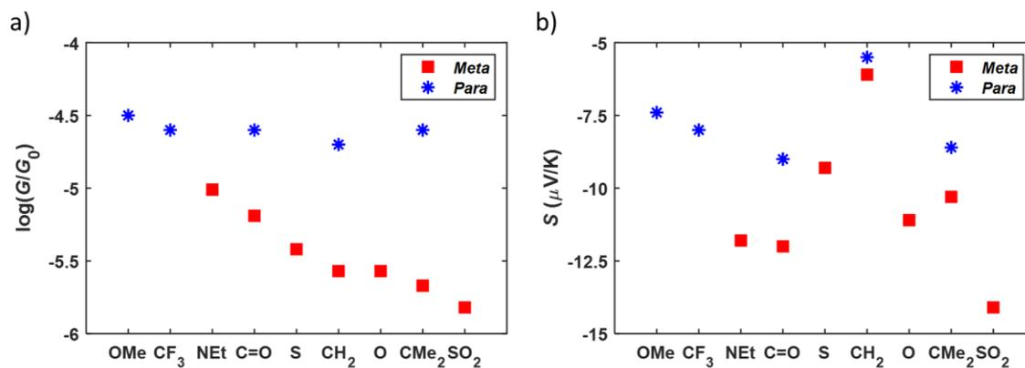
**Figure S80:** Measured conductance (a) and Seebeck coefficient (b) for the *meta*-connected compounds **1-7** (red squares), ordered by decreasing conductance, and comparison with the values of the *para*-connected systems (blue stars)<sup>6</sup>.
