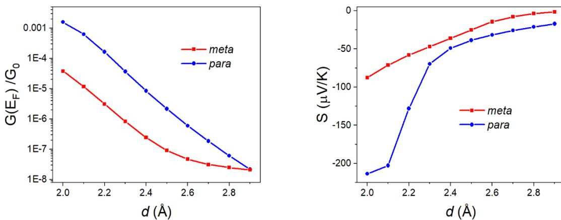
**Fig. S37** Molecule  $\mathbf{X} = \text{SO}_2$  (Left panel) Conductance vs contact distance  $d$ . (Right panel) Seebeck coefficient versus contact distance  $d$ .
