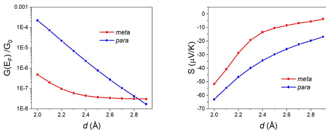
**Fig. S31.** Molecule  $X = \text{CH}_2$  (Left panel) Conductance vs contact distance  $d$ . (Right panel) Seebeck coefficient versus contact distance  $d$ .
