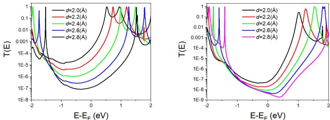
**Fig. S46** Transmission coefficient  $T(E)$  for varying contact distance  $d$  in the linear geometry. (Left)  $X = \text{CH}_2$  *para*. (Right)  $X = \text{CH}_2$  *meta*.
