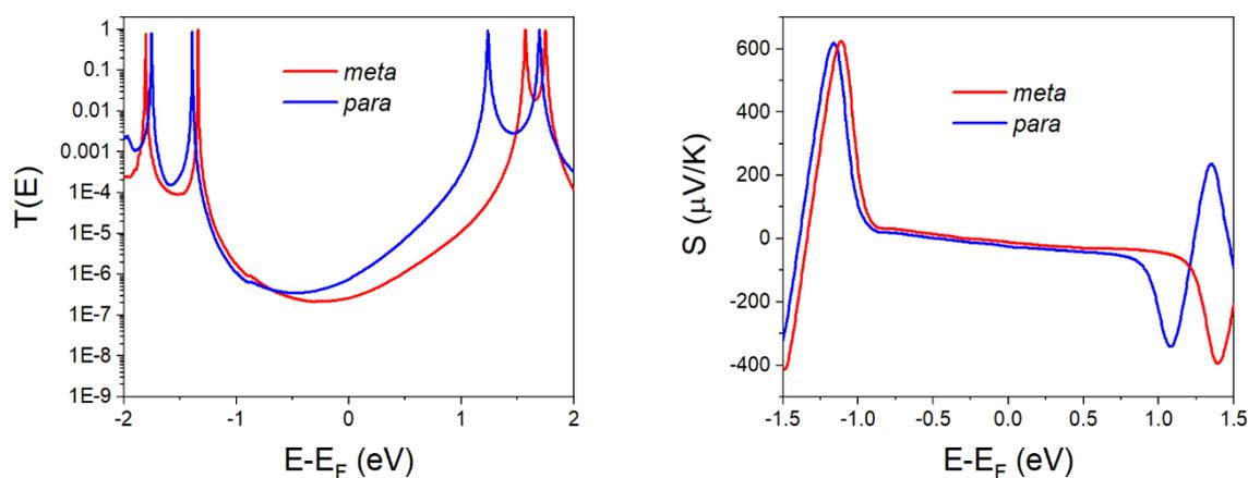
**Fig. S27** Comparison between *para* and *meta* connectivity for  $\mathbf{X} = \text{NEt}$ . Transmission coefficient (left panel) Seebeck coefficient (right panel).
