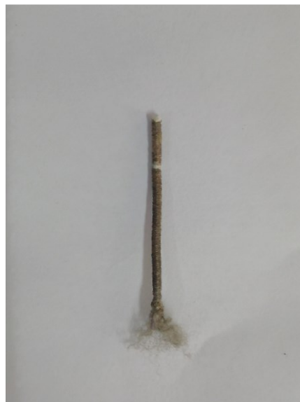
Fig. S5. (a,b) Optical photos of a pristine PET yarn(left) and AgNWs coated PET yarn(right).
