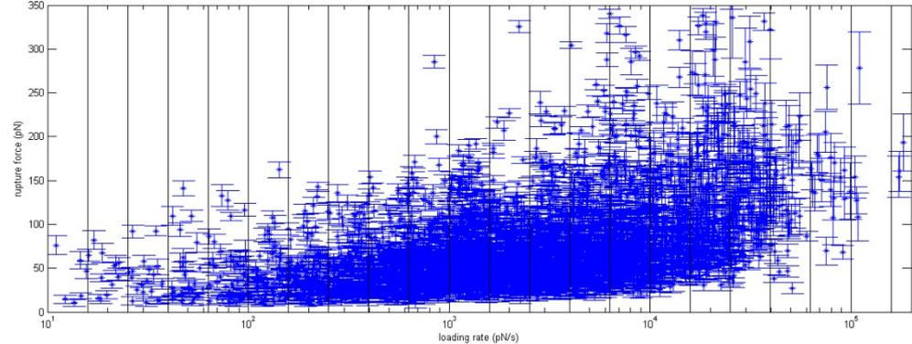
*Figure 4: Plot of individual rupture forces versus force loading rate of force spectroscopy experiments on ultraflat erythrocyte ghosts, using an ESD-1 functionalized tip.*
