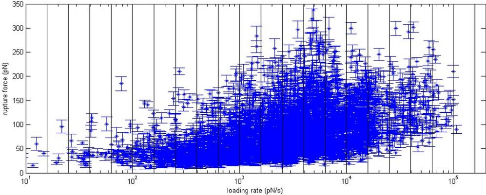
*Figure 3: Plot of individual rupture forces versus force loading rate of force spectroscopy experiments on ultraflat erythrocyte ghosts, using a BRAD5 functionalized tip.*
